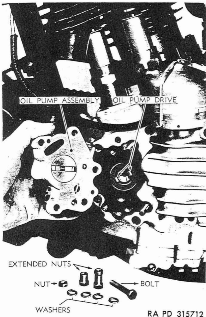
Figure 17—Oil Pump Removed
