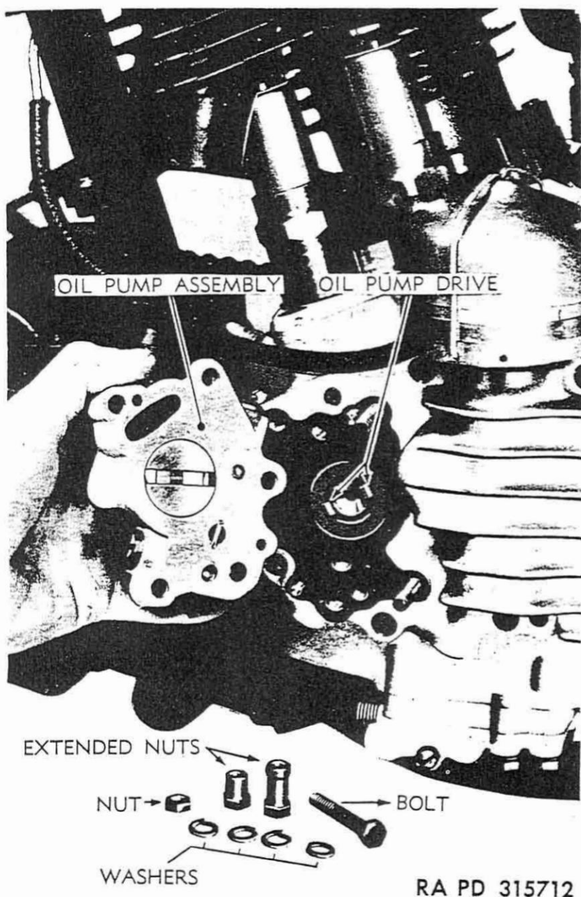
Figure 17—Oil Pump Removed
