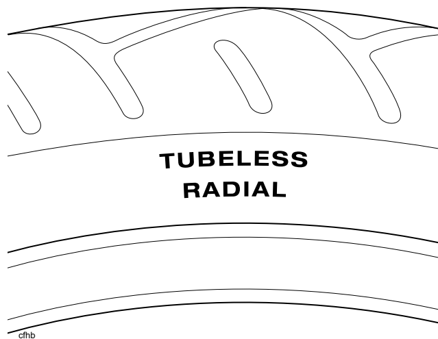
Typical Tyre Marking -Tubeless Tyre
