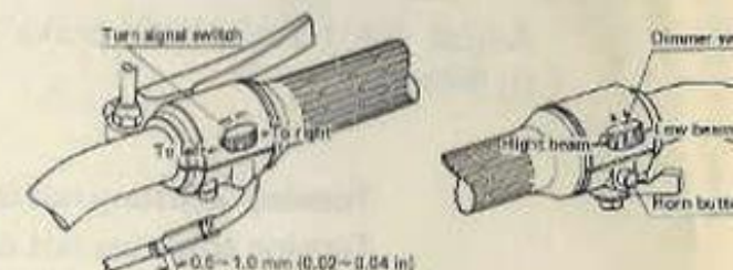
Fig. 15 Checking electrical equipment
