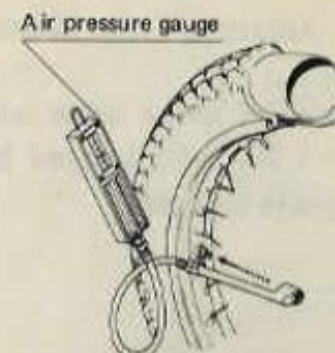
Fig. 14 Checking tire pressure
