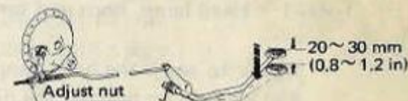
Fig. 12 Brake pedal play
