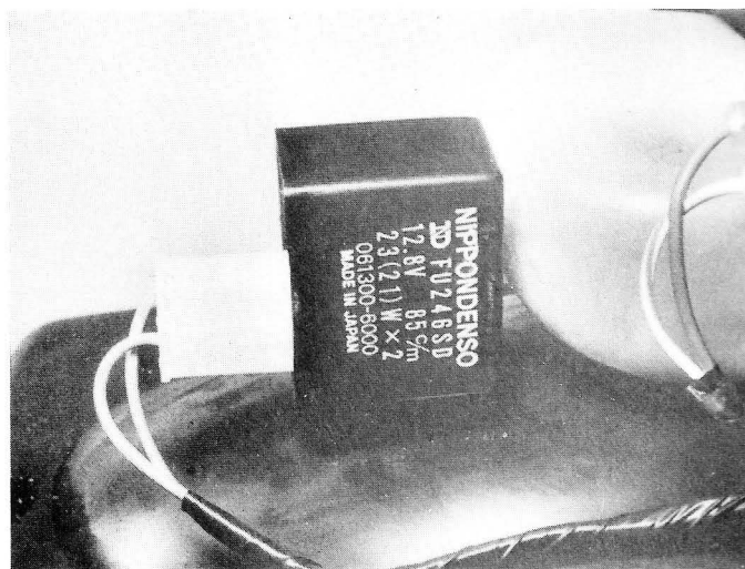
17.3 The turn signal relay. Note information on voltage, flash rate and specified bulb wattages
