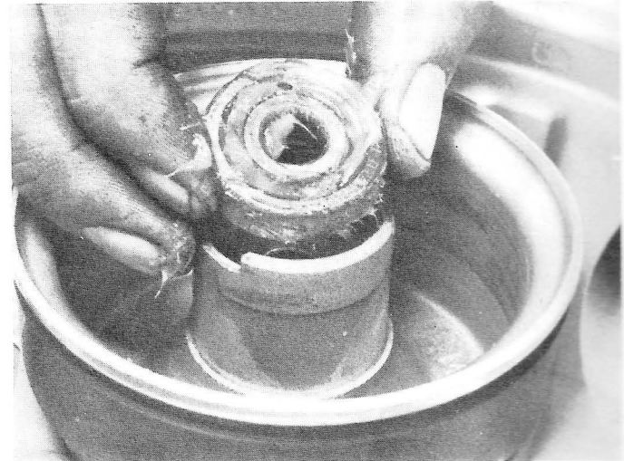
5.4a Pack bearings with high melting point grease ...
