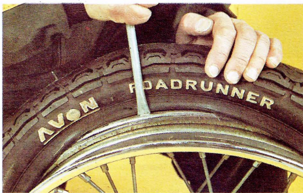
When first bead is clear, remove tyre as shown
