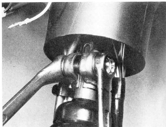
4.3 Remove clamp bolt and lift handlebar assembly clear of steering column splines
