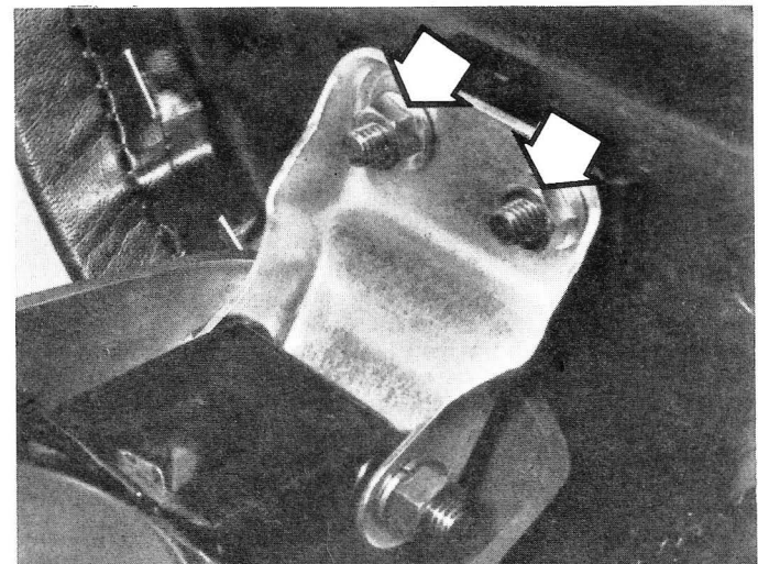
2.5a Remove nuts (arrowed) and lift seat away
