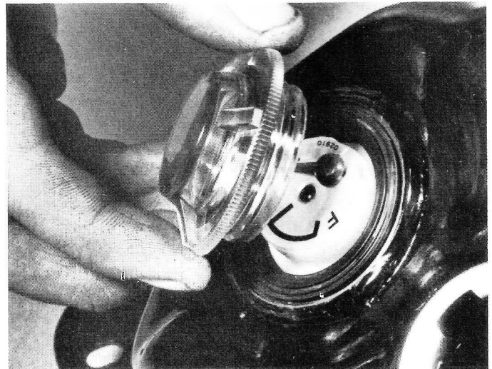
4.3a Unscrew the plastic lens, taking care not to damage it
