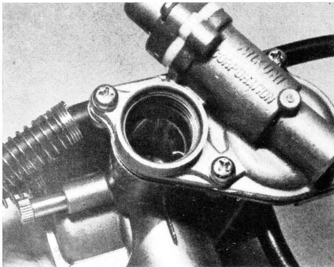
7.6a Automatic choke assembly is mounted on top of carburettor
