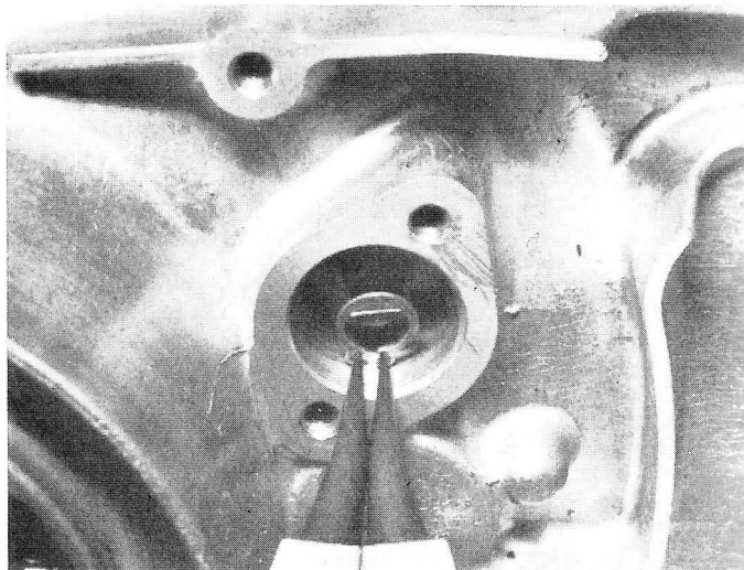
26.3b ... and secure with circlip
