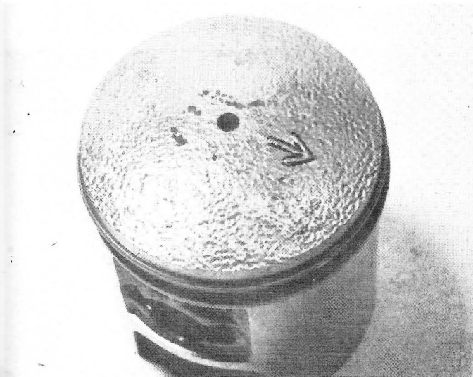
29.2b Arrow on piston crown must face exhaust port (rear of engine unit)
