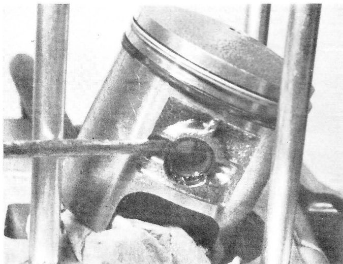
7.4a Prise out circlip using small screwdriver. Note rag packing in crankcase mouth
