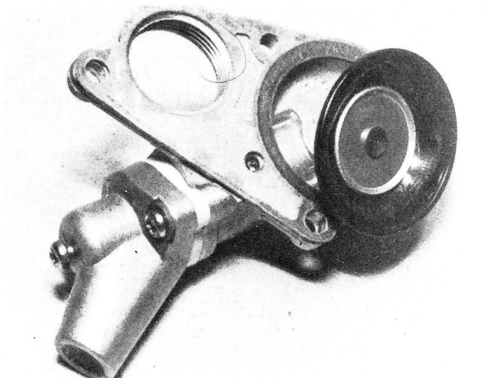
7.7a Carefully peel diaphragm off carburettor top
