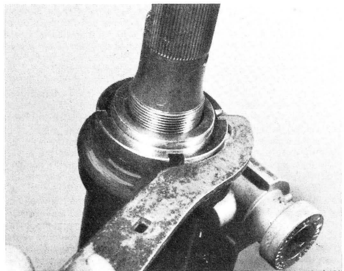
4.11 c Adjust the steering head bearings ...
