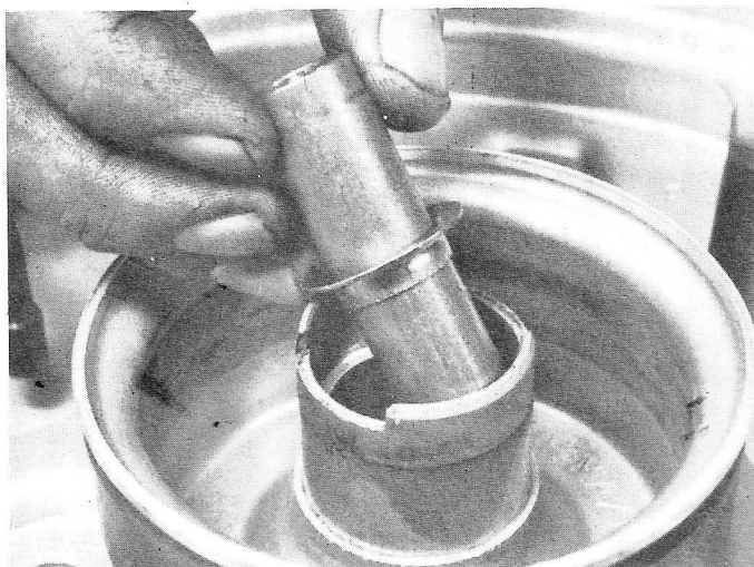
5.3 Bearings are separated by a spacer
