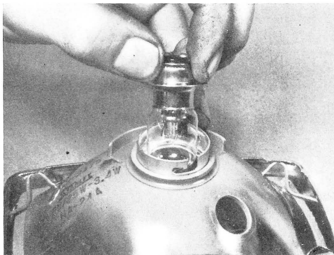
19.1c ... and lift the bulb out of the reflector
