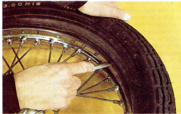
Work first bead over rim, using lever in final section
