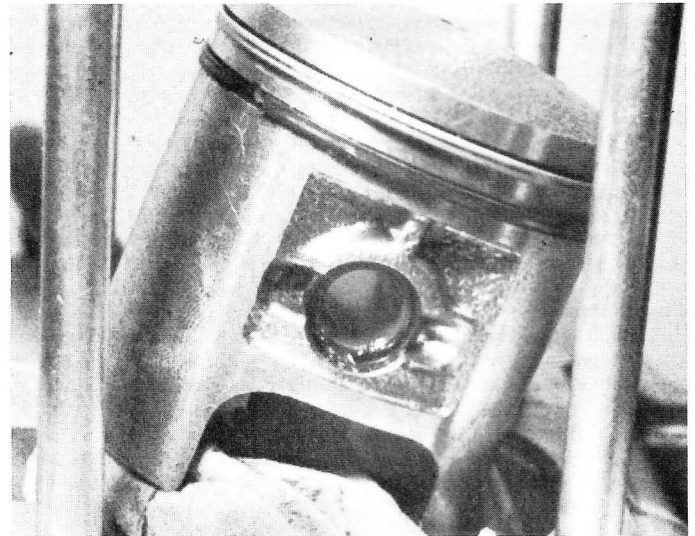
29.3 Secure gudgeon pin using new circlips
