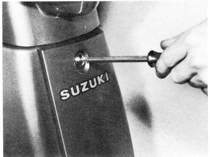
2.3a Centre section is retained by large cross-head screw
