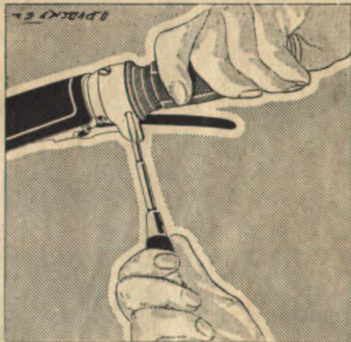
Fig. 47 - Adjusting the twist grip
