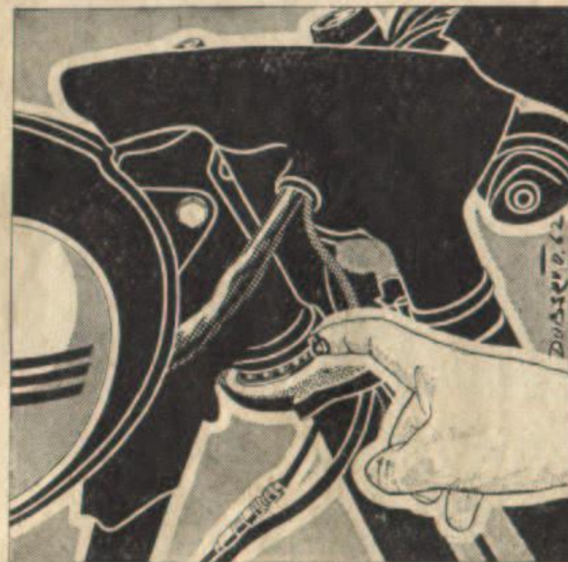
Fig. 46 - Lubricating the steering head ball bearing
