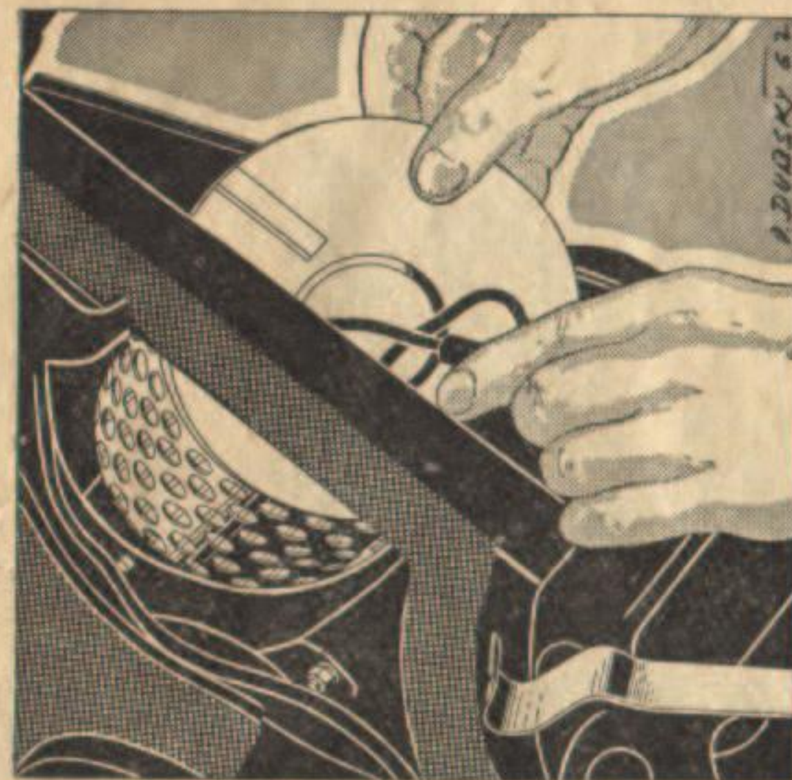
Fig. 26b - Removing the induction silencer top (250 c. c.)
