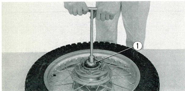
Fig. 2-13 ① Retainer wrench (07088-32901)
