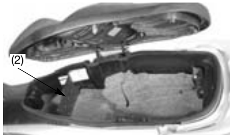
(1) Center compartment (2) Partition board
