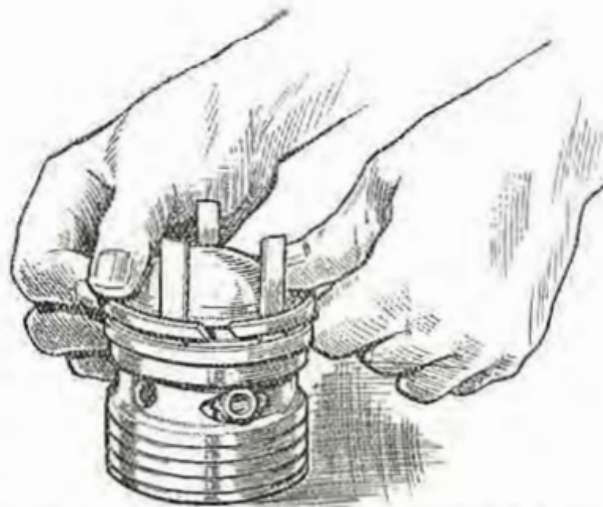
Three thin strips of tin fitted in a manner as illustrated, facilitates piston ring removal. Slip these behind the rings over the ring gap, one at a time, and then equally space, when the rings are readily removable.
