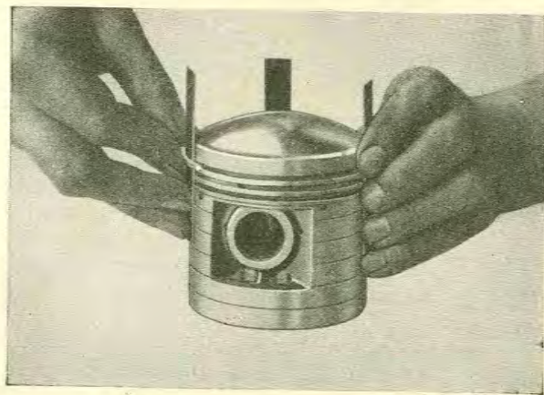
Removal or fitting of Piston Rings.
