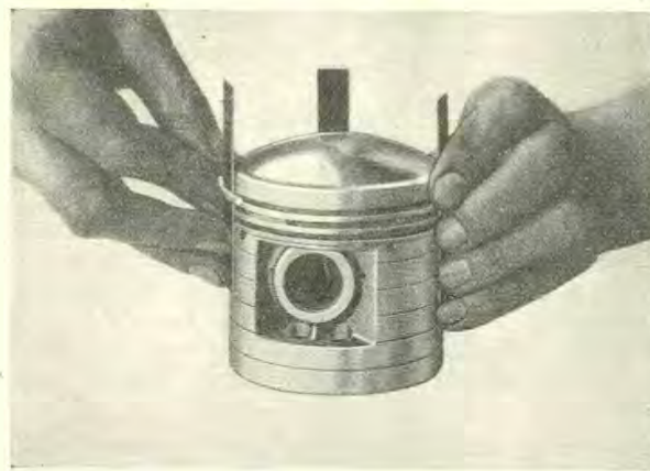
Removal or fitting of Piston Rings.
