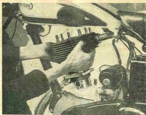
Removal of Cylinder Barrel.
