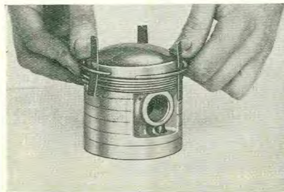
Removal or fitting of Piston Rings.
