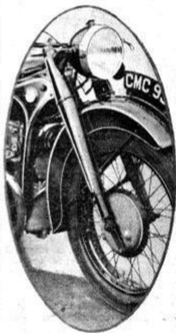
(Right) Telescopic, oval section, forks and a streamlined rubber mounting for the head lamp are features of the B.M.W.
