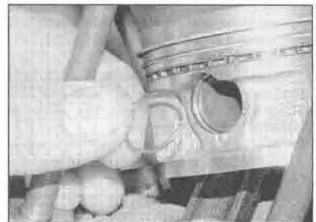
16.17b ... and secure it with the circlip, locating the open end away from the notch in the piston
