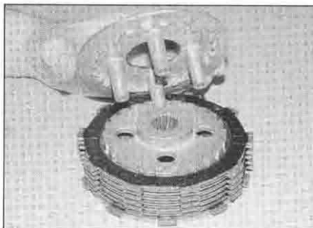
18.30e Fit the pressure plate into the centre, making sure it locates correctly
