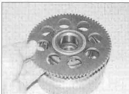
22.4a Withdraw the gear . . .
