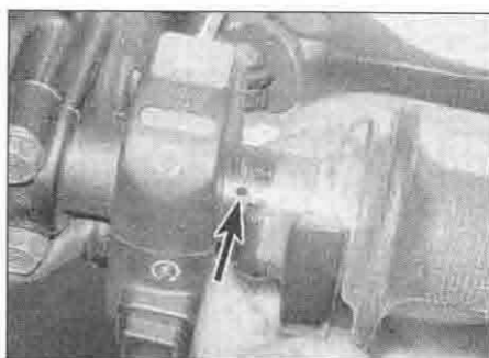
11.8b ... aligning the mating surfaces with the punch mark (arrowed)
