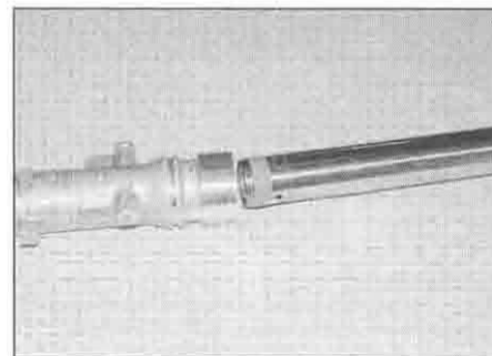
8.20a Slide the tube into the slider
