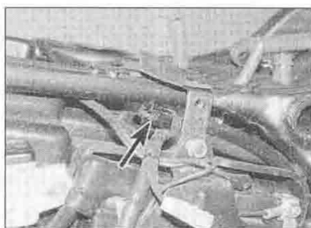
25.2b Diode (arrowed) – XL650V
