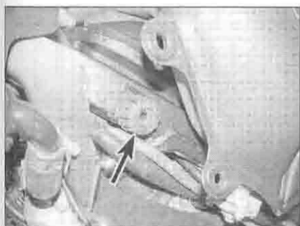
2.21 Take care not to dislodge the rubbers (arrow) as you locate the tank
