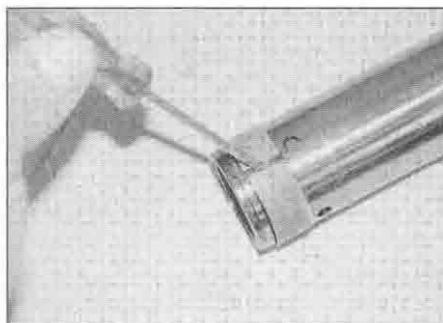
8.17b Carefully lever the ends apart and slide the bush off
