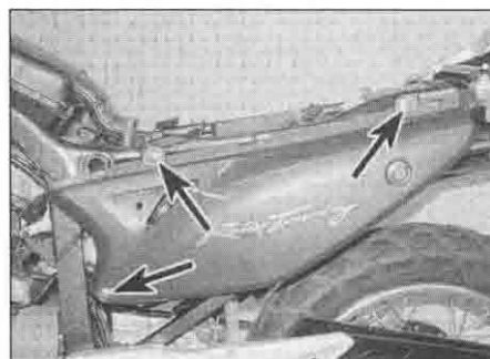
5.14a Undo the screws (arrowed) ...
