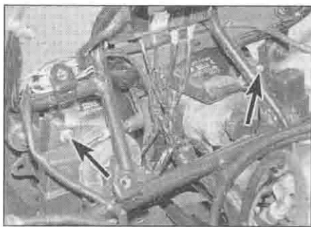
20.8b Horizontal adjustment screws (arrowed)
