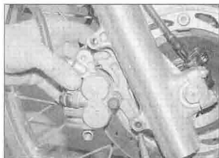
4.19 Slide the caliper onto the disc and install the bolts
