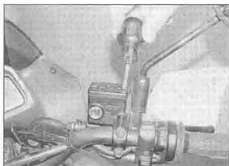
7.4 Slacken the reservoir cover screws
