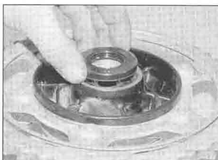
15.32a Press or drive the seal into the coupling
