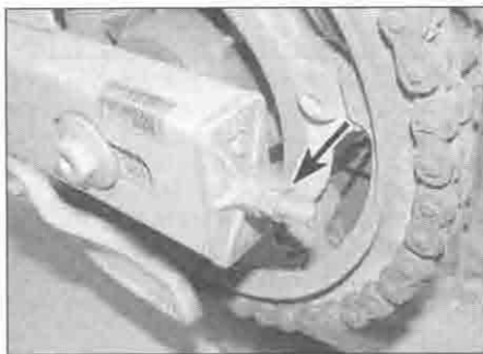
1.10a Slacken the locknut (arrowed) . . .
