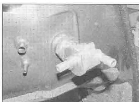
2.24c Fuel tap – XRV750-P models onwards
