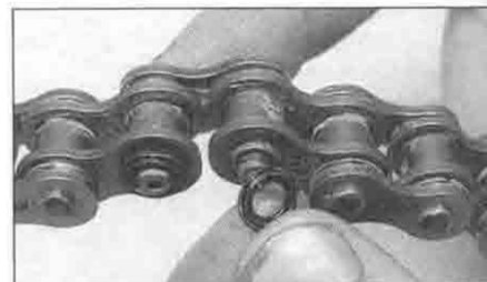
8.5 ... install the O-rings over the pin ends ...
