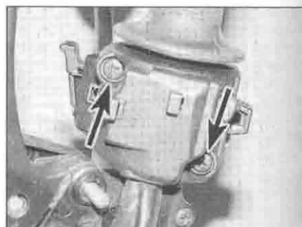
5.4b . . . and left-hand switch screws (arrowed)
