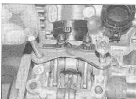
9.28b Fit the oil guide plate with the bolts
