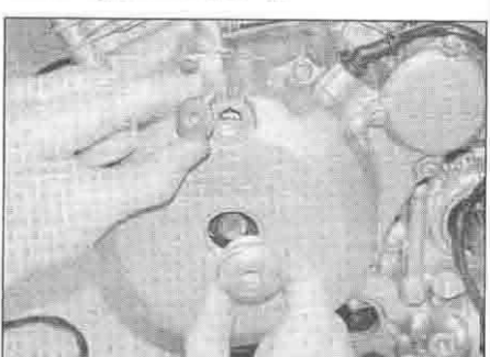
9.35 Smear the cap threads with grease and fit new O-rings if necessary
