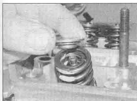
14.28c ... then fit the spring retainer
