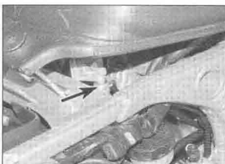
2.18a Detach the fuel hose (arrowed) ...
