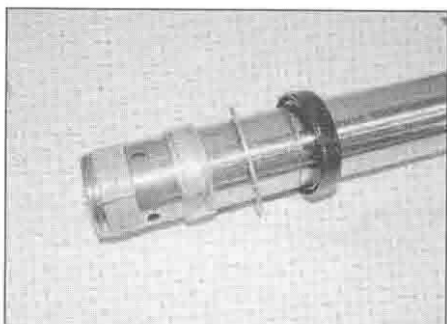
8.11b ... the slide-hammer effect will displace the oil seal and bush
