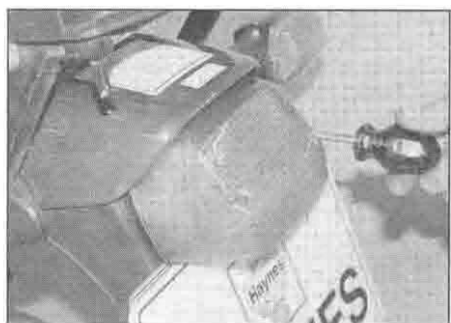
9.1a Undo the screws ...
