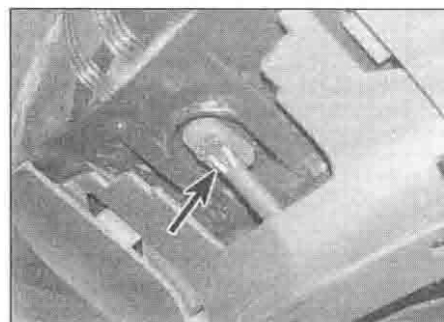
7.8a Sidelight bulbholder (arrowed) - XL650V
