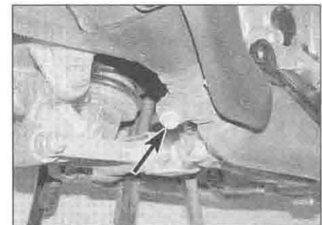
13.2e On XRV models, slacken the clamp bolt (arrowed) ...
