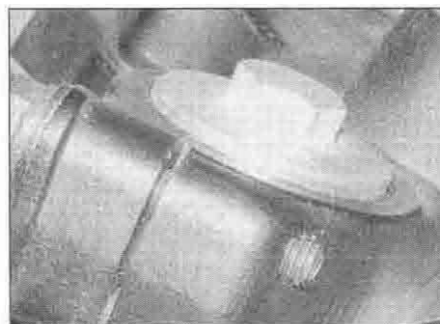
6.7 Set the fork height as shown, making sure it is the same on both sides
