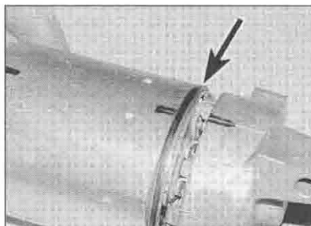
29.4a Remove the rear cover and its sealing ring (arrowed) . . .
