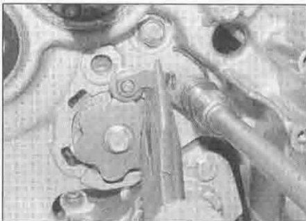
20.12b ... then position the arm on the cam and tighten the bolt
