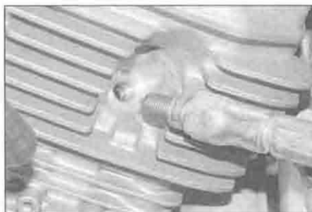
5.9 Fit the plug into the tool (the rubber insert should grip around the plug top) and thread it in by hand
