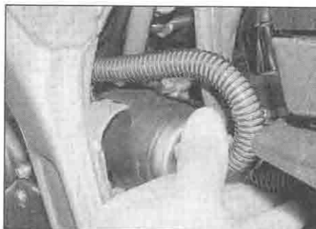
15.14 Draw the pump off its mounting lug and remove it
