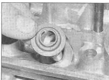
14.25 Fit the spring seat, making sure it is the correct way up
