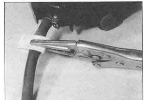
9.4 ... or thick card and self-locking grips
