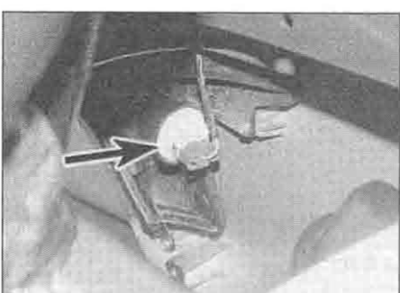
12.4c Release the bulbholder (arrowed) ...
