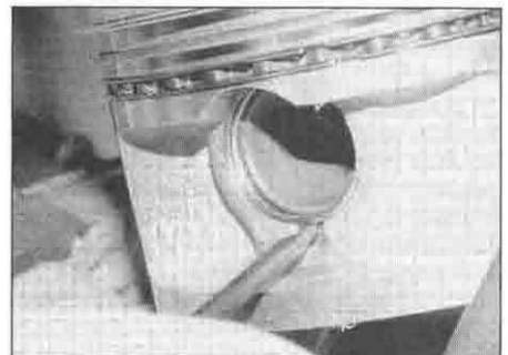
16.3a Prise the piston pin circlip out from one side of the piston
