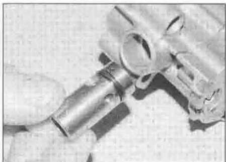
25.12a Withdraw the relief valve from the pump
