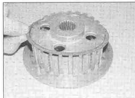
18.29a Fit the spring seat ...
