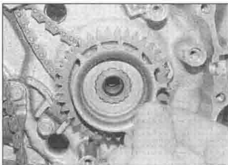
21.8 ... and on XL models the timing rotor
