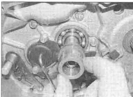
18.24 Slide the clutch housing guide onto the shaft . . .
