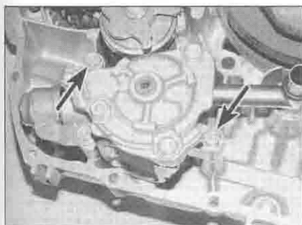
25.3a Unscrew the bolts (arrowed) ...
