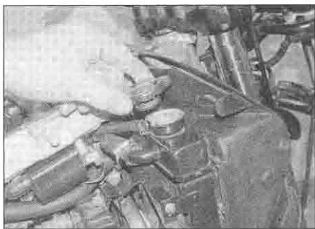
18.8 Remove the pressure cap as described
