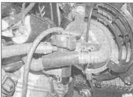
17.1 PAIR system control valve – XL650V models
