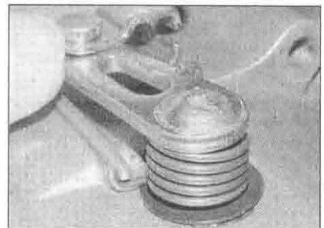
18.21d . . . and the spring ends locate correctly
