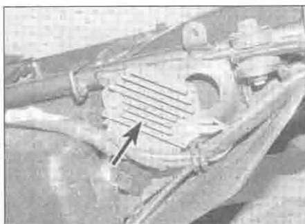
33.1b Regulator/rectifier (arrowed) - XL650V
