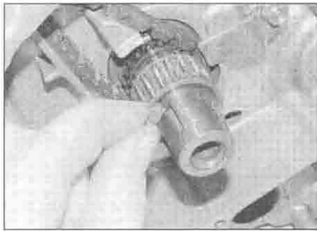
32.13 Fit the Woodruff key into its slot
