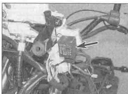
11.3b Turn signal relay (arrowed) – XL650V
