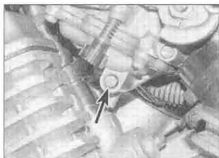
7.9a Carburettor drain screw (arrowed) – XL models
