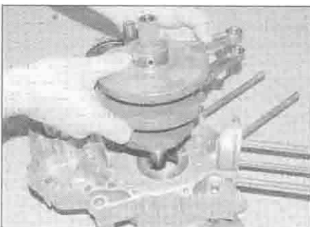
27.2 Lift the crankshaft out of the crankcase
