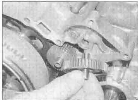
32.15b ... and the starter drive gear
