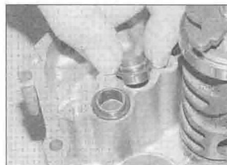
25.3c Remove the oil passage dowels ...
