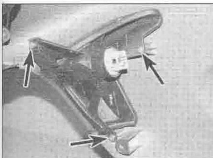
13.3b Turn signal screws (arrowed) – XL650V
