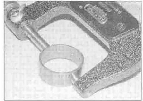
31.20b ... and the external diameter of its bush
