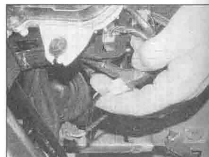
5.8d ... and the sidelight wiring connector
