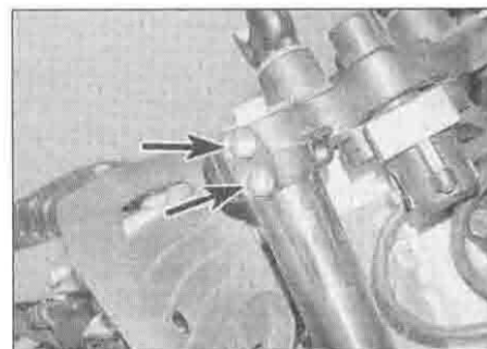
6.4a Slacken the fork clamp bolts (arrowed) in the top yoke ...
