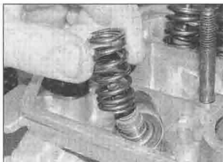
14.28a Fit the inner valve spring ...
