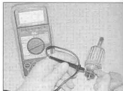
29.11 Continuity should exist between the commutator bars
