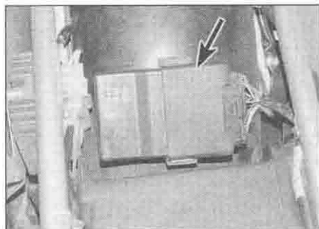
5.3a Ignition control unit (arrowed) – XL600V
