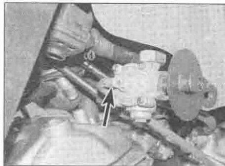
2.3b ... and the vacuum hose (arrowed)
