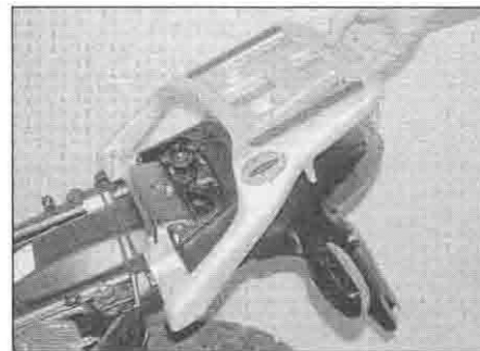
5.22c ... and remove the rack ...
