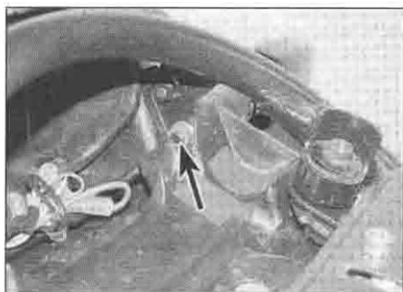
13.8b Rear turn signal nut (arrowed) – XL650V
