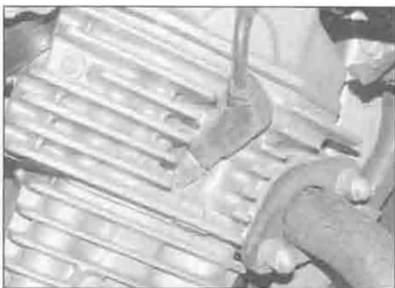
5.2a Front cylinder – right-hand plug
