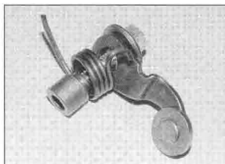
20.8b ... and the stopper arm assembly as described
