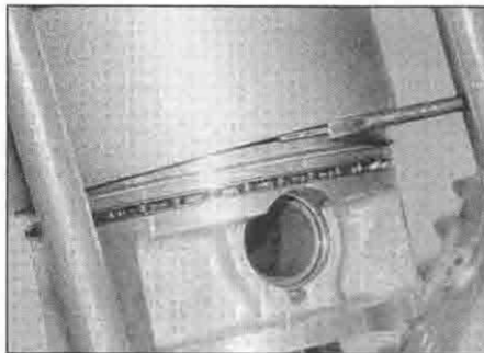
15.23 . . . and feed the piston rings into the bore
