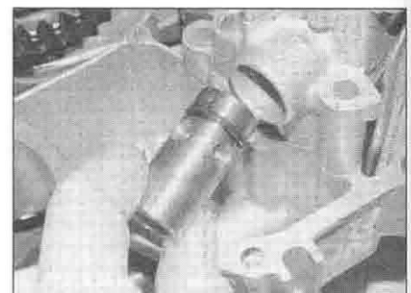
25.2c ... and withdraw the pressure relief valve
