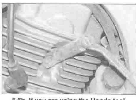
5.5b If you are using the Honda tool, locate it onto the plug and use a ring spanner to turn it
