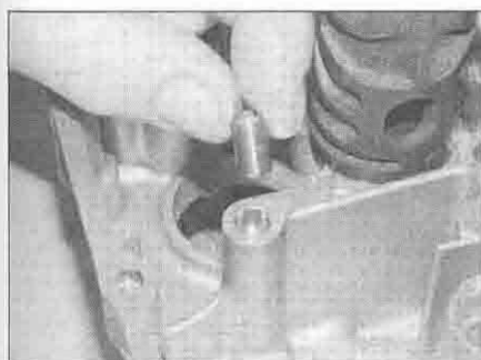
25.3d ... and the pump dowel
