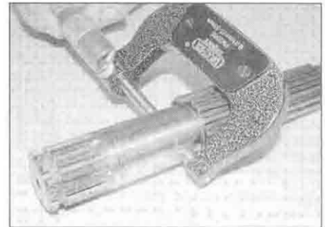
31.20d ... and the external diameter of the shaft
