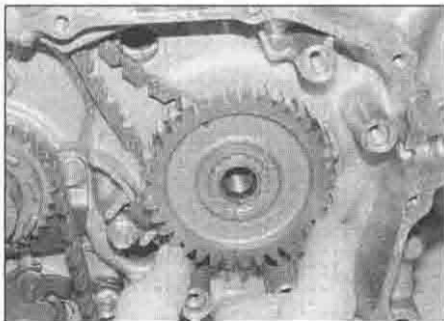
21.5 Slide the primary drive gear off the shaft
