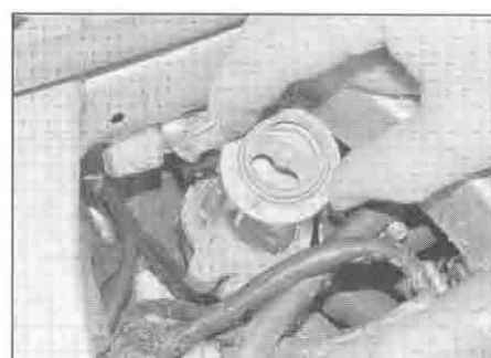
5.4c . . . and lift out the thermostat
