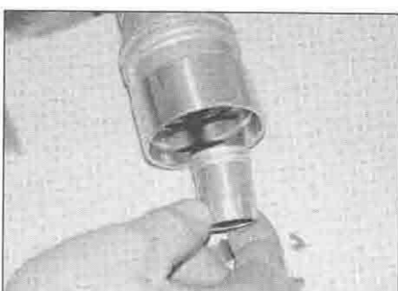
8.13 Remove the damper rod seat from the slider
