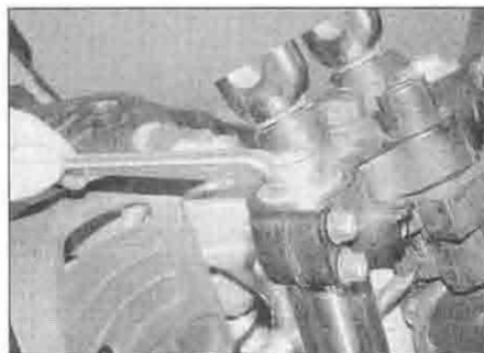
6.4b ... and if required the fork top bolt
