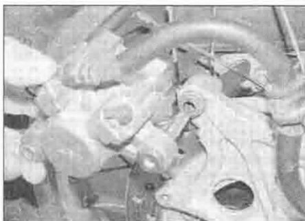
5.2 Slide the caliper off the bracket
