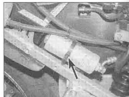
11.10b Slacken the clamp screw (arrowed) and draw the reservoir out
