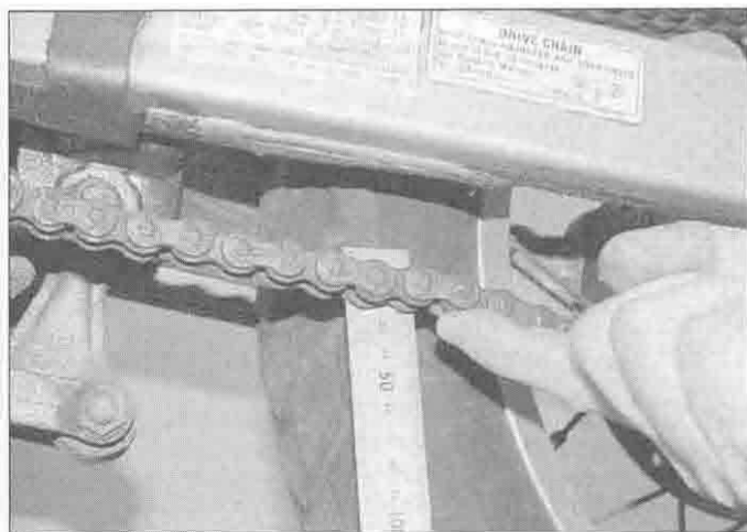
1.3 Push up on the chain and measure the slack
