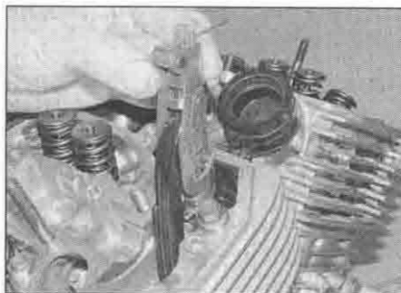
11.4b ... then withdraw the tensioner ...
