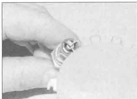
5.8a Using a wire type gauge to measure the spark plug electrode gap
