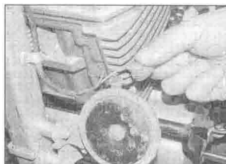
26.2 Disconnect the wiring connectors
