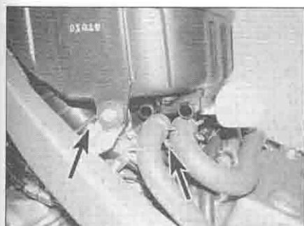
4.10 Slacken the clamp screws (arrowed)
