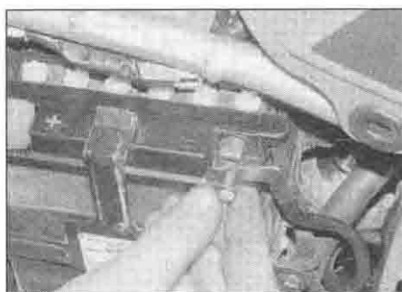
3.2a Disconnect the negative lead first ...
