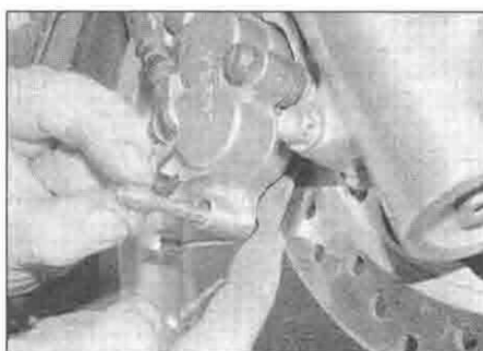
2.20d Press the pad up against the spring and insert the retaining pin
