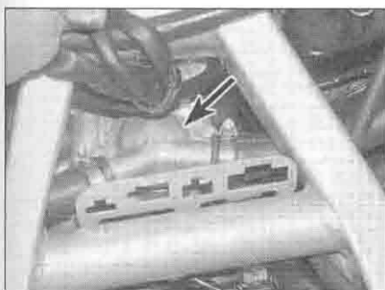
5.3c . . . to access the thermostat housing (arrowed)
