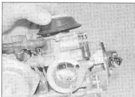
10.12a Fit the piston into the carburettor ...
