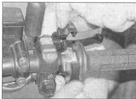
11.8a Assemble the housing ...
