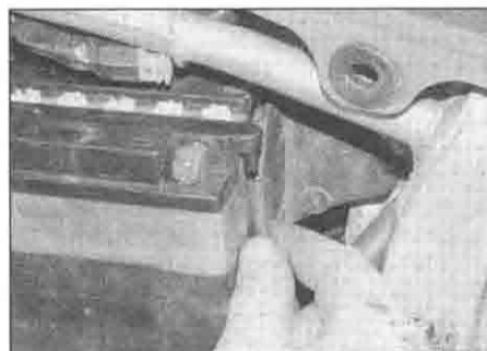
3.3c Disconnect the breather tube
