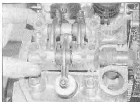
9.6c ... and remove the holder, noting how it fits
