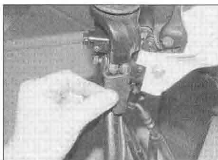
15.4a Pull back the rubber boot to access the adjuster
