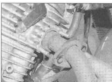
13.3d Draw the flange off the studs ...
