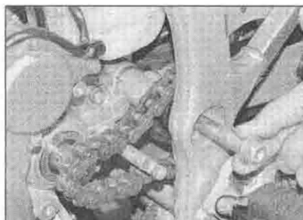
14.5d ... withdraw the bolt ...
