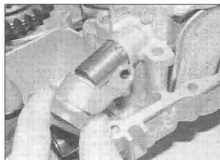
25.2b ... and remove the cover ...
