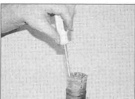
13.7a Dig out the old sealing ring ...
