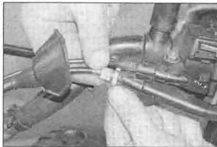
19.4 Pull back the rubber cover, then slacken the lockring and thread the adjuster fully in
