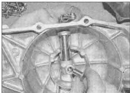
18.34 Align the shaft and install the release rod
