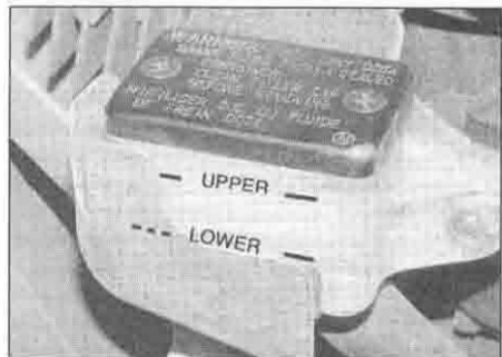
8.4a Master cylinder reservoir – XL600V
