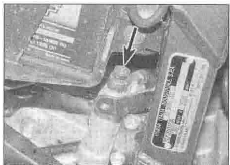
8.5 Brake hose banjo bolt (arrowed)
