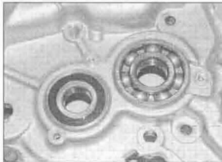
31.22 Check the transmission shaft bearings
