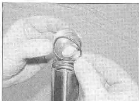
7.16 Fit the top bolt using a new O-ring
