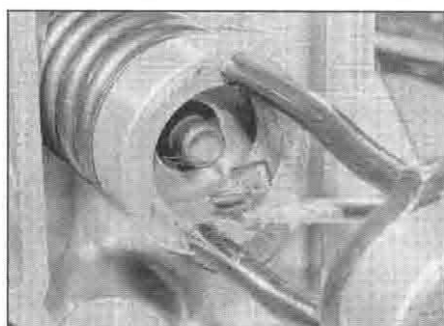
14.5c Remove the collets as described
