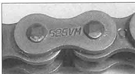
8.10 Typical chain size and type marking
