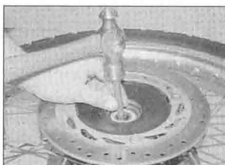
15.4a Knock out the bearings using a drift . . .
