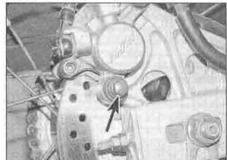
2.33a Unscrew the bolt (arrowed) . . .
