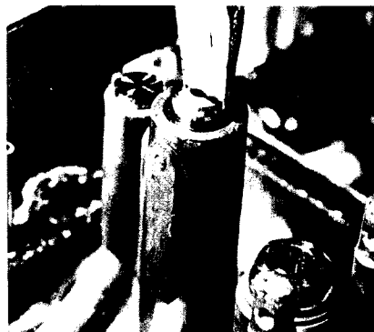
Unscrewing the main jet
