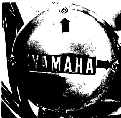
Alternator rotor cover allen bolts
