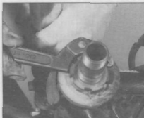
19.7 The ring nut can be tightened with spanner wrench (C-spanner)
