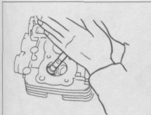
12.24a After lapping, the valve face should exhibit a uniform, unbroken pattern . . .
