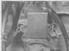
15.5 Remove the mounting screws (arrowed) to detach the ignition main (key) switch
