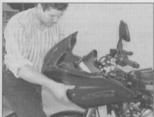
5.7d Manoeuvre the fairing forwards, splying its sides out to clear the turn signal mounts
