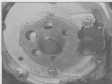
25.11 When the signal generator rotor tab opposite the T mark is aligned with the pick-up coil protrusion, no. 2 and 3 cylinders are at TDC; the valves for the cylinder which is on its compression stroke can be adjusted
