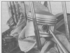
14.3b Remove the circlip from one side of the piston – wear eye protection and be careful not to let it fly out
