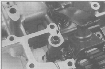
22.9 The dowel inside the case has an O-ring (arrowed)
