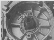
31.3b Remove the oil nozzle (arrowed)
