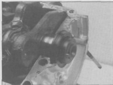
22.14a If the end seal has a lip, make sure it's seated securely in its groove . . .
