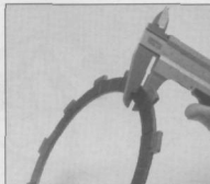
18.14 Measure the thickness of the friction plates
