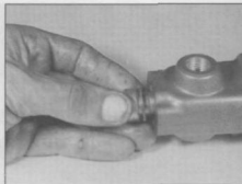
6.4c . . . and remove the bolt and its copper washer – use a new copper washer during reassembly
