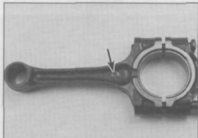
26.2b If there's an A mark on the side of the connecting rod, it faces the right side of the engine; if there's any other mark, carefully note which way it faces before removing the connecting rod
