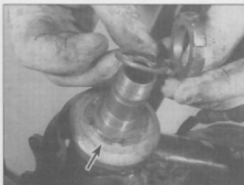
7.5b ... unscrew the upper ring nut, lift off the rubber washer and unscrew the lower ring nut (arrowed)
