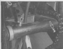
24.1 Lubricate the swingarm through the grease fittings (arrowed)
