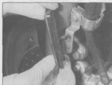
2.1a Remove the nut and detach the reflector from the mount ...
