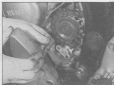
12.2b . . . and take off the engine sprocket cover and bolt spacer
