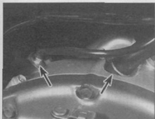
5.8 Remove the crankcase ventilation hose and disconnect the ground (earth) cable (arrowed)
