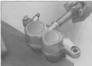
3.5 Blow air into the bleed valve hole to force the pistons out, DO NOT get your fingers in the way; use rags or a piece of wood to catch the pistons
