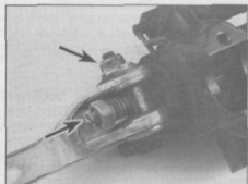
5.7 Remove the snap-ring (left arrow); undo the locknut (right arrow) and unscrew the pivot bolt
