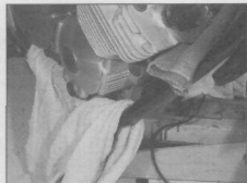
5.16b ... and pad the frame with a thick layer of rags so it won't be scratched as the engine is removed
