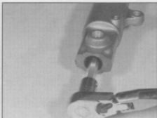
6.4b Loosen the damper rod bolt with an Allen wrench . . .
