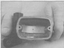
5.8 Lift the splash plate (if equipped) out of the cylinder body so you can clean the fluid ports in the bottom
