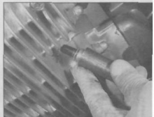
4.2 Use an extension and a deep socket to remove the spark plugs
