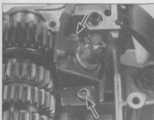
27.9 The starter chain tensioner piston is secured to the crankcase by two Allen bolts
