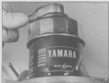
18.6a This tool is used to remove the oil filter . . .
