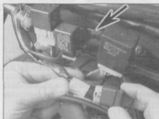
15.12a Disconnect the heater relay from its mounting tab (arrowed) and disconnect its wiring
