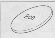
25.24 There's a thickness mark on the underside of each valve shim (be sure to place the marked side of the shim down during installation)
