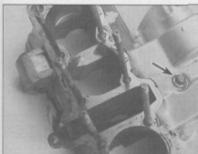
27.7 This bolt secures the cam chain rear (intake side) guide; don't remove it unless you plan to separate the case halves
