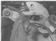
6.8 Lift the master cylinder up and over the footpeg bracket, then undo the union bolt
