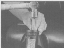
7.11 Drive the lower bearing outer race out from above; drive the upper bearing outer race out from below
