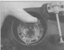
7.2a Lift the retaining clip to free the bulb ...
