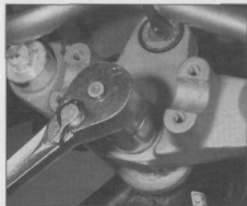
7.4b Unscrew the steering stem nut
