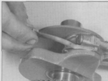
26.1 Measure the clearance between the crankshaft and the connecting rod with a feeler gauge
