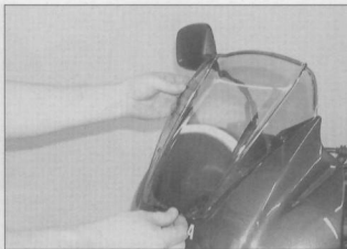
5.4b ... and remove the windshield
