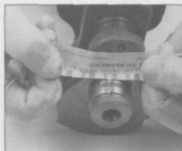
25.11 Measuring the width of the crushed Plastigauge (be sure to use the correct scale – standard and metric are included)
