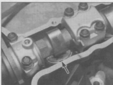
25.17 The valve lifter notch (arrowed) should be toward the centre of the engine
