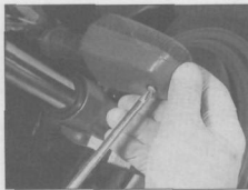
9.1 To replace a turn signal bulb, remove the screws and take off the lens
