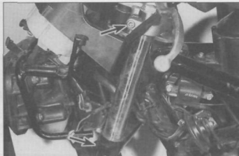
5.6 Loosen the triple clamp bolts (arrowed) and lower the fork out of the triple clamps
