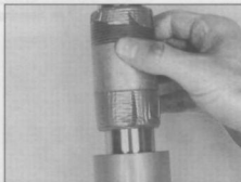
6.16b ... if you don't have the proper tool, a section of pipe can be used the same way the special tool would be used - as a slide hammer (be sure to tape the ends of the pipe so it doesn't scratch the fork tube)
