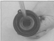
7.16a Remove the screw inside the throttle piston ...
