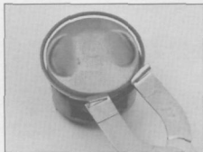
14.6 Remove the piston rings with a ring removal and installation tool
