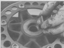
13.18 Lift the collar out of the brake disc side of the wheel
