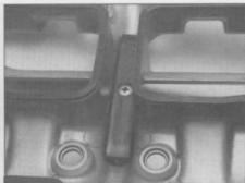
7.7 Replace the upper cam chain guide inside the valve cover if it's worn or damaged
