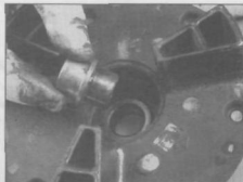
13.16 Remove the coupling collar; don't forget to install it later or the bearings will be ruined
