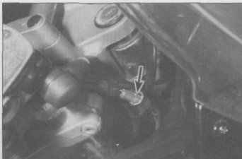
5.13 To adjust throttle freeplay, pull back the rubber boot from the mid-line adjuster, loosen the locknut, turn the adjuster (arrowed), then tighten the locknut
