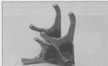
30.3 Reassemble the forks onto the guide bar so they don't get mixed up; the number on each fork faces the right side of the engine when the forks are installed
