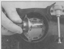
7.2b ... and pull the bulb out; be careful not to touch the bulb glass with your fingers
