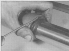
6.6 Pry the dust seal out of the outer tube
