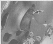
11.7c Align the fork leg protrusion with the notch in the speedometer drive unit (arrowed)
