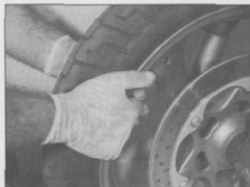
19.4 Grasp the front wheel and try to pull it back and forth; if it moves, the steering head bearings are loose and in need of adjustment
