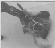
5.10b ... then pull out the pushrod
