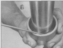
6.7 Pry out the retaining ring
