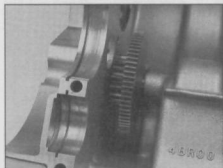
31.9a The idler gear should look like this when it's installed . . .
