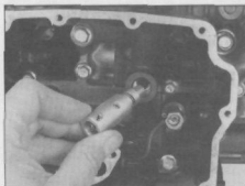
16.7a Pull the main oil relief valve out of the crankcase ...
