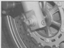
11.4b Axle clamp bolt and axle head – 1998-on UK models
