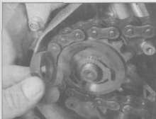
13.6b . . . the recessed side of the nut faces the sprocket
