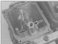
7.12b ... and note the position of the needle jet alignment pin
