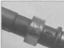
9.12b Check the lobes of the camshaft for wear – here's a good example of damage which will require replacement (or repair) of the camshaft
