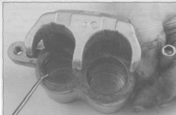
3.7a Remove the dust seal and piston seal from each bore with a pointed tool; this is a front caliper ...
