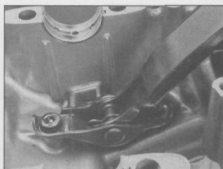
27.8b The starter chain lower guide is secured to its bracket by a clip and pivot pin; the bracket is secured to the case by two Allen bolts
