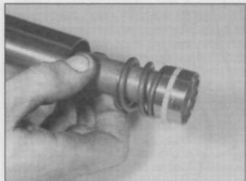
6.5 Remove the damper rod and the Teflon ring – don't separate the ring from the damper rod unless you plan to replace it
