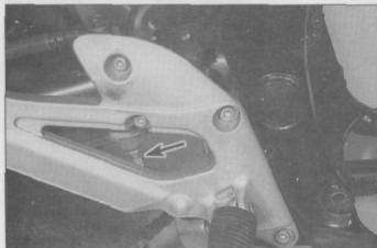
8.3b To adjust the brake pedal height, loosen the locknut (arrowed) and turn the adjusting bolt
