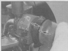
5.9 Throttle cable freeplay is measured at the grip flange
