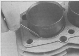
13.13a Install a new O-ring around the base of each cylinder press it completely into its groove. . .
