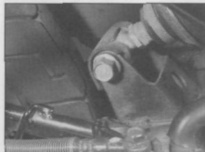
8.3c ... and the lower mounting bolt and nut and lift the shock absorber out
