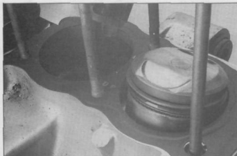
13.13b . . . then, install the new gasket between the block and cylinder assembly, making sure the UP mark is up . . .
