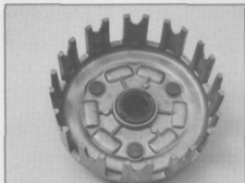
18.10 Slide the clutch housing off and remove the thrust washer
