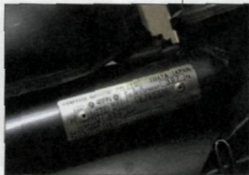
The frame number is printed on a label on the right side of the frame ...
