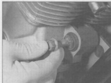
5.17a With the engine supported by a jack, remove the engine mounting bolts at the upper front . . .
