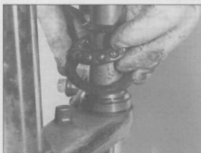
7.8 Carefully lower the steering stem out of the steering head and remove the rubber washer, lower bearing and dust seal
