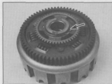
18.17 Remove the snap-ring (arrowed) and take off the oil pump drive gear if its damaged
