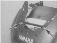
5.7a The fairing is retained at the front by two screws (arrowed) ...
