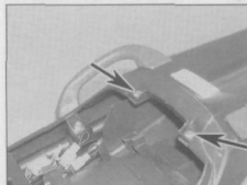
3.9a The tail cover is retained by two screws (arrowed)
