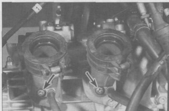
6.6a Remove the vacuum fitting screws (arrowed) . . .
