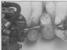
7.18c ... then unscrew the choke plunger cap and pull out the spring and the choke plunger
