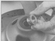
11.7a There's a collar in the right side grease seal
