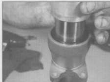
6.16a Drive the bushing into position with a tool like this one if it's available (use the tool like a slide hammer) ...
