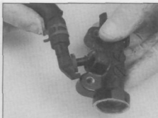
6.10a Pry the fluid feed hose fitting out of the grommet ...
