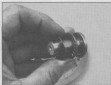
18.19 Check the release bearing for worn or damaged rollers
