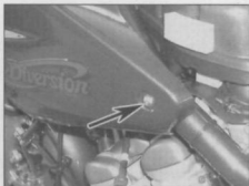
5.7b ... a screw on each side (arrowed) ...
