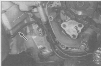
4.2 Follow the pick-up coil harness (arrowed) to its connector
