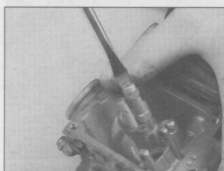
7.9 Unscrew the main jet and lift it out with its washer
