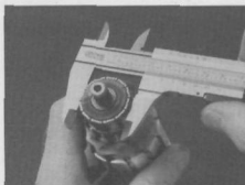
24.5 Check the commutator for cracks and discoloration, then measure its diameter
