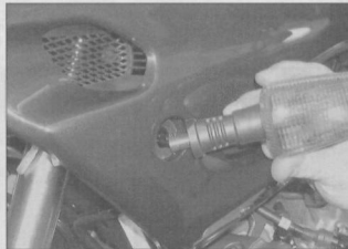
5.6b ... and withdraw the turn signal from the fairing
