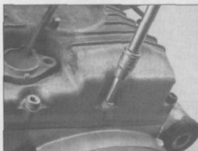
16.2 Remove the oil pan bolts around the edge of the pan
