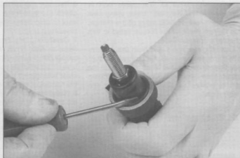
6.16 Push the rubber boot into its groove
