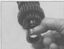
29.3b Remove the bearing and snap-ring from the end of the shaft
