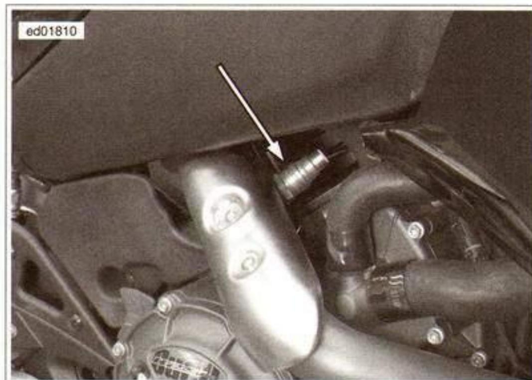
Figure 6-43. Rear O2 Sensor Location
