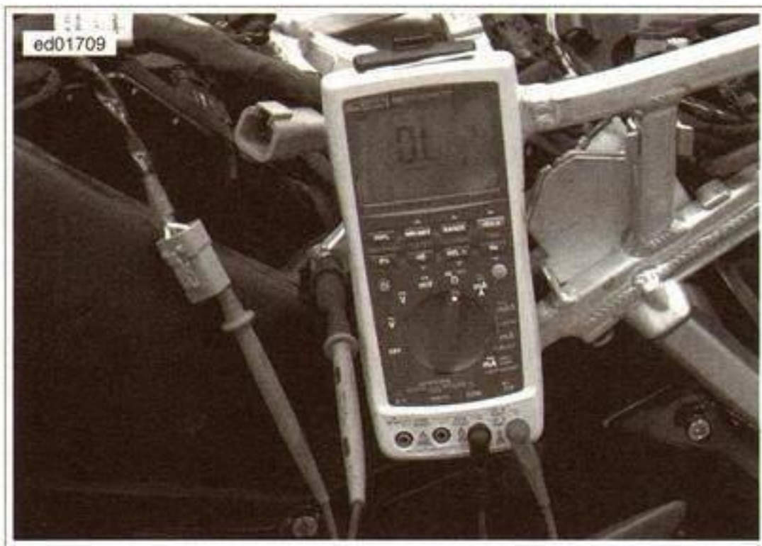
Figure 3-16. Test for Grounded Stator (typical)
