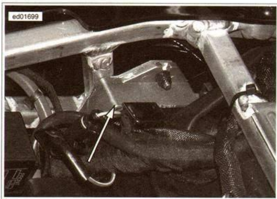
Figure 3-11. Voltage Regulator Location
