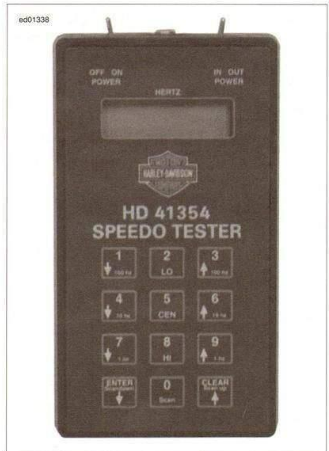
Figure 1-23. Speedometer Tester (Part No. HD-41354)
