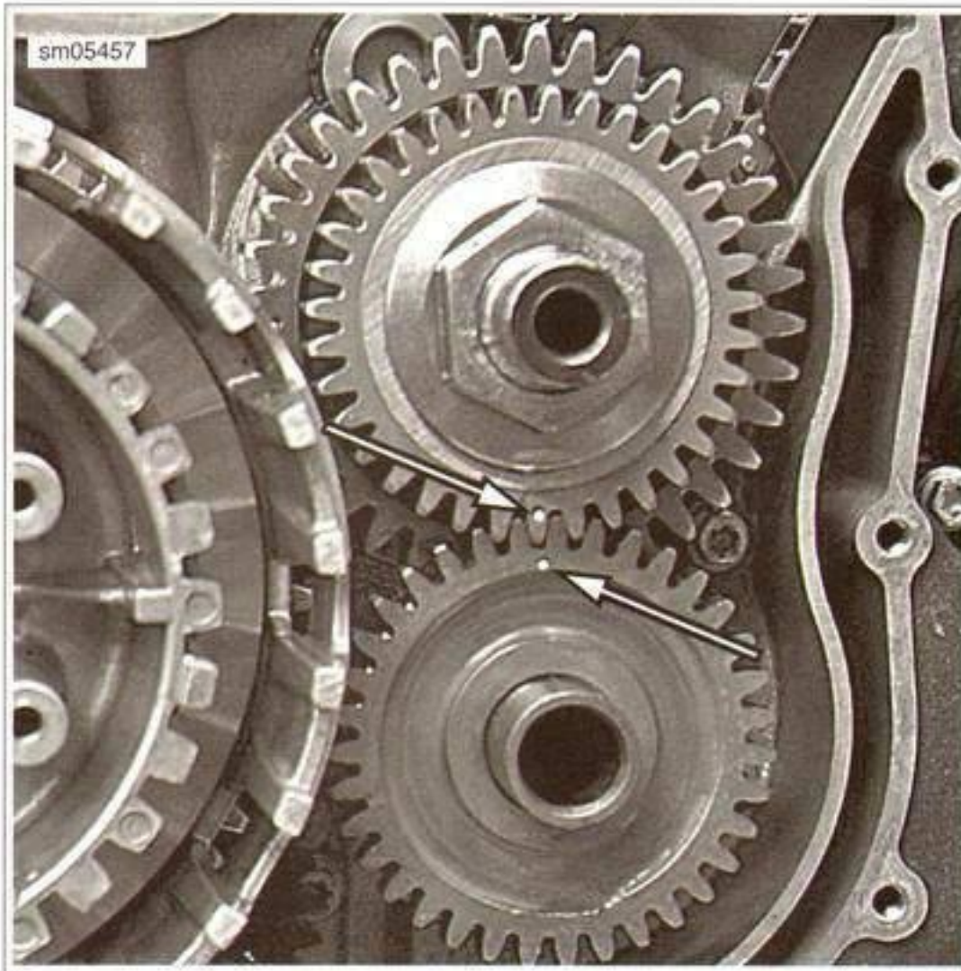
Figure 3-123. Balancer Timing Marks
