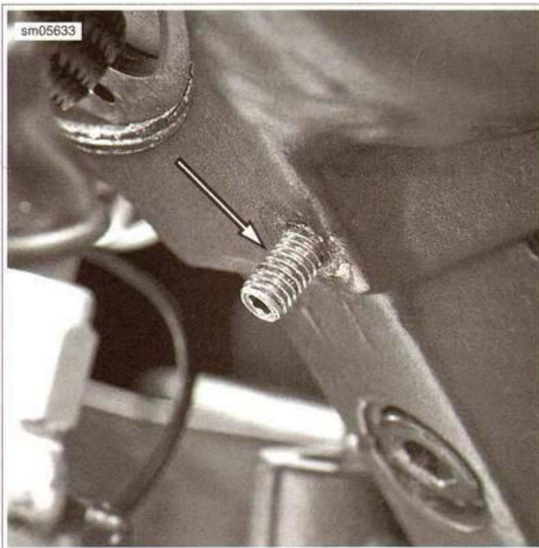
Figure 4-61. Fuel Pump Cover Set Screw
