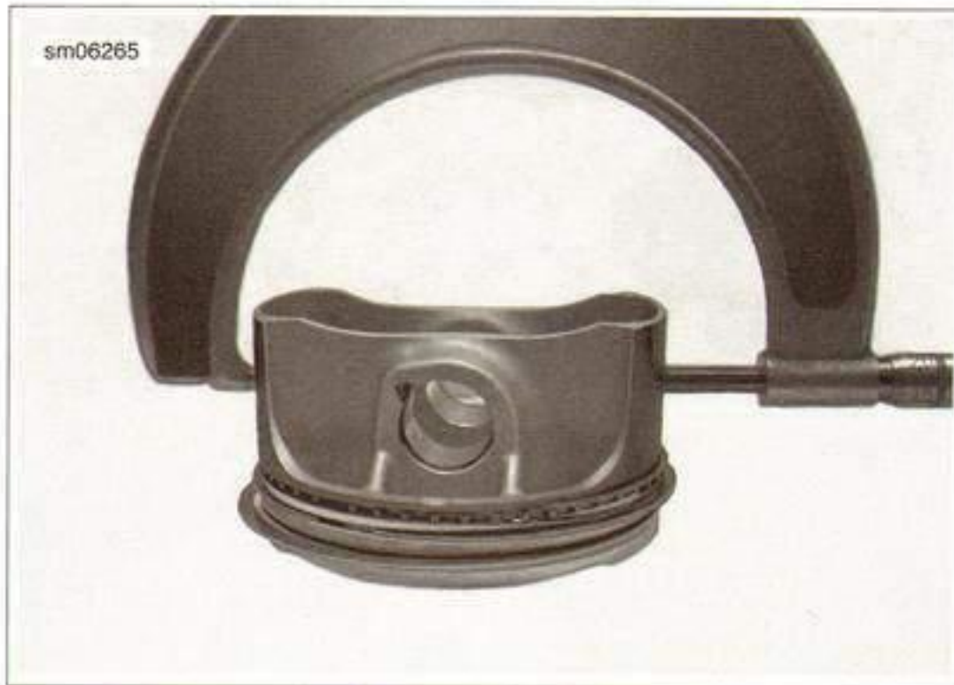
Figure 3-100. Measuring Piston Diameter
