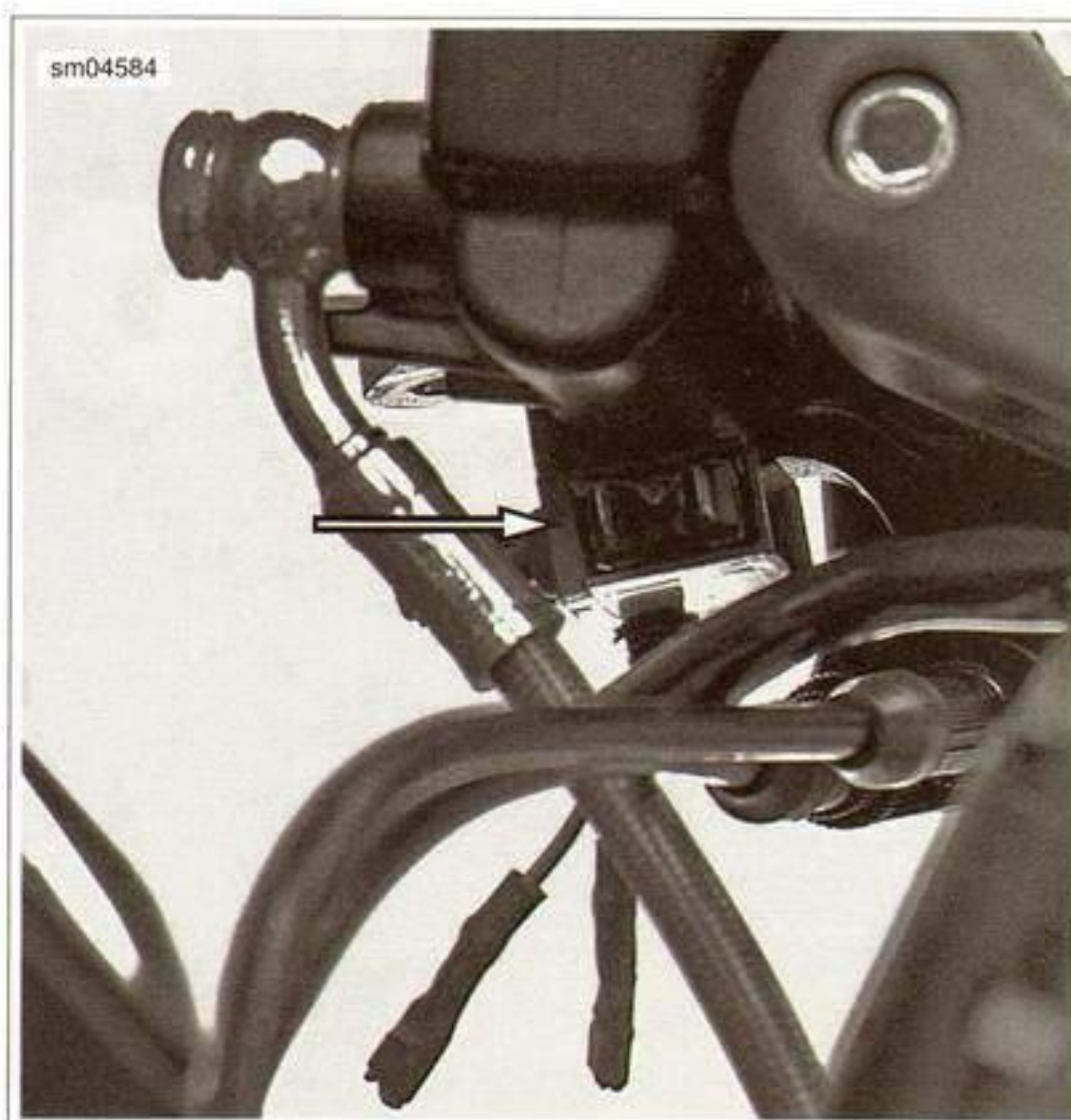
Figure 2-50. Brake Light Switch Spade Connectors
