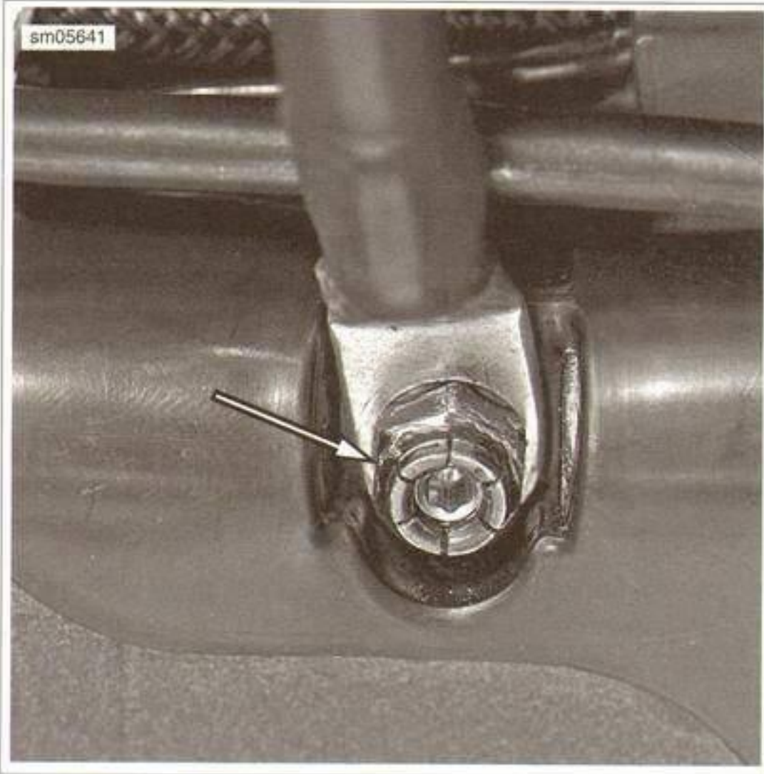
Figure 7-13. Negative Battery Cable Ground
