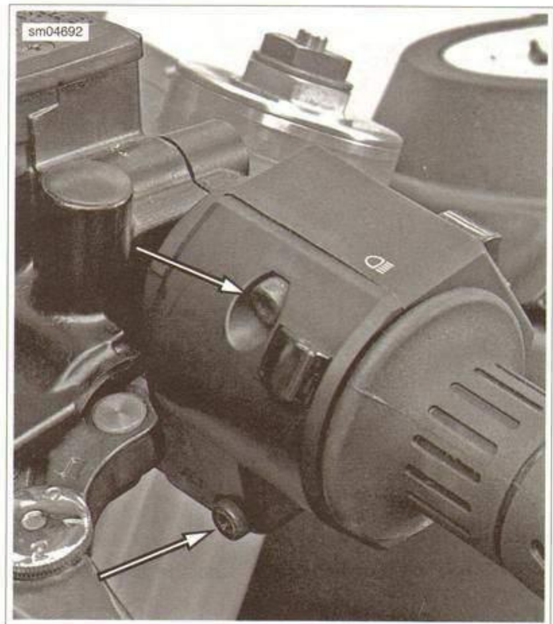
Figure 7-98. Left Handlebar Switch Housing Fasteners
