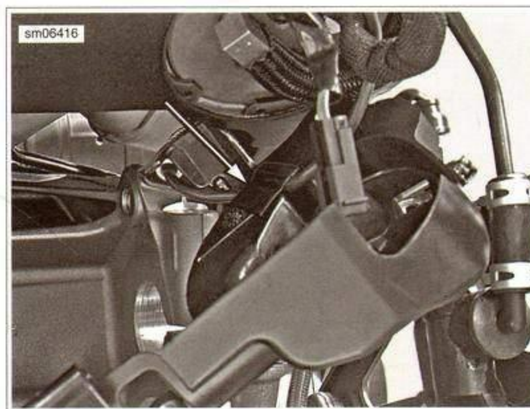
Figure 4-68. VSS Lead Taped in Cover
