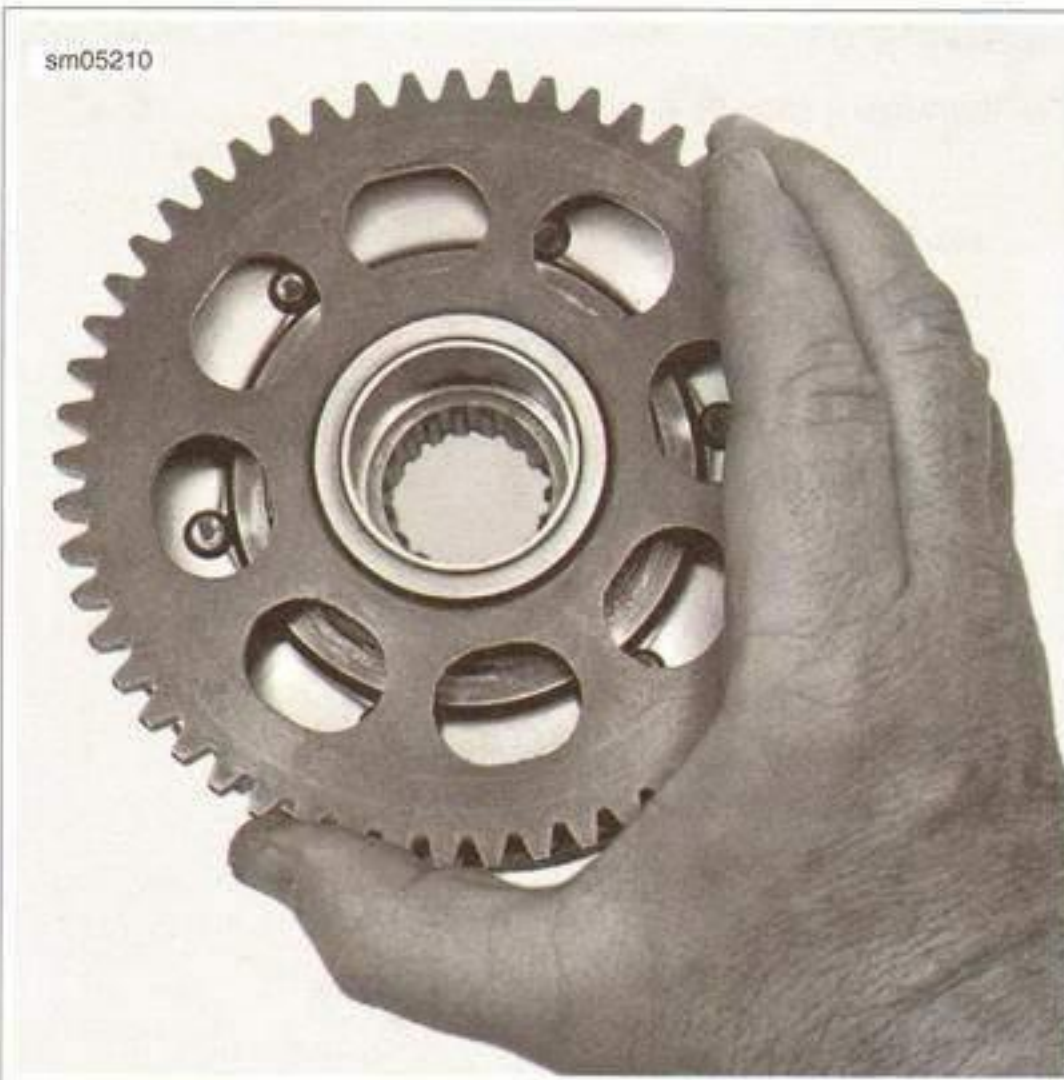
Figure 7-37. Rotate Starter Gear to Fit Sprag Clutch
