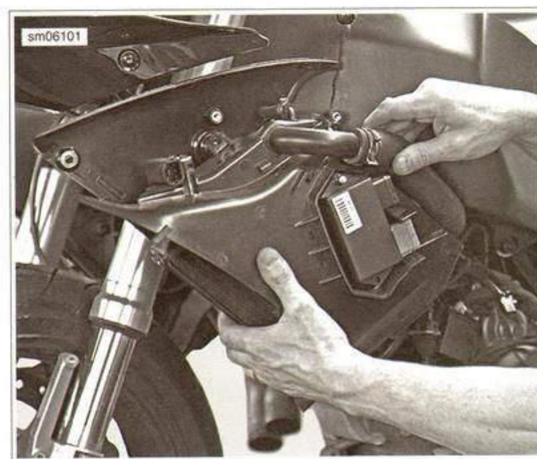
Figure 3-33. Removing the Radiator
