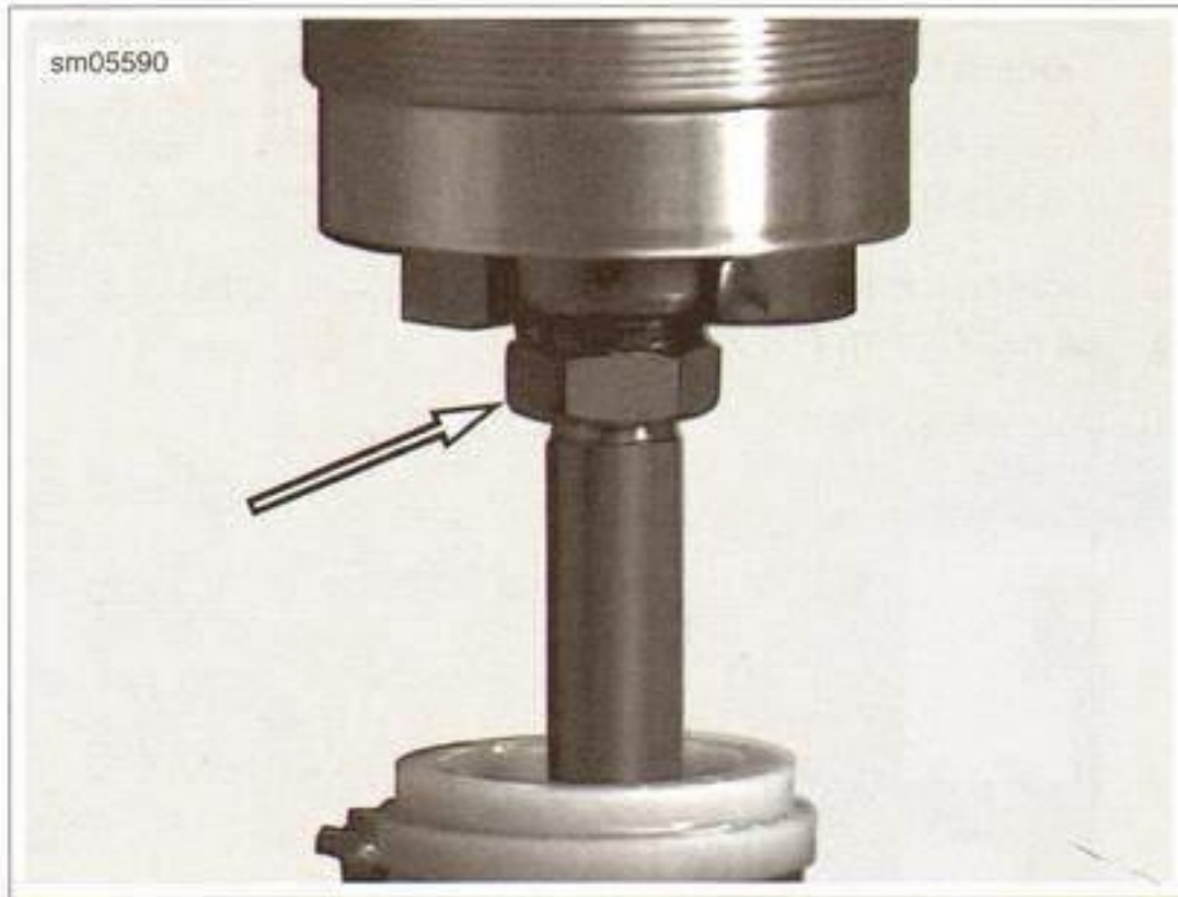
Figure 2-95. Damper Rod Jamnut
