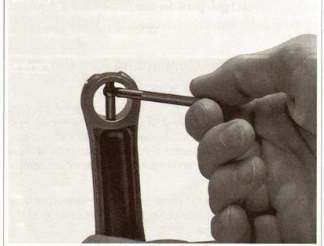
Figure 3-97. Connecting Rod Piston Pin Bore Measurement
