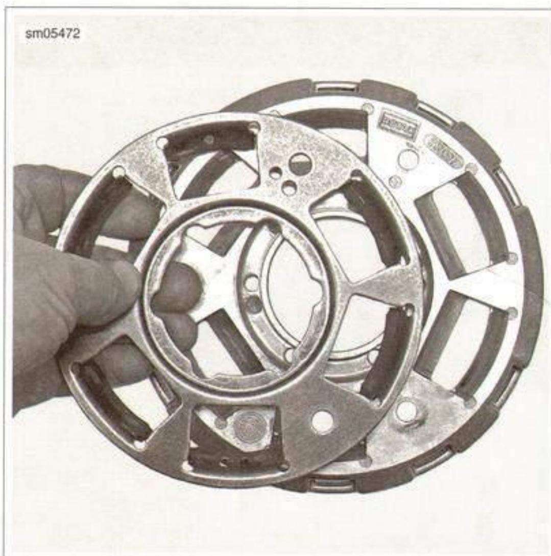
Figure 6-54. Inner Support Plate and Clutch Drum
