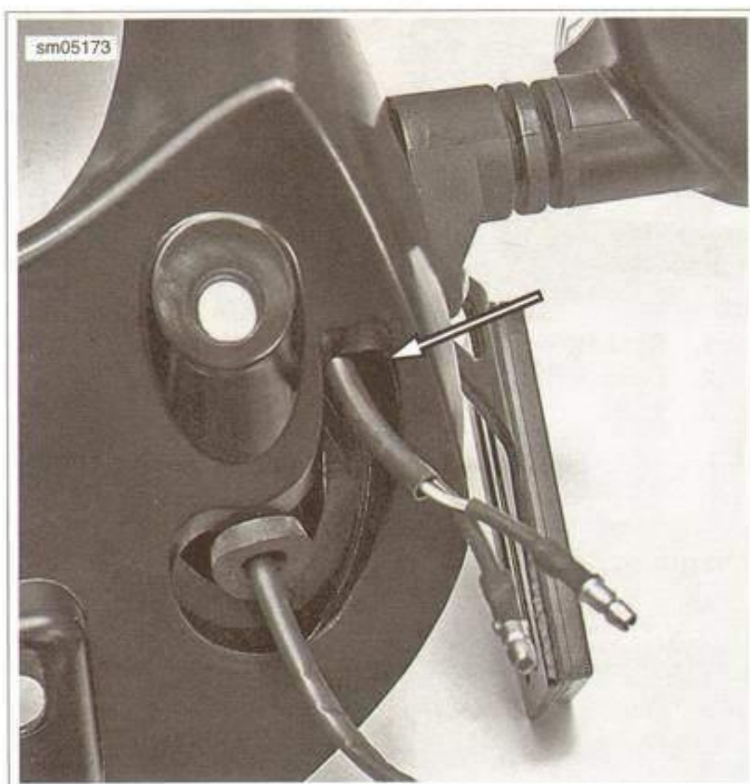
Figure 7-65. License Plate Wiring Through J-shaped Opening
