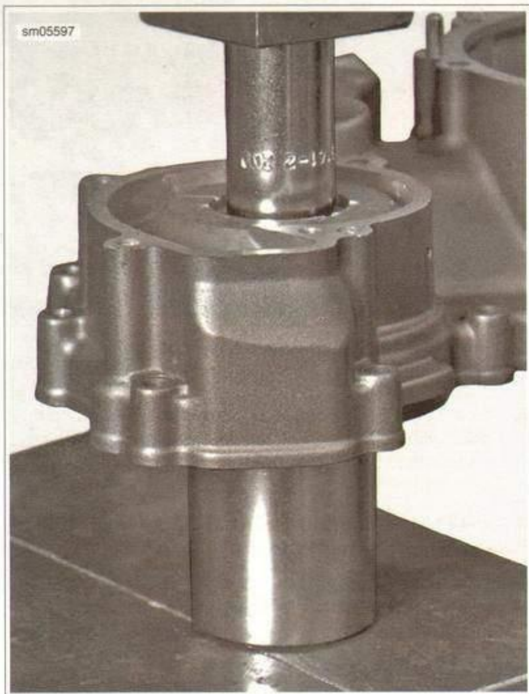
Figure 5-20. Installing Inner Oil Seal
