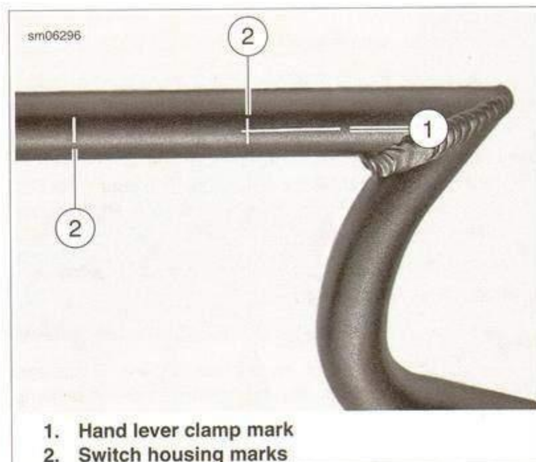
Figure 7-101. Hand Lever Clamp and Switch Housing Marks: 1125CR
