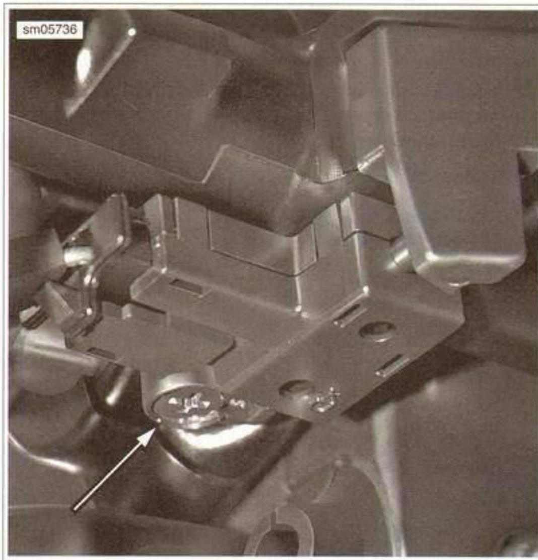
Figure 7-82. Clutch Interlock Switch Fastener
