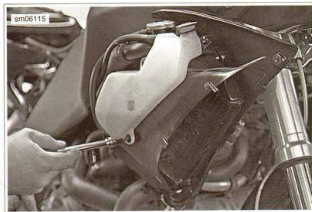
Figure 3-32. Remove Overflow Tank
