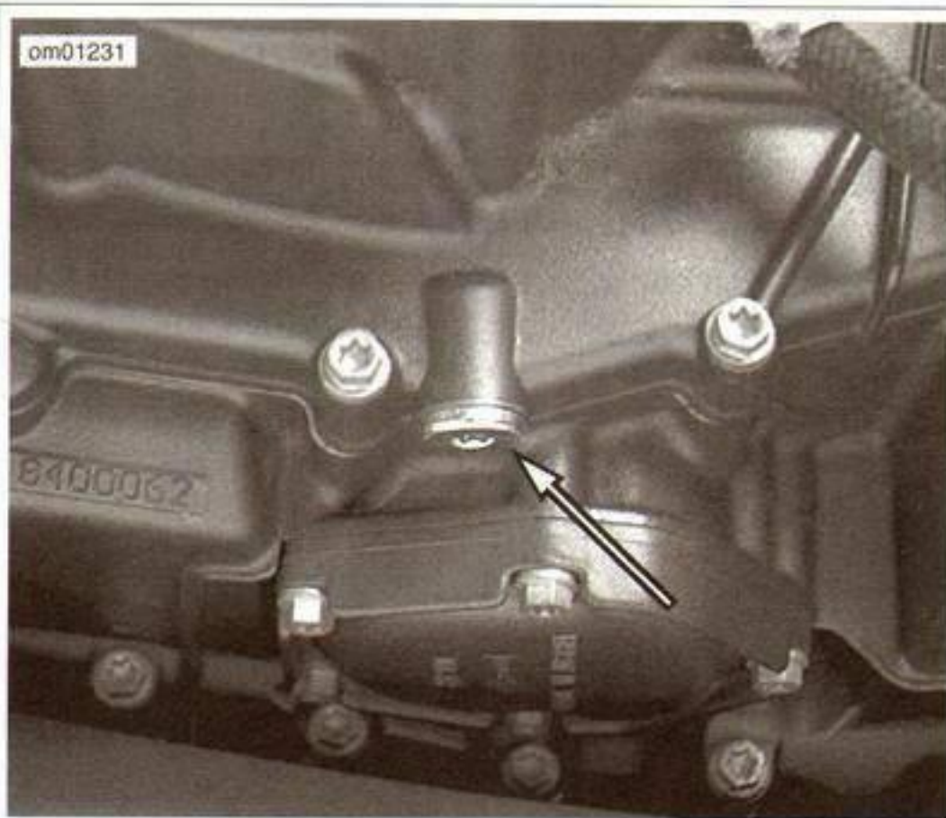
Figure 1-4. Engine Oil Drain Plug (Right Side): Buell 1125 Models
