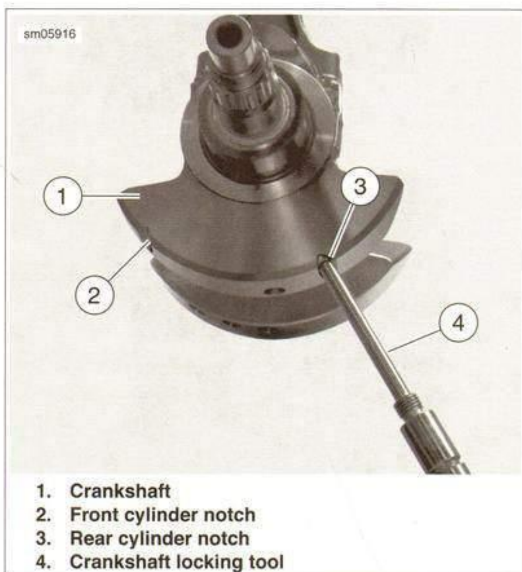
Figure 3-61. Locking Crankshaft
