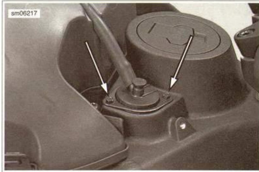
Figure 4-55. Fuel Vent Valve Fasteners
