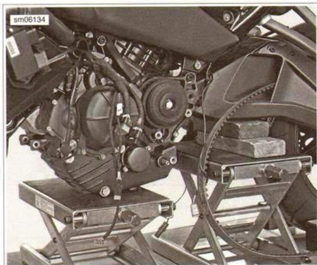
Figure 3-38. Support Engine and Swingarm
