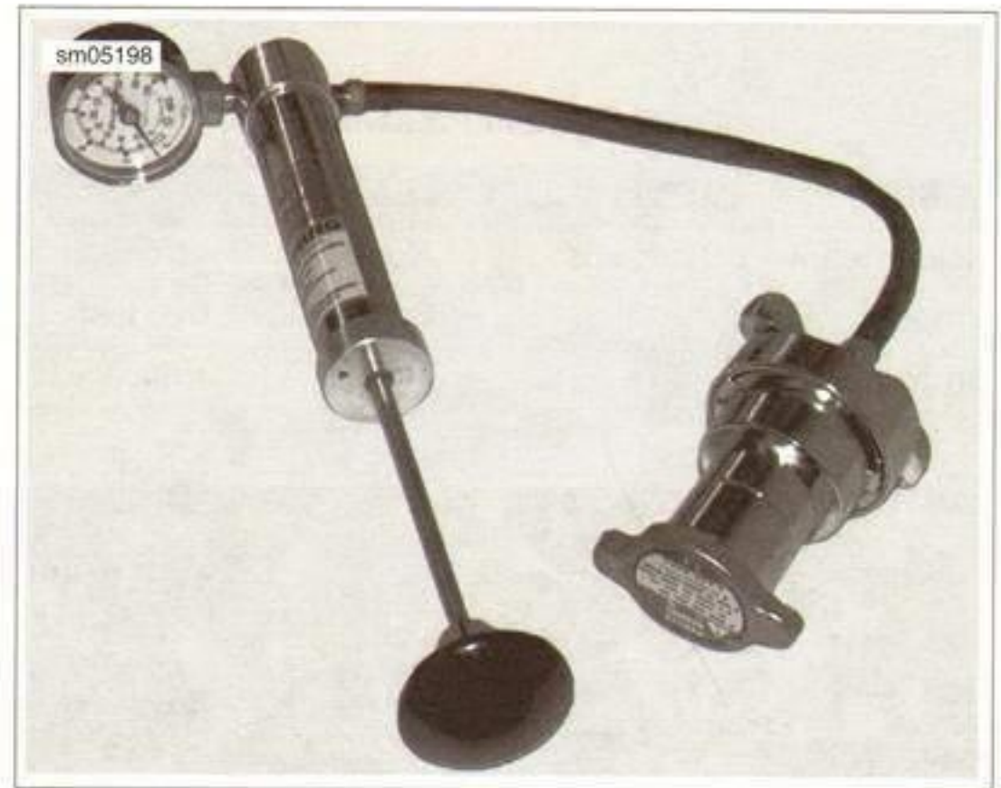
Figure 5-4. Pressure Cap Test
