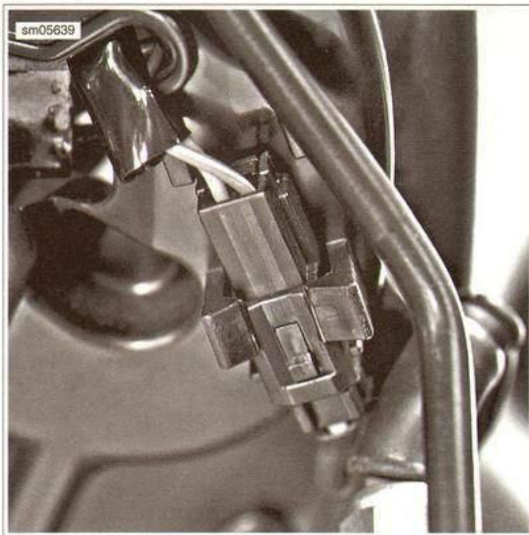
Figure 4-69. Brake Light Switch Connector [121]
