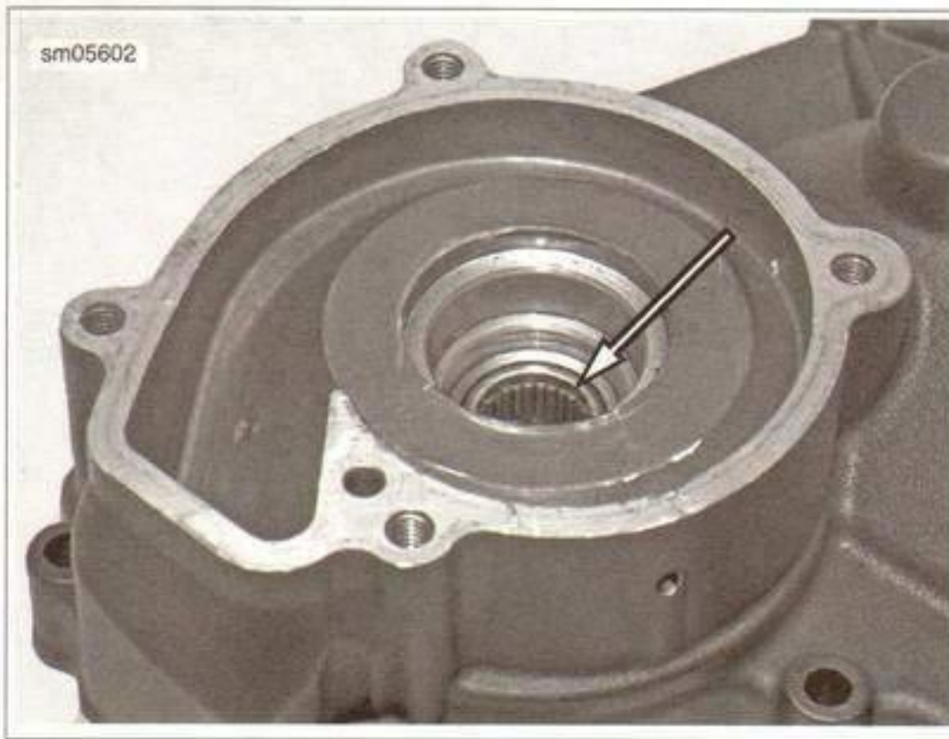
Figure 5-16. Bearing in Side Cover
