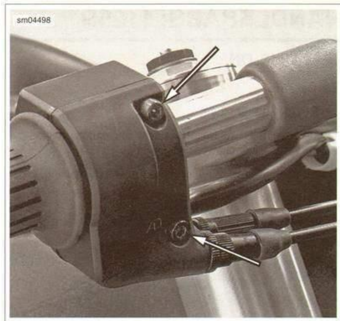
Figure 2-142. Switch Housing Fasteners
