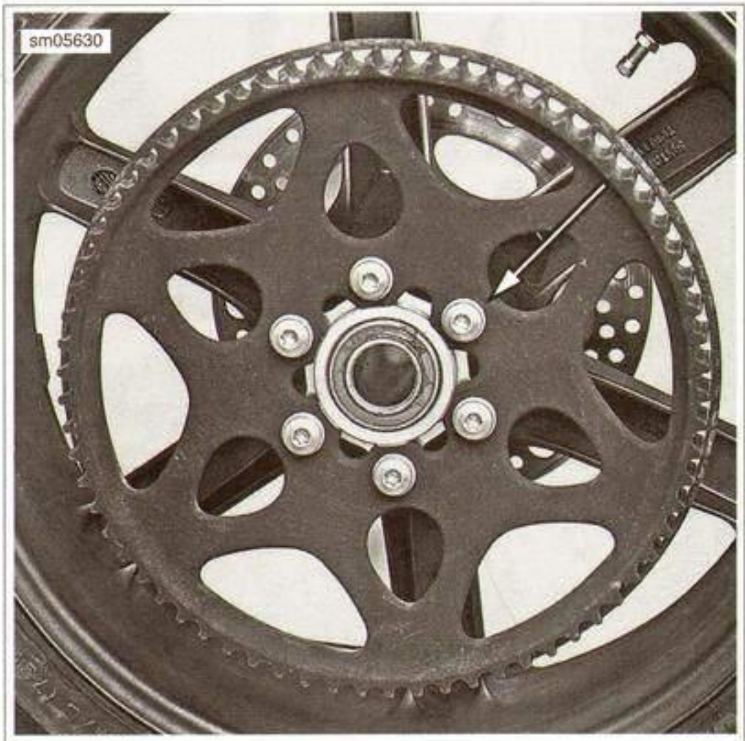
Figure 2-34. Drive Sprocket Fasteners
