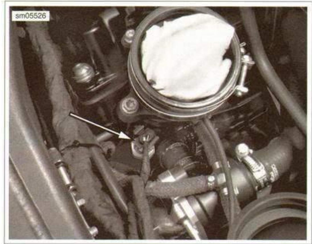
Figure 3-22. Engine Temperature Sensor
