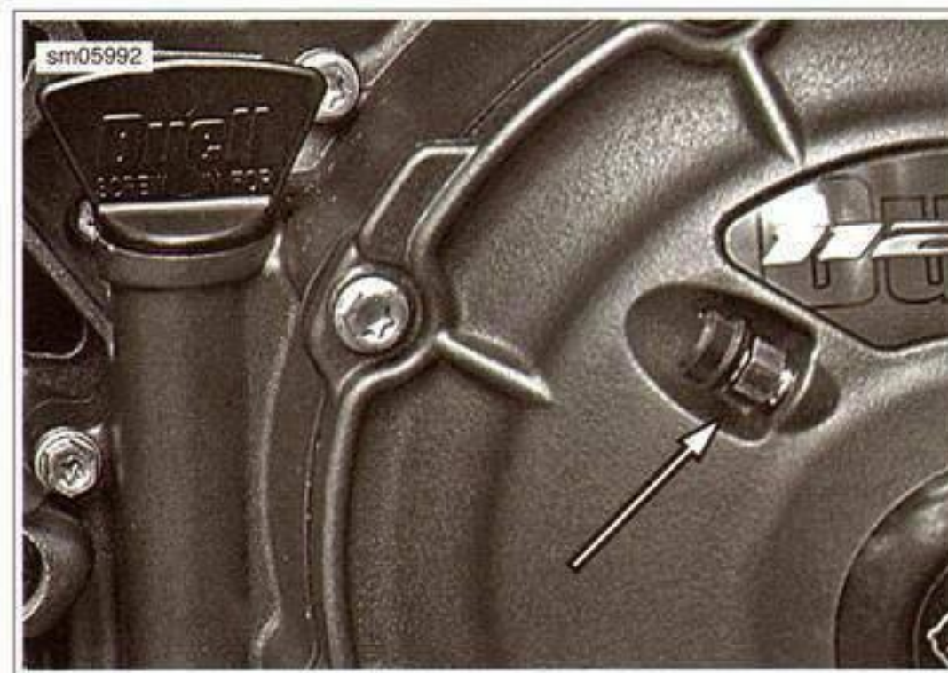
Figure 1-16. Clutch Fluid Bleeder Valve
