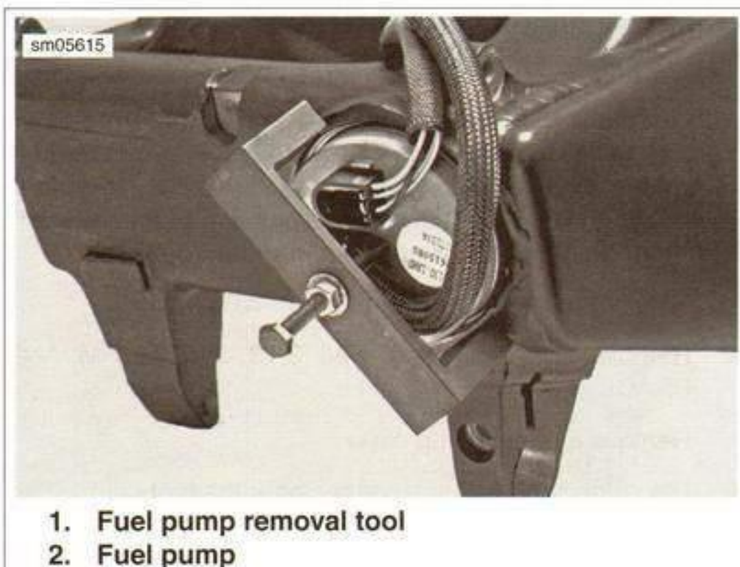
Figure 4-72. Fuel Pump Removal
