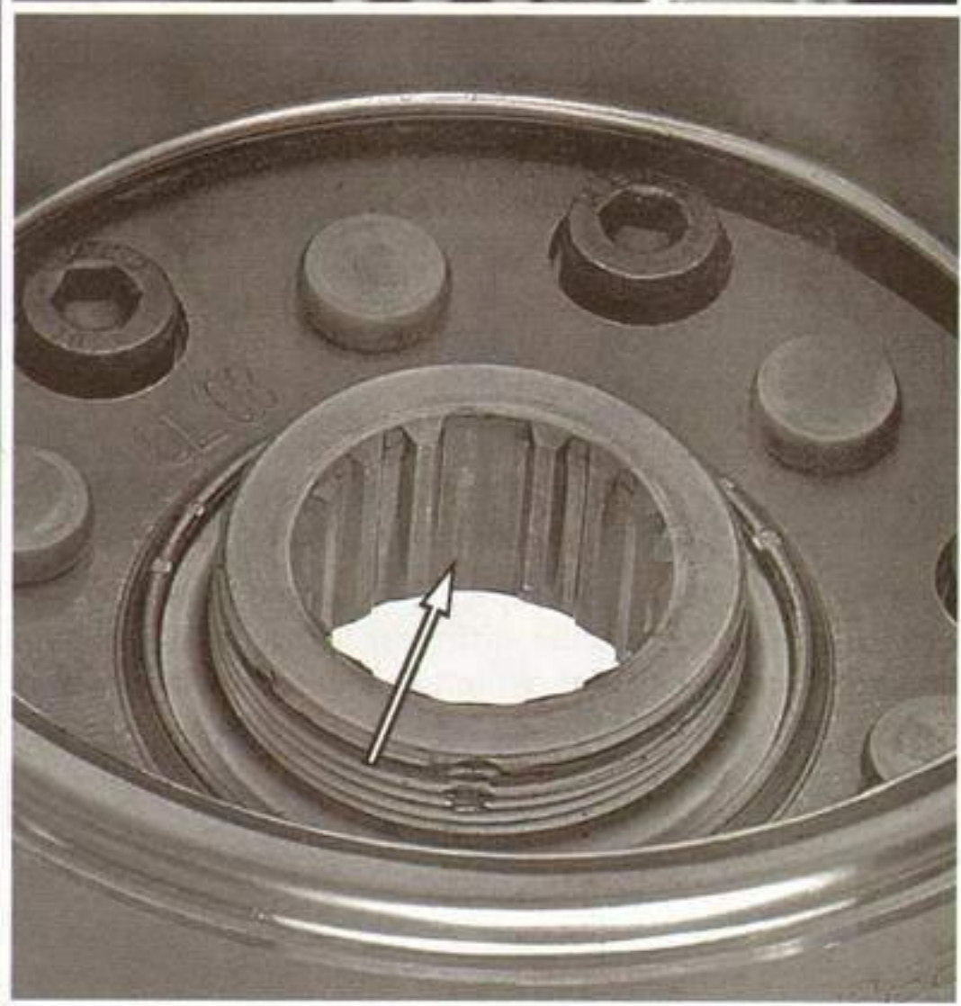
Figure 7-38. Crankshaft Spline Double Tooth and Gap in Splines in Rotor
