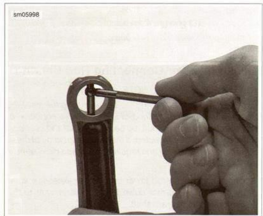
Figure 3-97. Connecting Rod Piston Pin Bore Measurement
