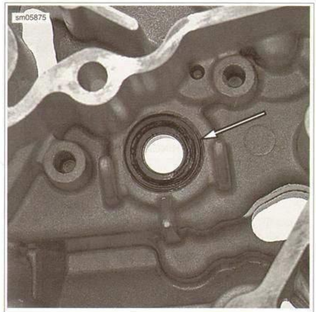
Figure 6-86. Right Case Seal (inner)
