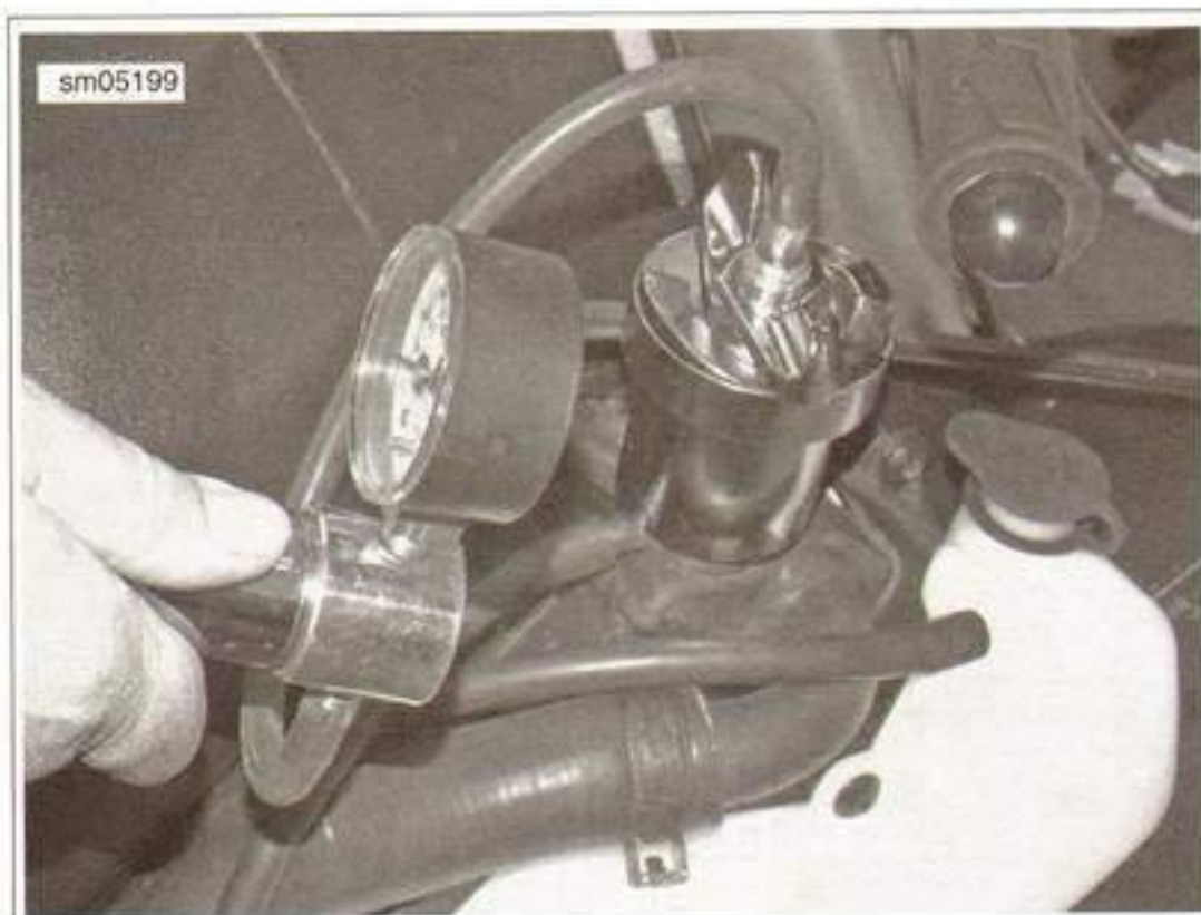
Figure 5-5. System Pressure Test
