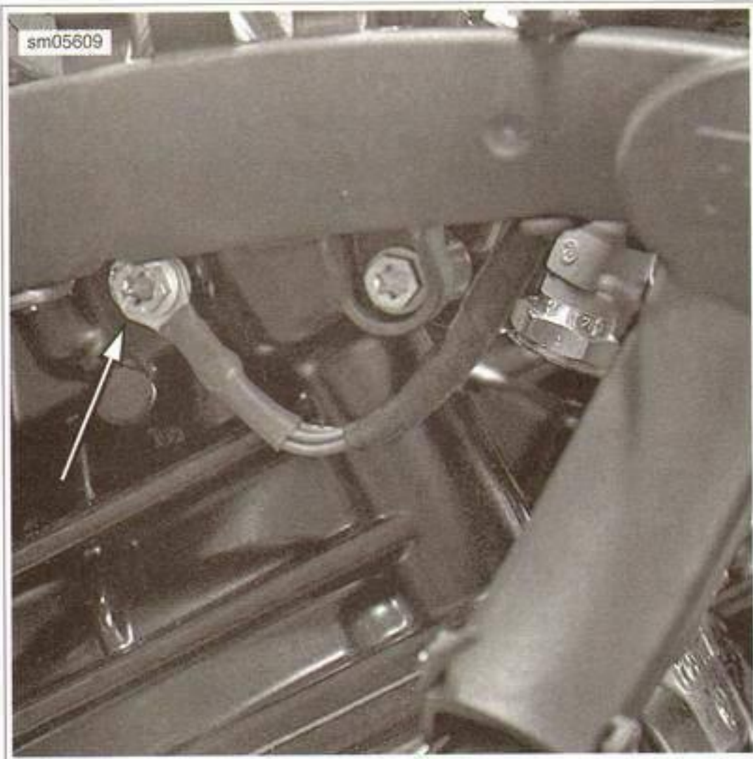
Figure 7-108. Engine Ground Connection
