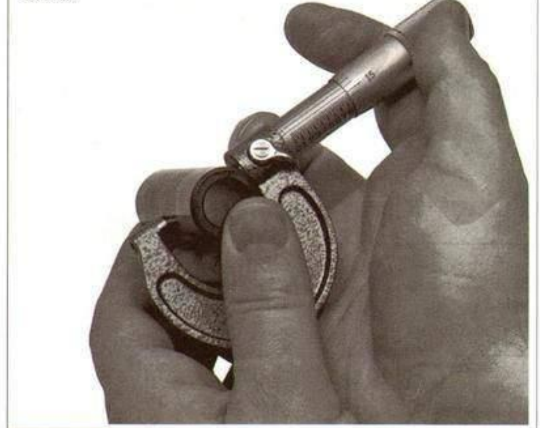
Figure 3-96. Piston Pin Diameter Measurement
