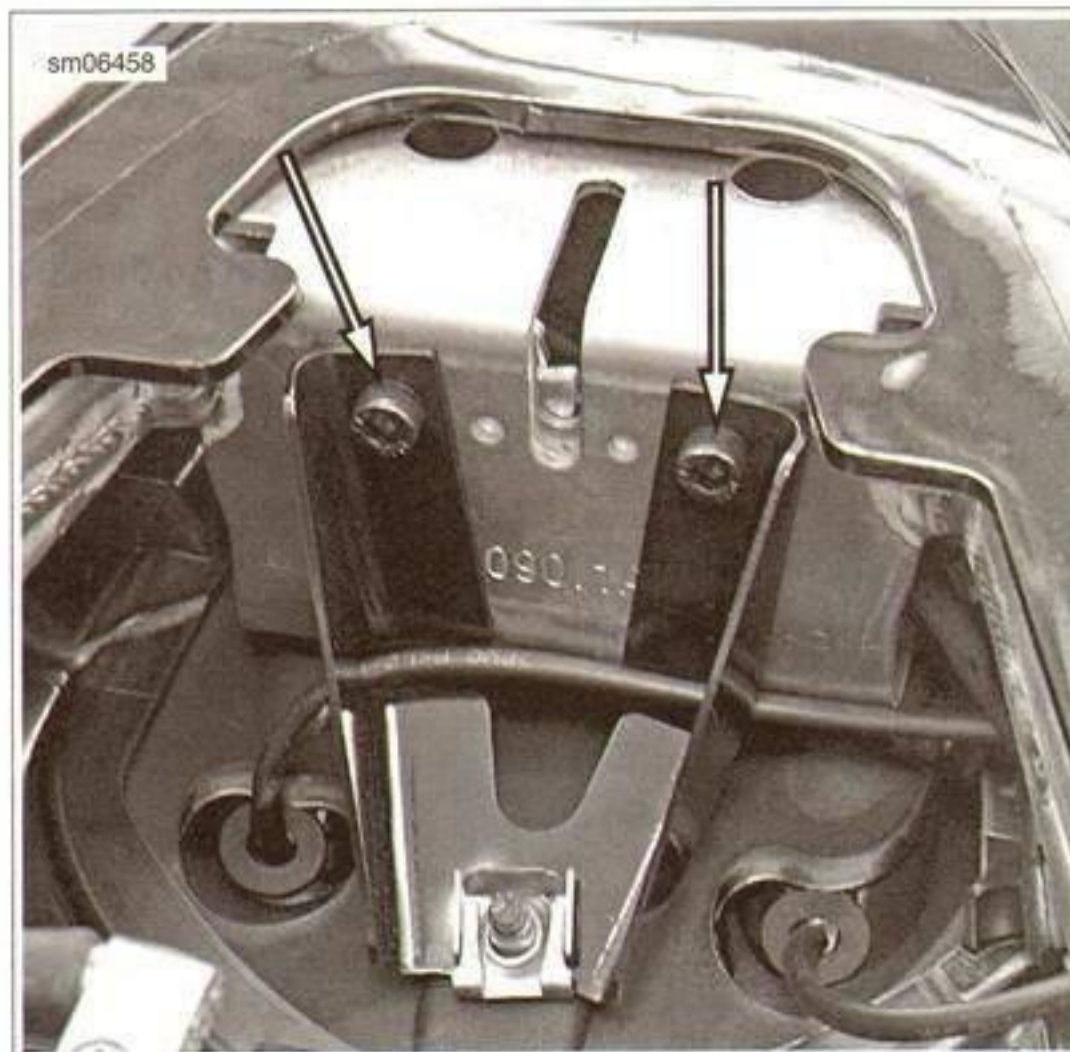
Figure 2-121. Pillion Latch Fasteners
