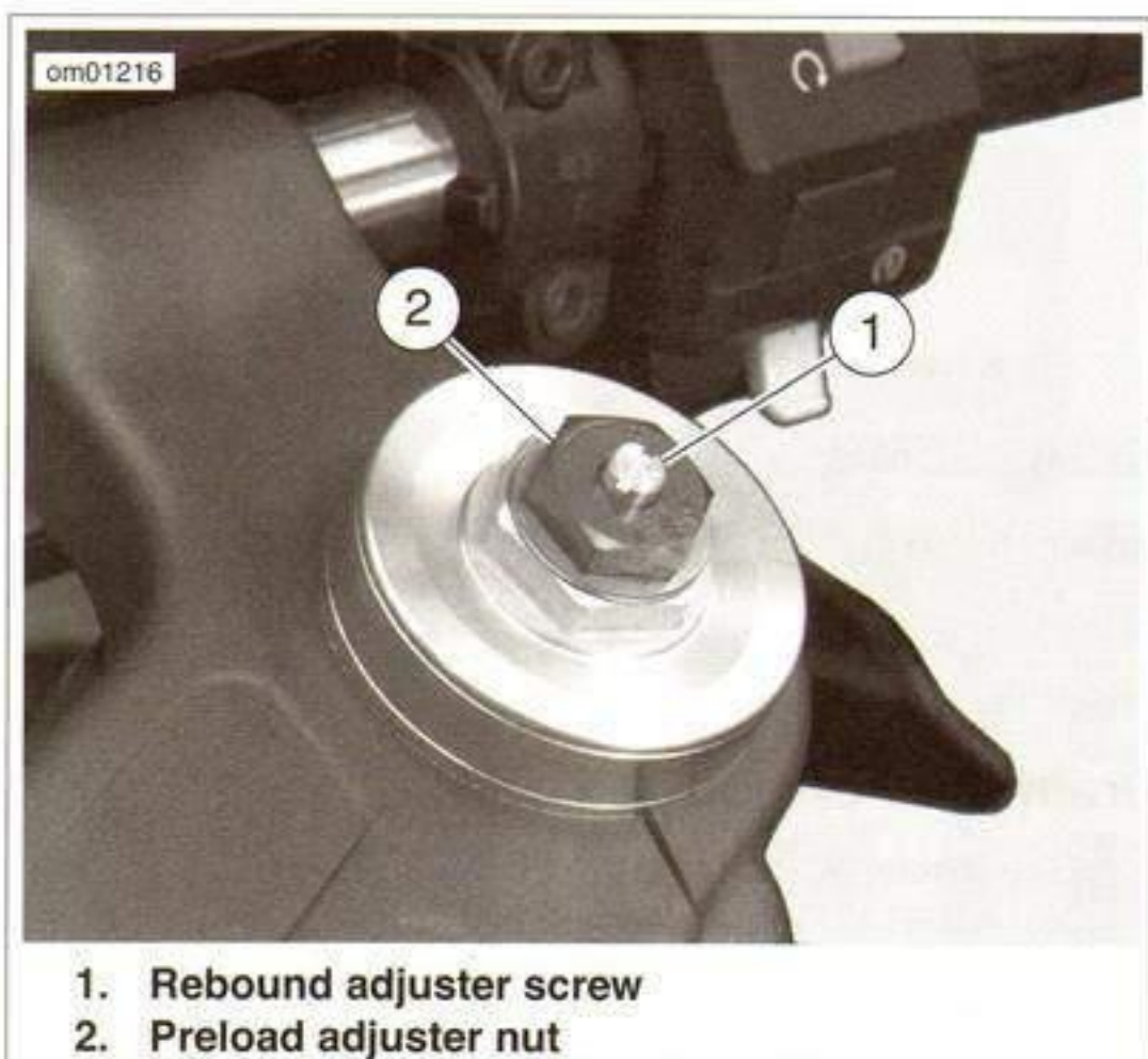
Figure 2-83. Front Fork Preload and Rebound Adjuster
