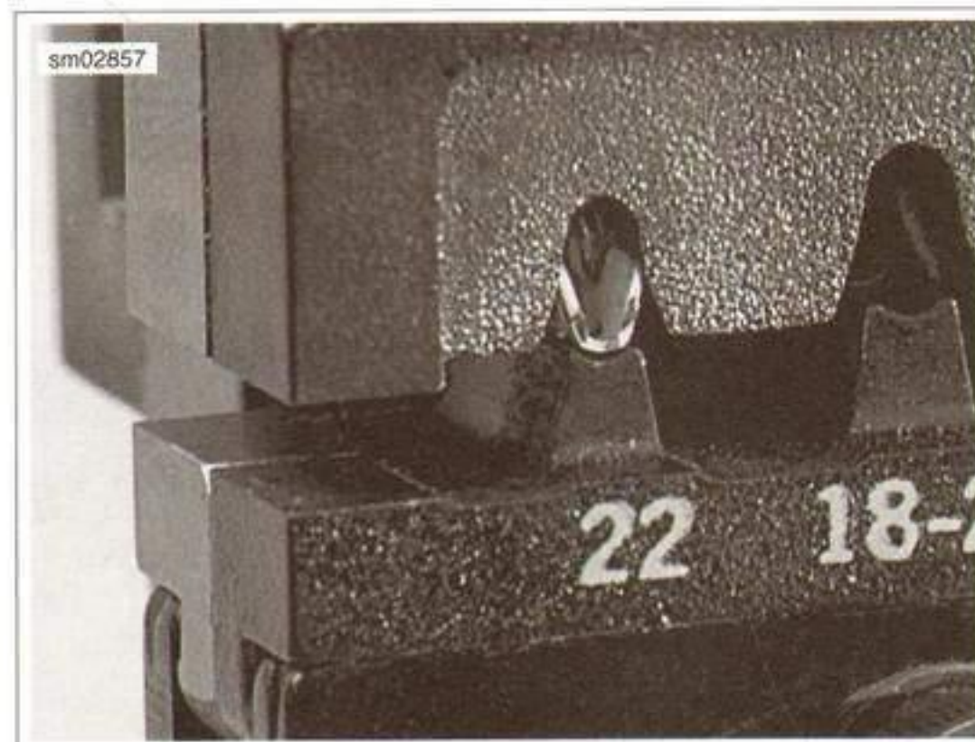
Figure A-34. Crimp Tails in Vertical Alignment between Punch and Die
