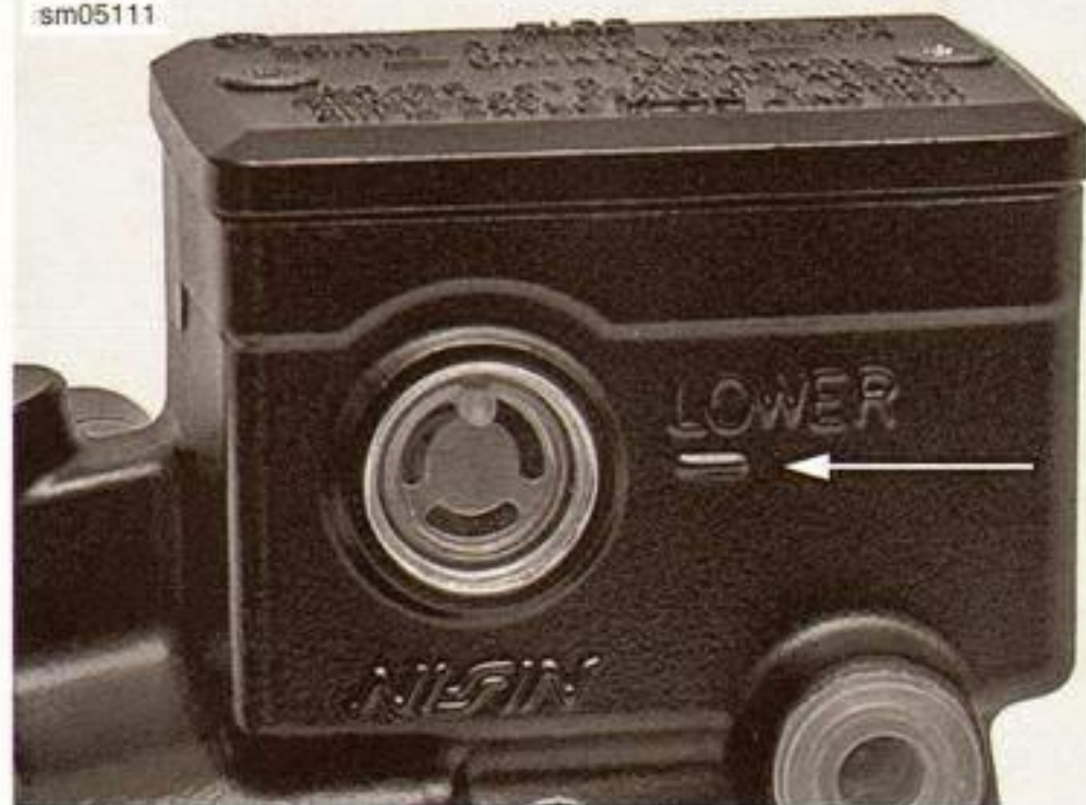
Figure 1-19. Brake Fluid Reservoir LOWER Line
