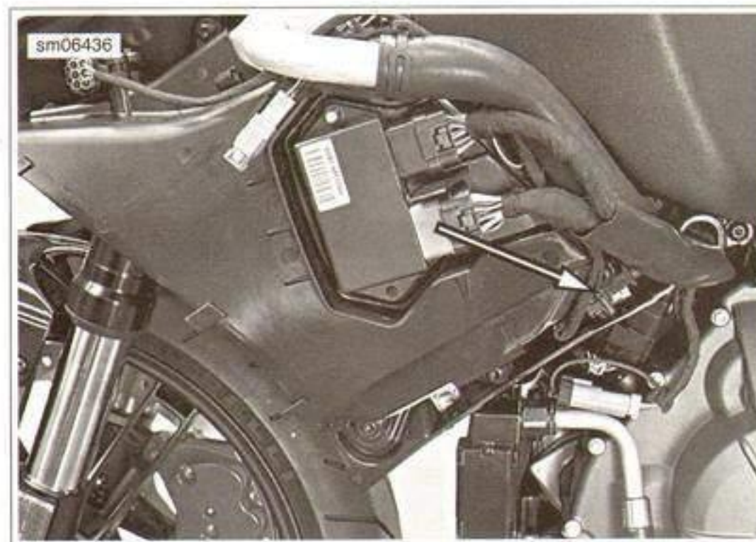
Figure 7-92. CKP Sensor Connector [79]
