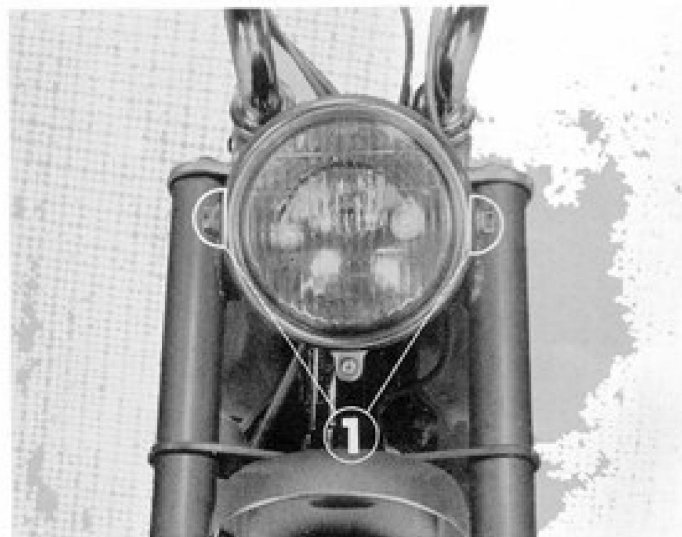
① Headlight mounting bolts
