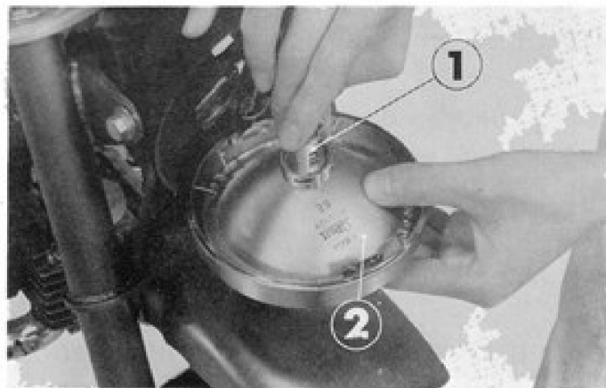
① Headlight socket ② Reflector
