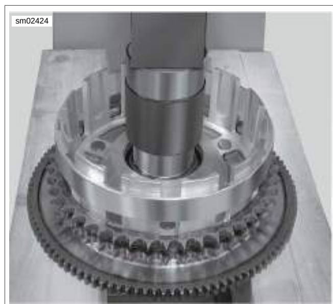
Figure 5-35. Pressing Bearing From Clutch Shell
