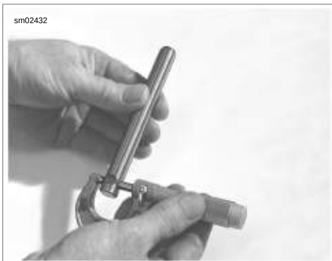
Figure 3-71. Checking Shaft to Support Plate Fit
