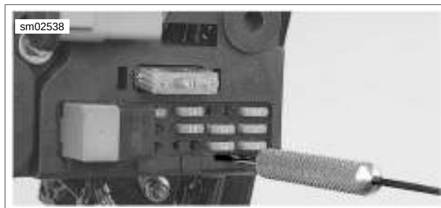
Figure 7-2. Removing Relay/Fuse Panels
