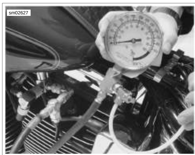
Figure 4-59. Fuel Pressure Gauge Installed (Typical)
