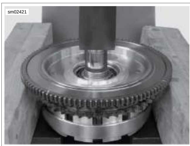
Figure 5-33. Pressing Clutch Hub From Bearing
