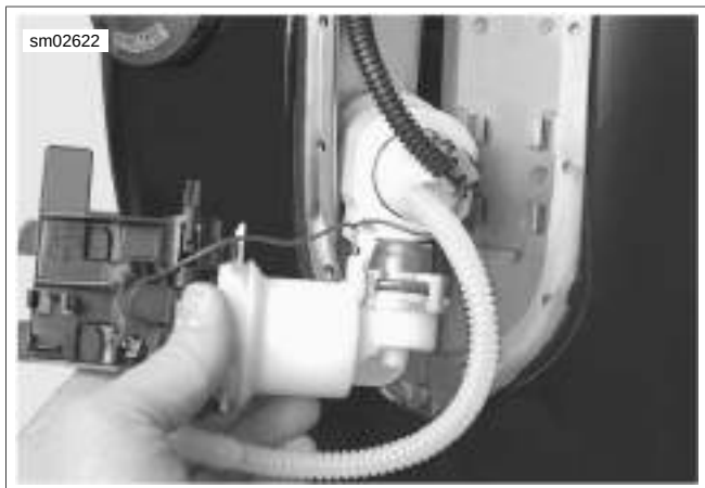
Figure 4-49. Fuel Pump Installation
