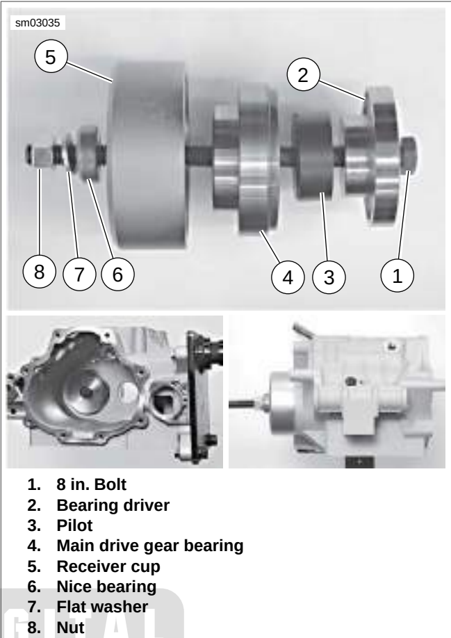
Figure 6-36. Removing Main Drive Gear Bearing
