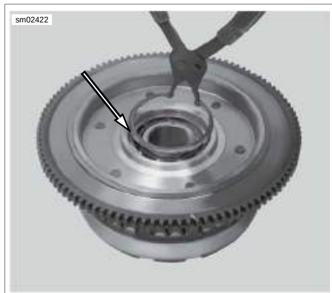
Figure 5-34. Install Clutch Shell Retaining Ring with Flat Side Against Bearing
