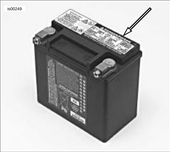
Figure 1-37. AGM Battery with Warning Label
