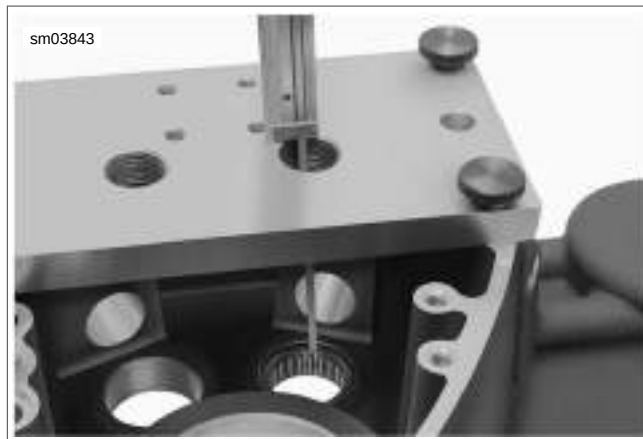
Figure 3-120. Measure from Top of Support Plate to Edge of Needle Bearing
