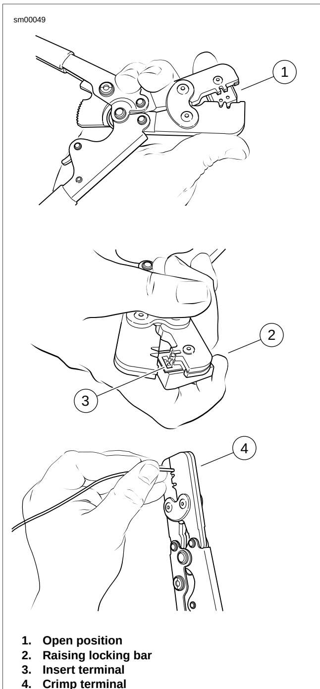
Figure A-51. Packard Micro 64 Connector: Terminal in Crimper
