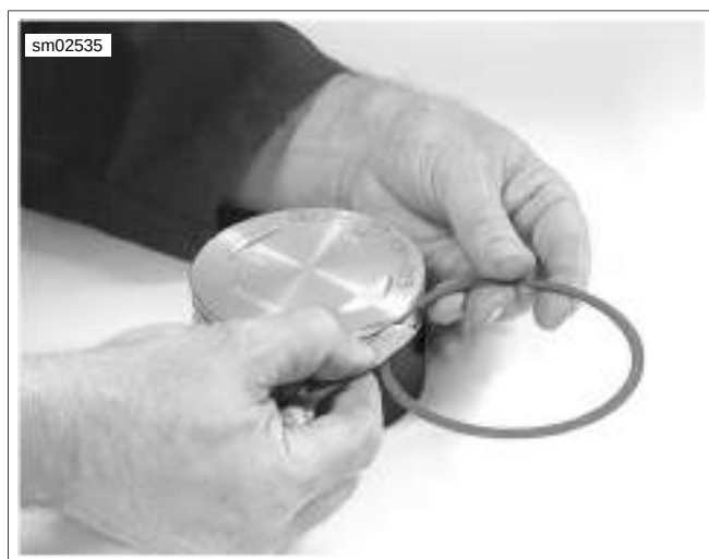
Figure 3-102. Measure Piston Ring Side Clearance
