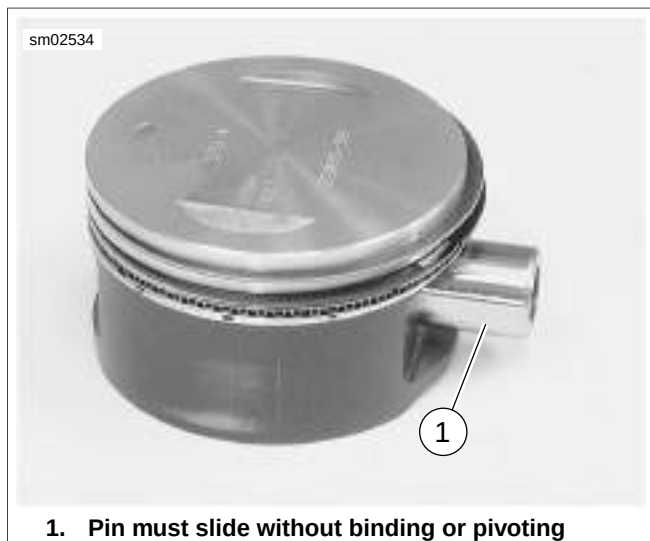
Figure 3-101. Piston Pin Clearance
