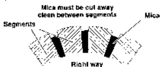
Figure 5-15. Undercutting Mica Separators
