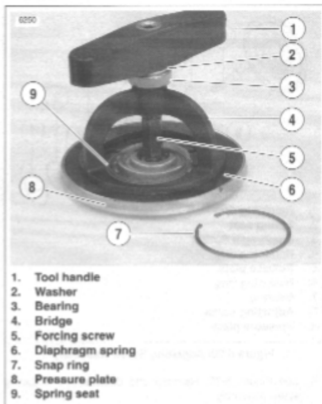
Figure 6-19. Pressure Plate Assembly
