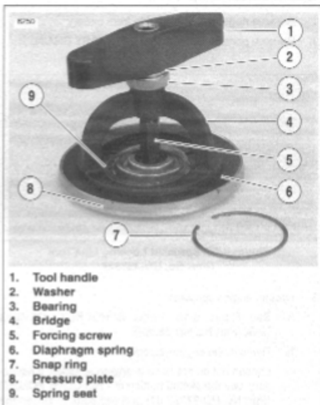
Figure 6-14. Pressure Plate Assembly
