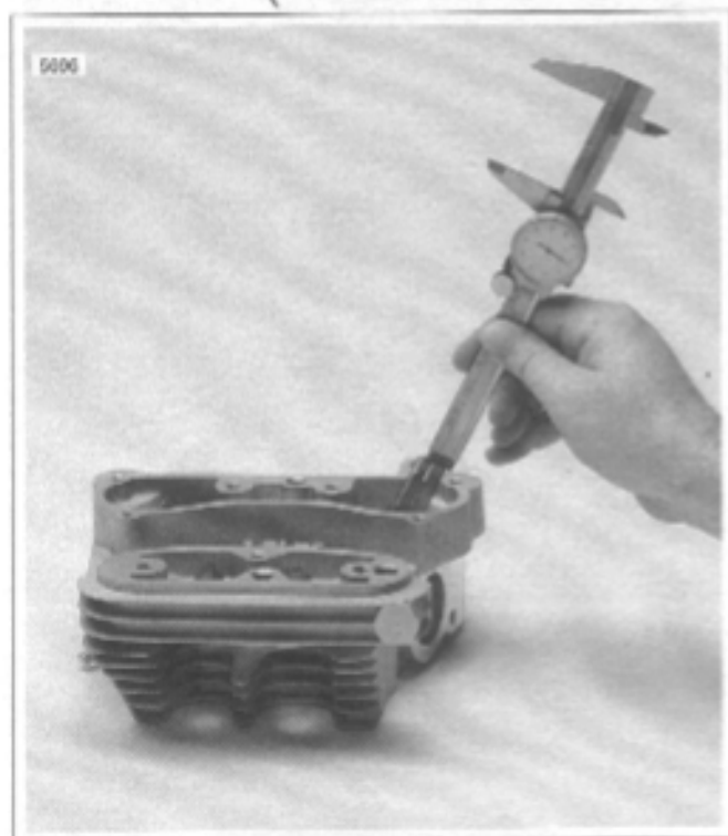
Figure 3-73. Measuring Valve Stem Protrusion
