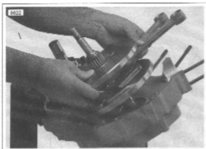
Figure 3-136. Removing Flywheels from Left Crankcase
