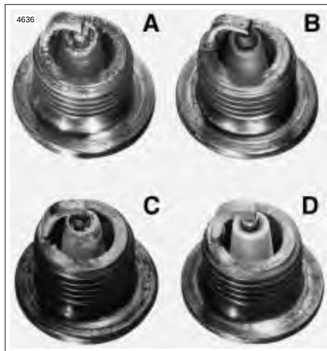
Figure 1-40. Typical Spark Plug Deposits
