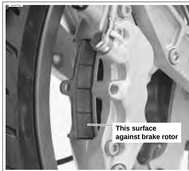
Figure 2-29. Installing Brake Pads
