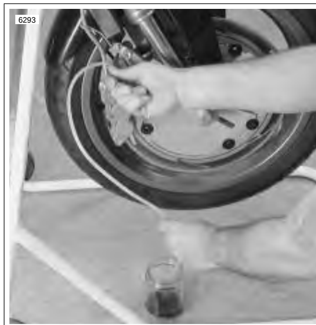
Figure 2-17. Draining Front Brake System (Typical)
