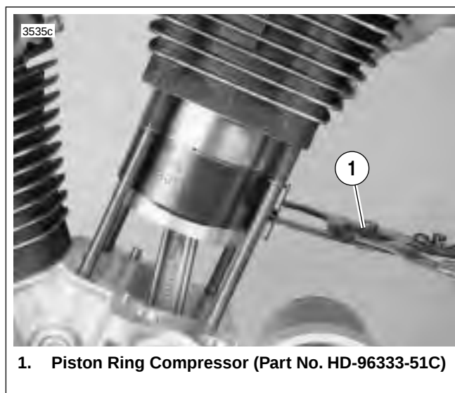
Figure 3-42. Compressing Piston Rings
