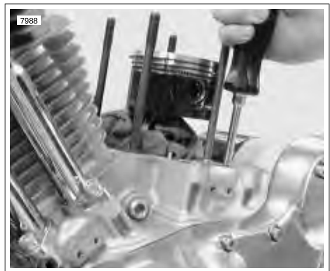
Figure 3-71. Checking Cam Gear End Play
