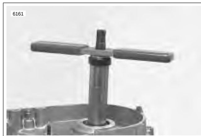
Figure 3-91. Installing Flywheel Spacer and Outer Bearing
