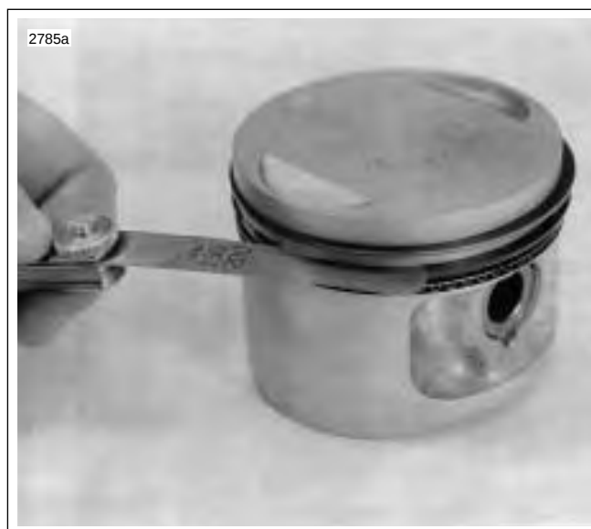
Figure 3-37. Measuring Ring Clearance in Groove
