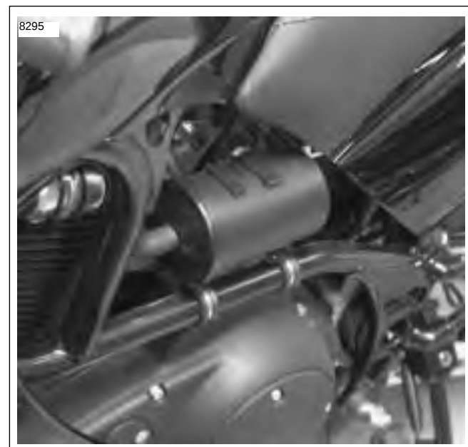
Figure 4-110. Carbon Canister Installed
