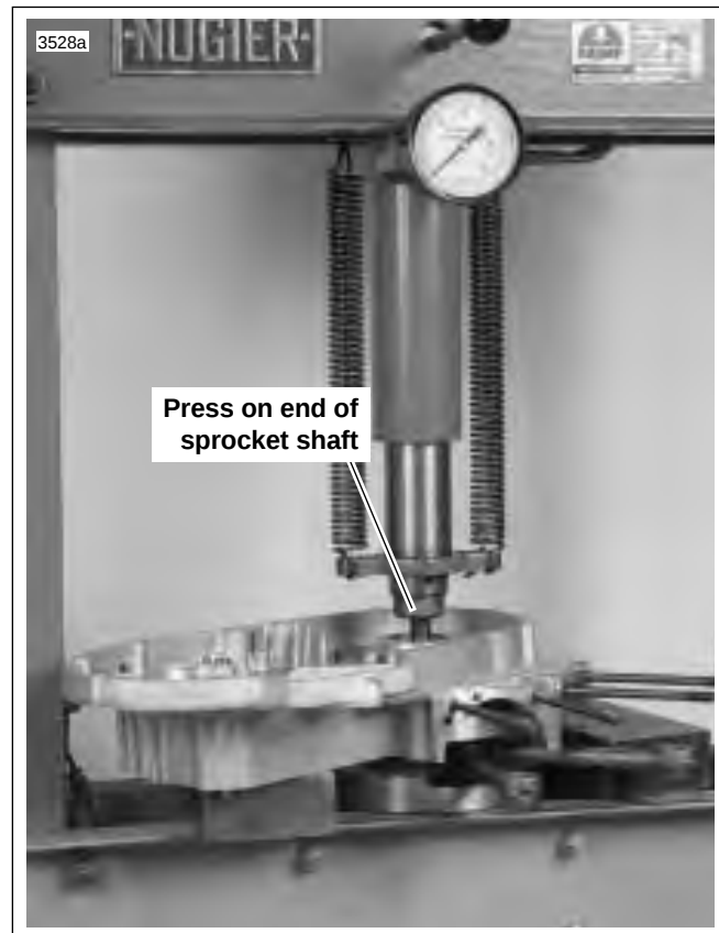
Figure 3-74. Pressing Flywheel from Crankcase
