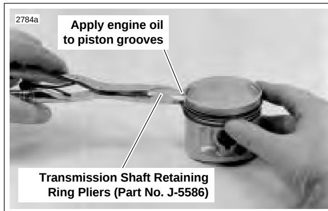
Figure 3-35. Installing Piston Rings
