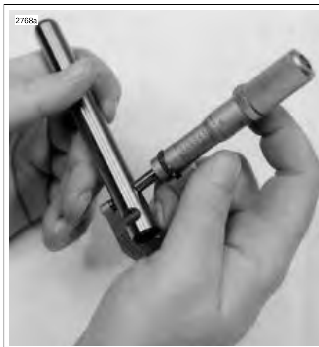
Figure 3-13. Measuring Rocker Arm Shaft Diameter (Rocker Arm Bushing Position)
