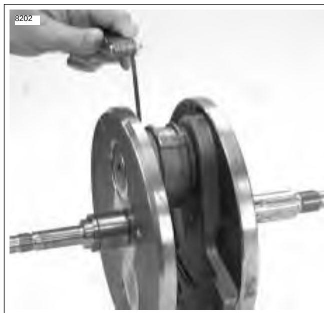
Figure 3-80. Checking Connecting Rod Side Play
