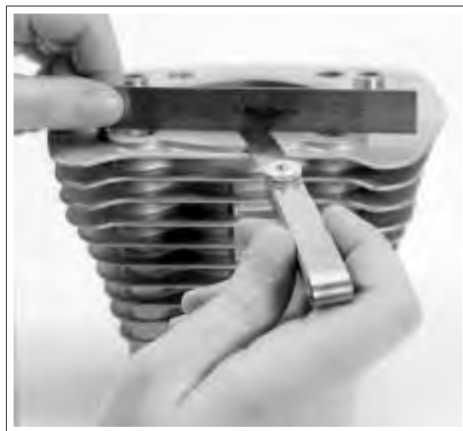
Figure 3-31. Checking Gasket Surfaces
