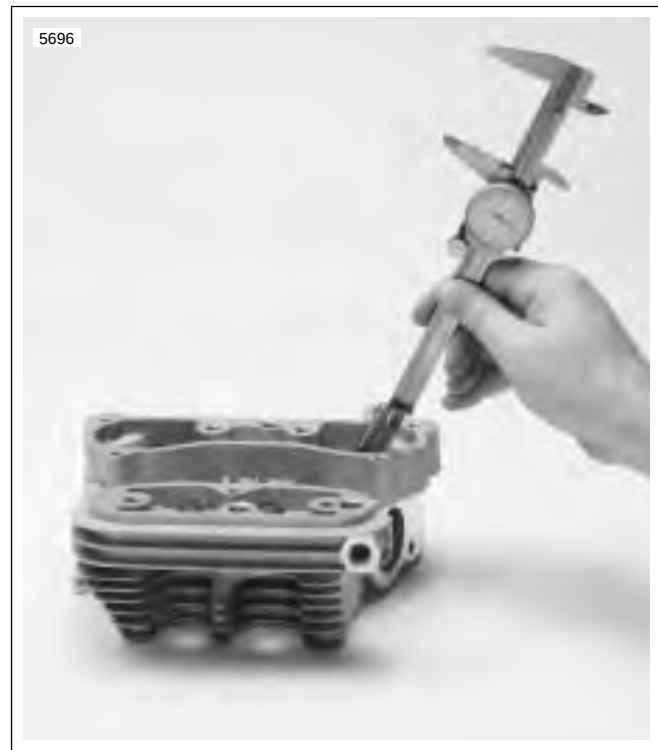
Figure 3-23. Measuring Valve Stem Protrusion
