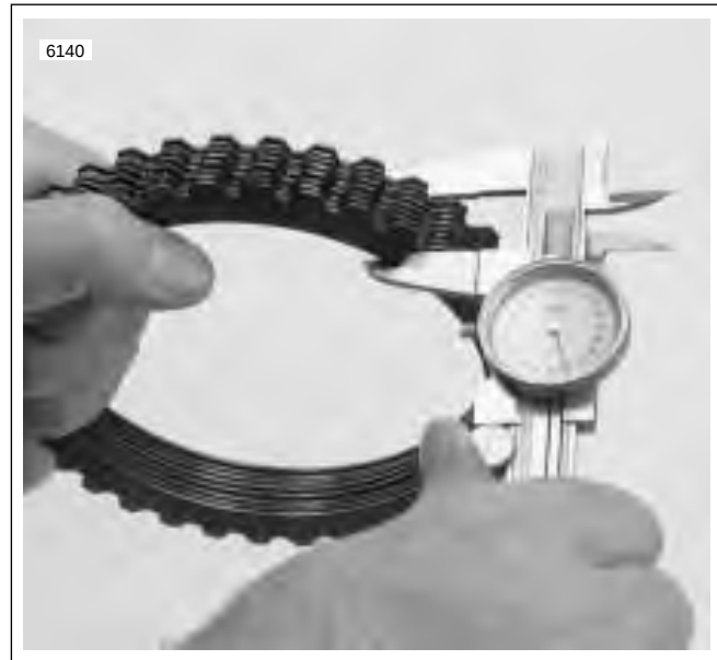
Figure 6-19. Measuring Friction Plates
