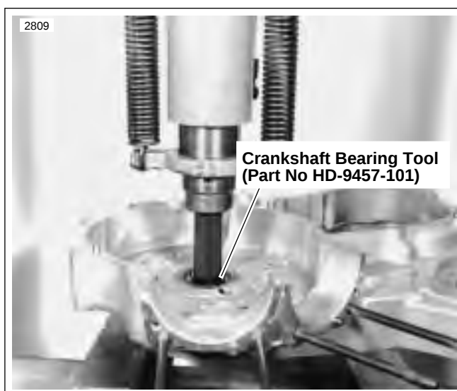
Figure 3-77. Sprocket Shaft Outer Race Removal
