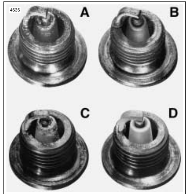
Figure 1-40. Typical Spark Plug Deposits
