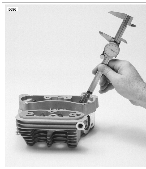
Figure 3-23. Measuring Valve Stem Protrusion
