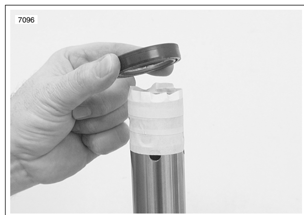
Figure 2-54. Slide Pipe Protection
