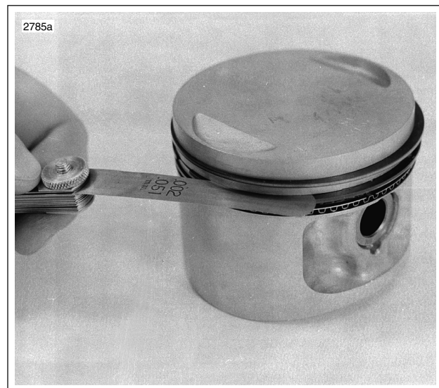
Figure 3-37. Measuring Ring Clearance in Groove
