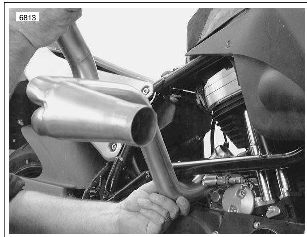
Figure 2-96. Exhaust Header Positioning (Typical)
