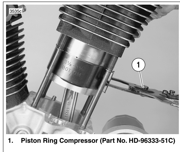
Figure 3-42. Compressing Piston Rings
