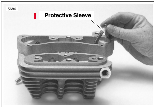
Figure 3-26. Valve Guide Seal Protector Sleeve
