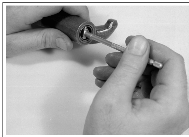
Figure 3-15. Measuring Rocker Arm Bushing Inner Diameter
