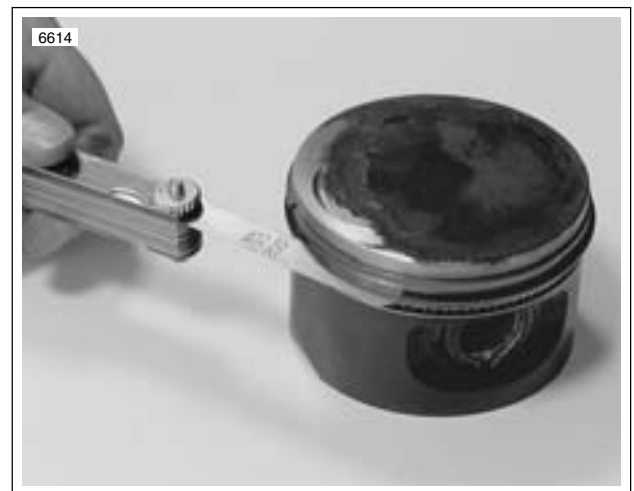
Figure 3-75. Measuring Ring Clearance in Groove
