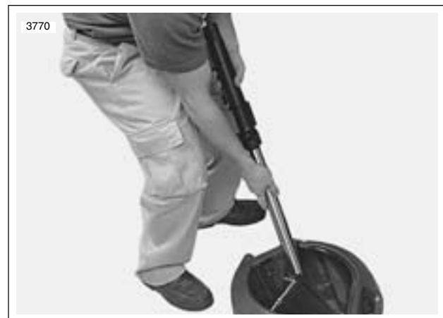
Figure 2-62. Pumping Fork Oil
