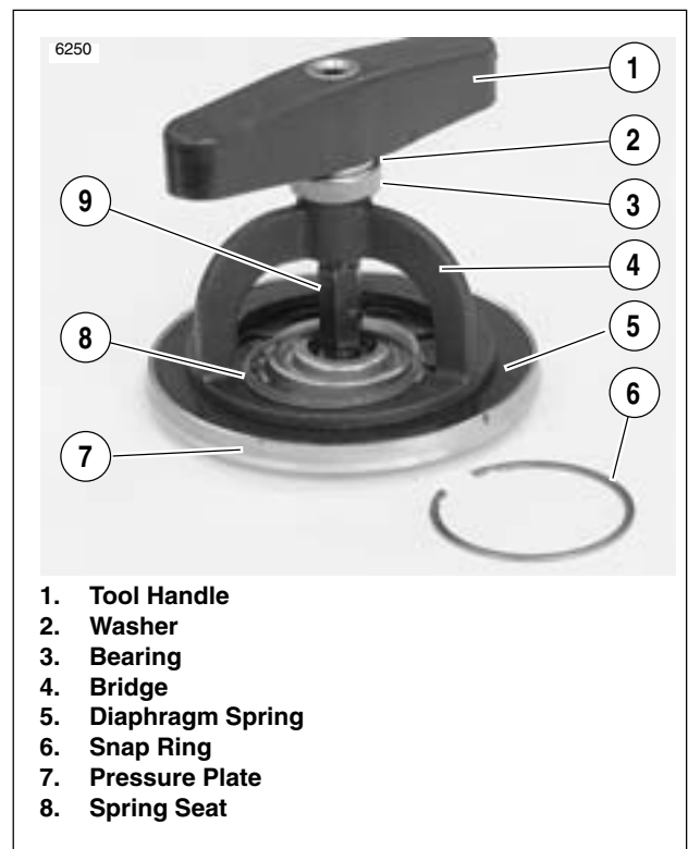
Figure 6-21. Pressure Plate Assembly
