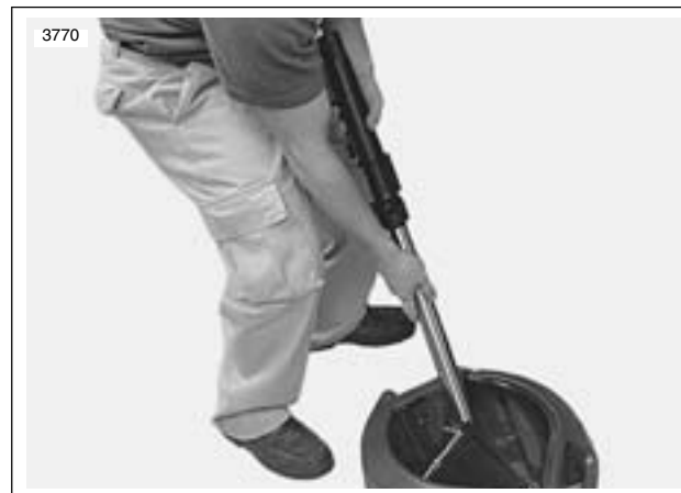
Figure 1-29. Pumping Fork Oil
