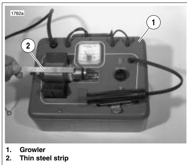
Figure 5-20. Shorted Armature Test Using Growler
