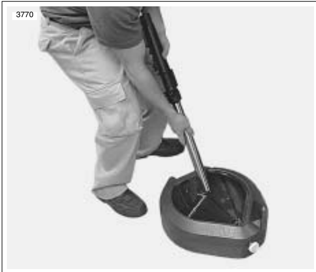
Figure 1-30. Pumping Fork Oil
