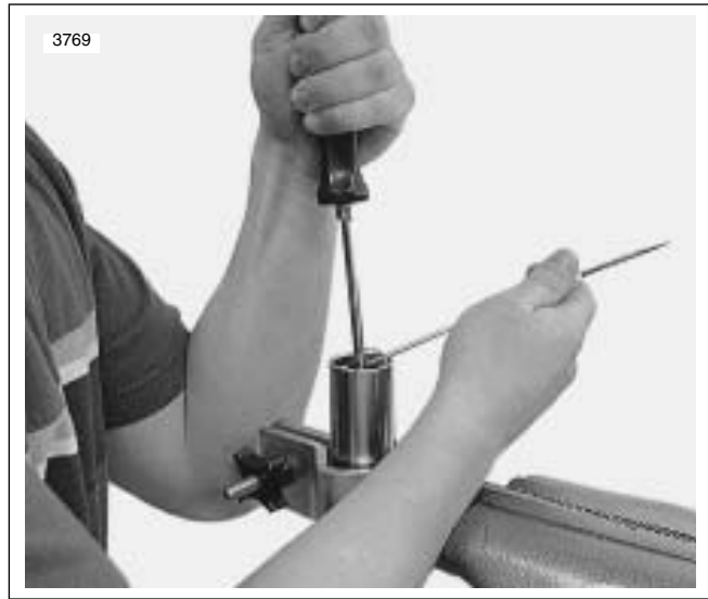
Figure 2-93. Compressing Spring Seat to Install Stopper Ring
