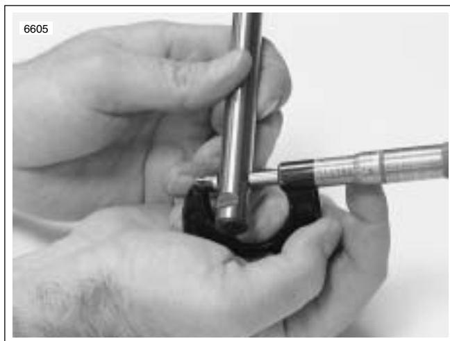
Figure 3-52. Measuring Rocker Arm Shaft Diameter (Rocker Arm Bushing Position)
