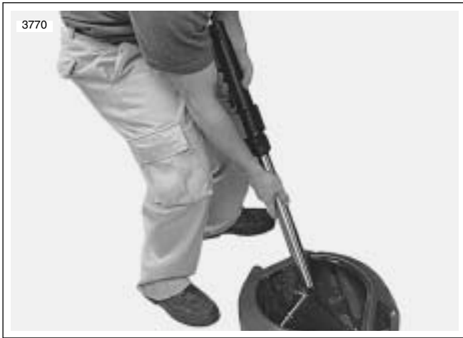
Figure 2-71. Pumping Fork Oil
