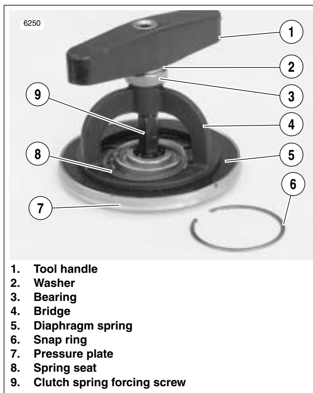
Figure 6-13. Pressure Plate Assembly
