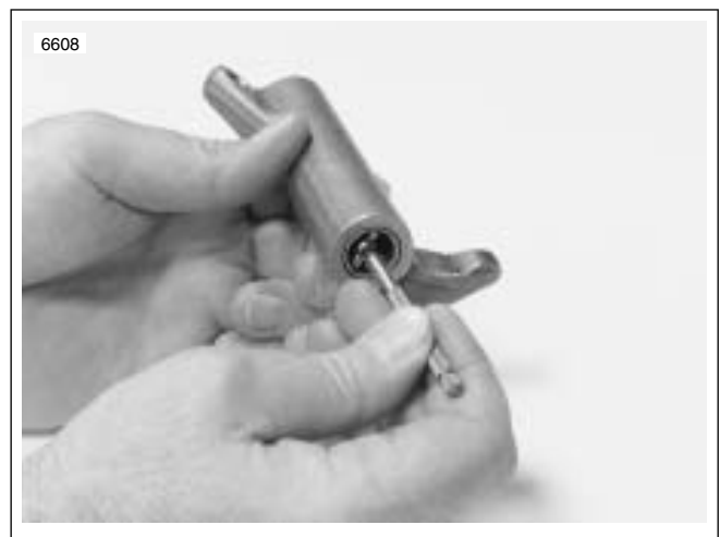
Figure 3-54. Measuring Rocker Arm Bushing Inner Diameter
