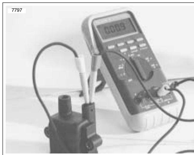
Figure 7-25. Ignition Coil Primary Resistance Test
