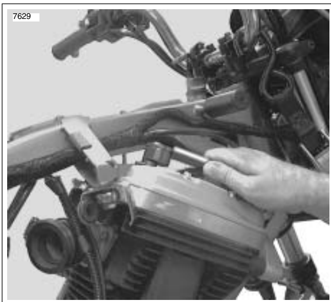
Figure 3-1. Remove Crankcase Breather Hose
