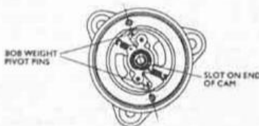
Correct location of timing advance unit
