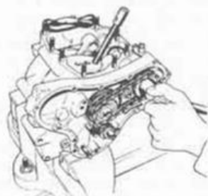
Removing the camshaft sprocket nut
