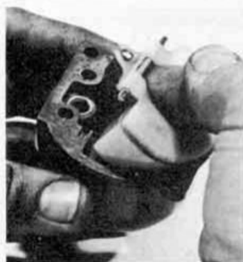
Removing the float, spindle, and float needle
