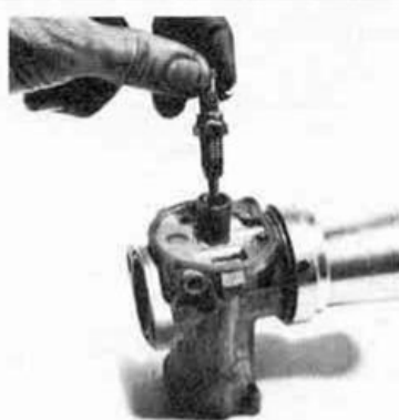
Removing the jet holder complete with main and needle jets
