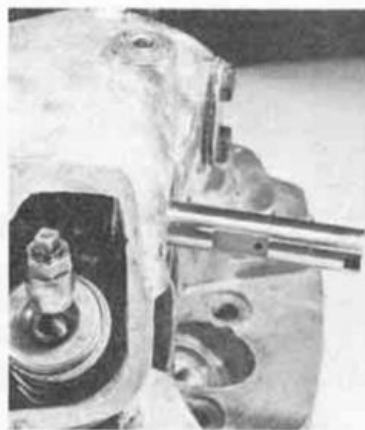
The oil hole in the spindle must face AWAY FROM the center of the head.
