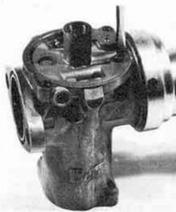
Removing the pilot jet
