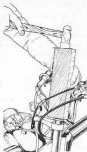
Freeing the fork tube from the upper triple clamp
