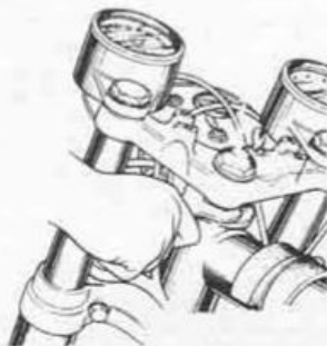
Adjusting the steering head bearings (pre-1971 models)
