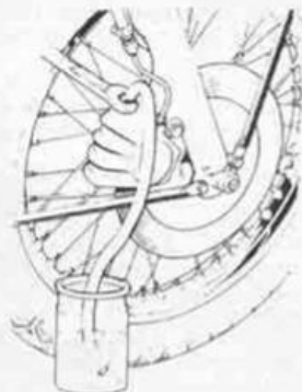
Bleeding the front disc brake
