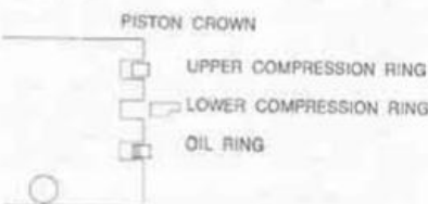
Correct installation of stepped compression ring
