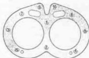
Cylinder head tightening sequence; reverse the order when removing the head
