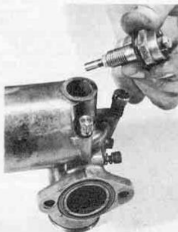
Removing the jet holder and jets
