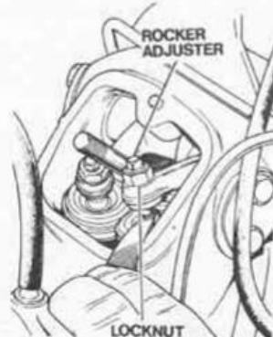
Adjusting the valves
