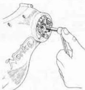
Removing the advance mechanism
