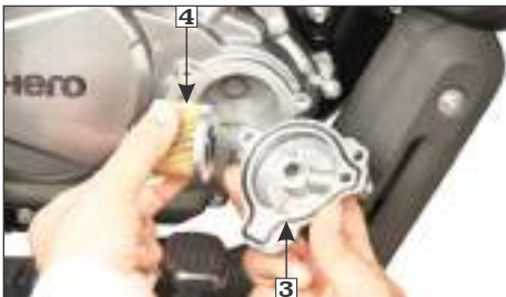
(3) O-ring (4) Engine oil filter element
