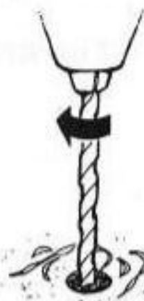
2. Drill hole in stud
