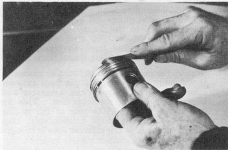
FITTING RINGS TO THE PISTON: Worn rings allow the engine to pump excess oil and may break up in operation. Maximum ring groove clearance due to wear should not be over .008 or .010. The proper clearance should be .002 to .003 and rings should not bind in the grooves.
