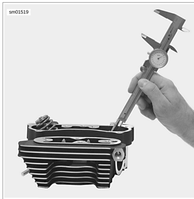
Figure 3-120. Measuring Valve Stem Protrusion
