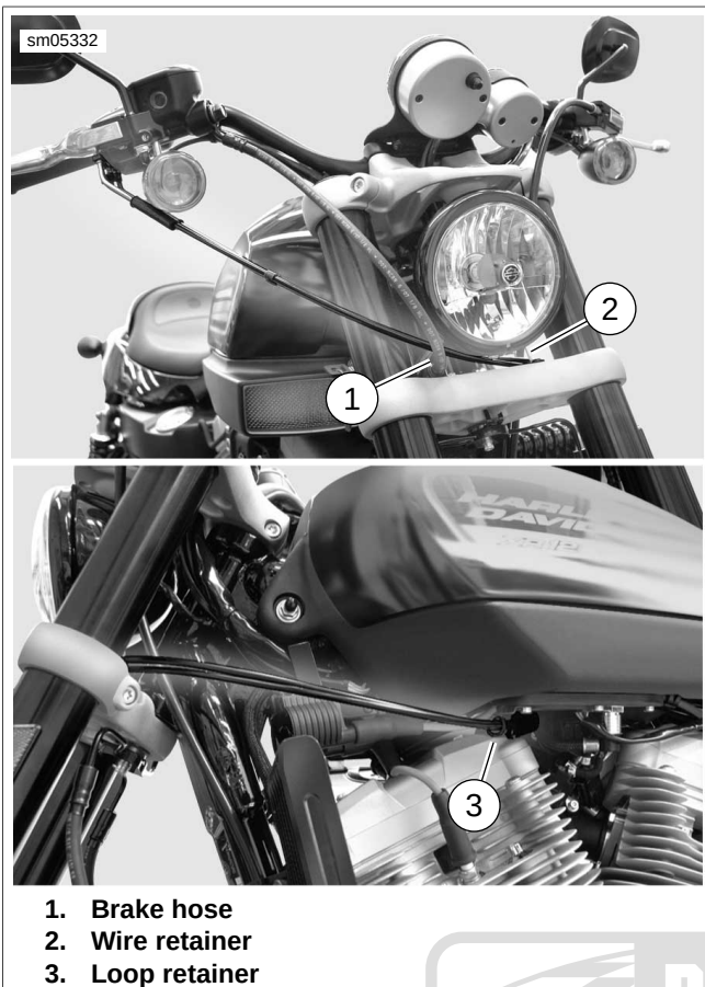
Figure 2-219. Throttle Control Cable Routing: XR Models
