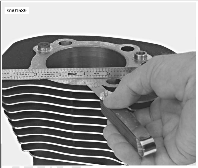
Figure 3-136. Checking Gasket Surfaces
