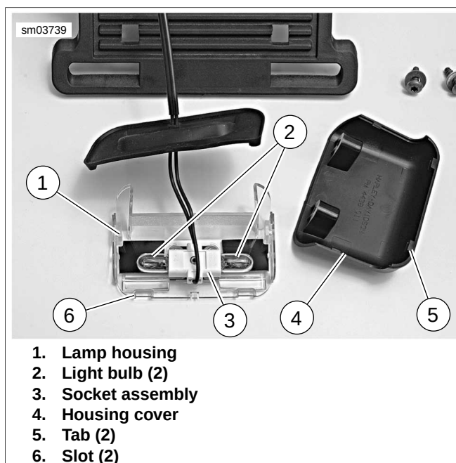
Figure 6-90. Replacing License Plate Light Bulbs: XL 1200N (HDI)
