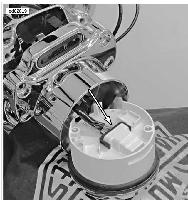
Figure 2-12. Speedometer Connector [39] on XL or Tachometer Connector [108] on XR (Typical)
