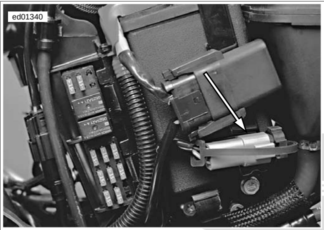
Figure 2-24. Data Link Connector [91A] (Behind Left Side Cover)
