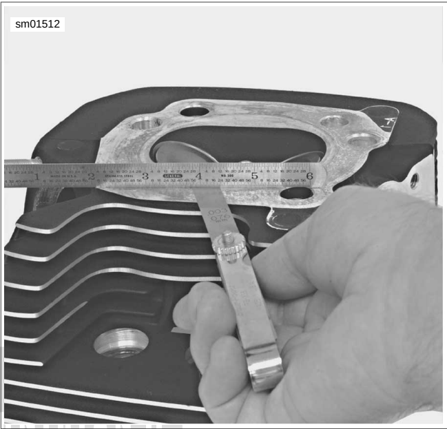
Figure 3-115. Checking Gasket Surface: Must Be Flat Within 0.006 in. (0.152 mm)
