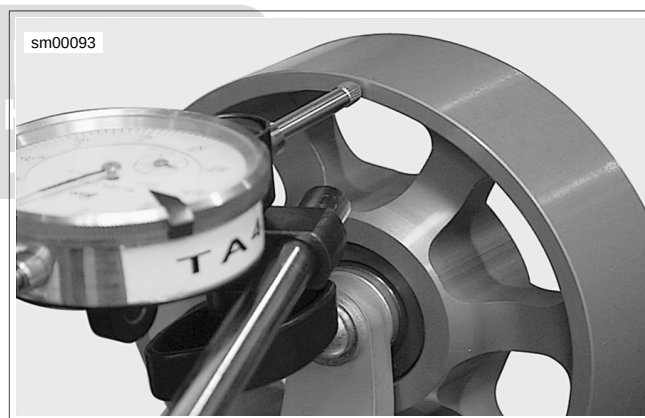
Figure 1-51. Measuring Lateral Side Play on Idler Pulley
