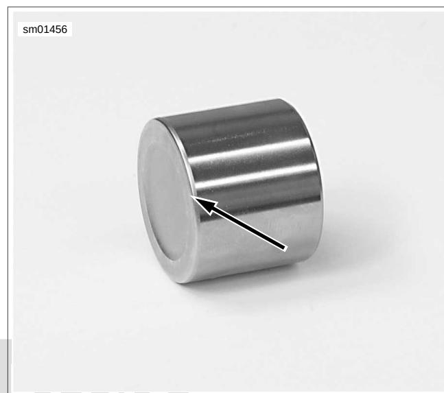
Figure 2-128. Piston Nose Radius
