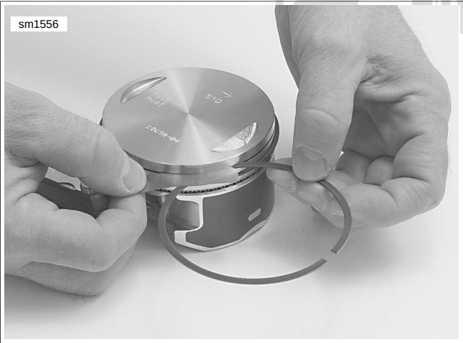
Figure 3-145. Measuring Ring Clearance in Groove (typical; XL model shown)
