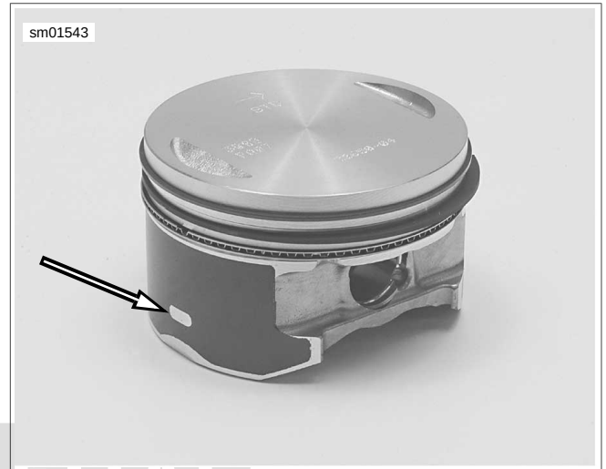
Figure 3-138. Measurement Area (typical; XL model shown)
