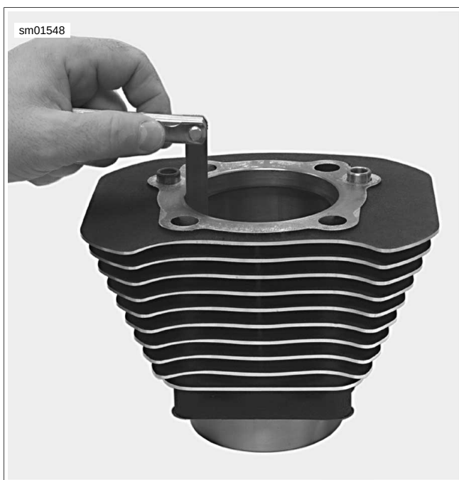
Figure 3-141. Measuring Ring End Gap
