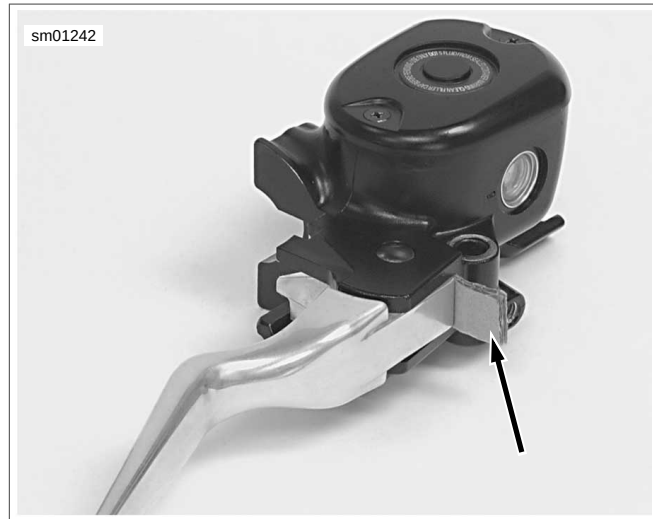
Figure 2-74. Install 5/32 in. (4 mm) Cardboard Insert Before Installing Master Cylinder Assembly
