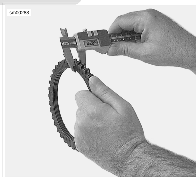
Figure 5-24. Measuring Friction Plates
