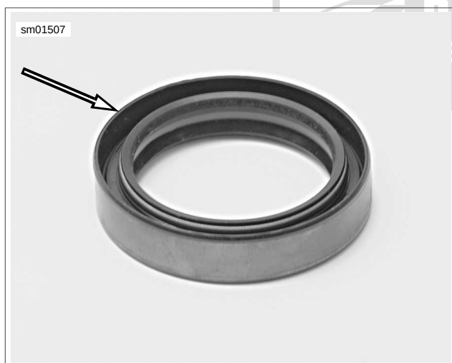
Figure 3-87. Open (Lipped) Side of Seal Faces Out
