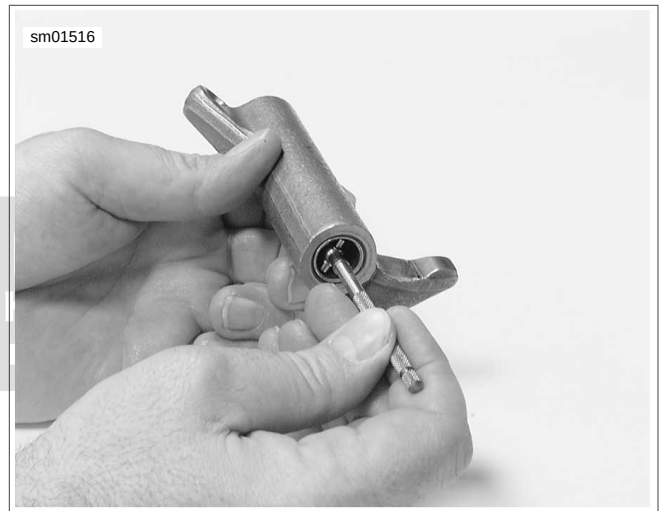
Figure 3-118. Measuring Rocker Arm Bushing Inner Diameter
