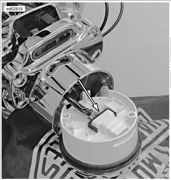
Figure 2-16. Speedometer Connector [39] on XL or Tachometer [108] on XR (Typical)
