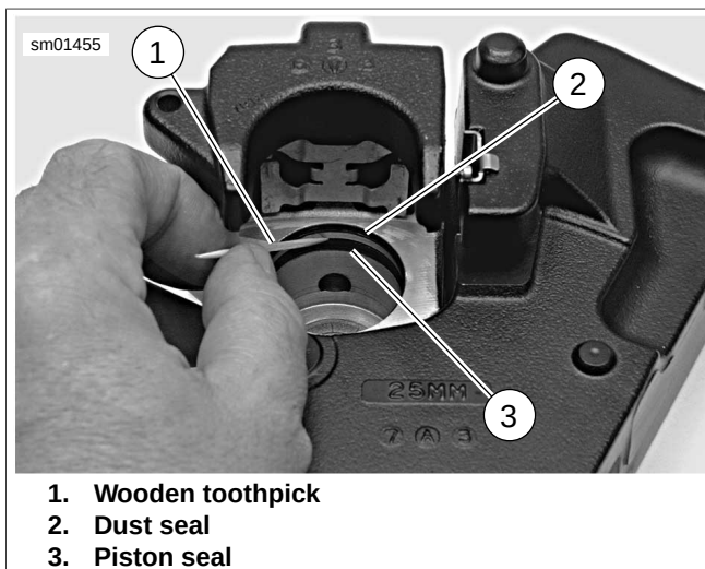
Figure 2-125. Caliper Seals
