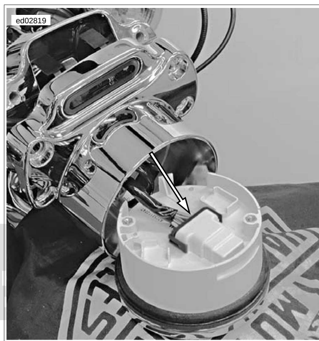
Figure 4-62. Speedometer Connector [39] on XL, and tachometer connector [108A] on XR (Typical)
