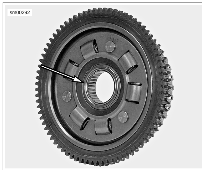
Figure 5-29. New Needle Bearing in Clutch Shell
