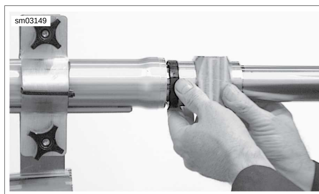
Figure 2-185. Install Bushing, Spacer, and Install Fork Seal in Place with Seal Driver
