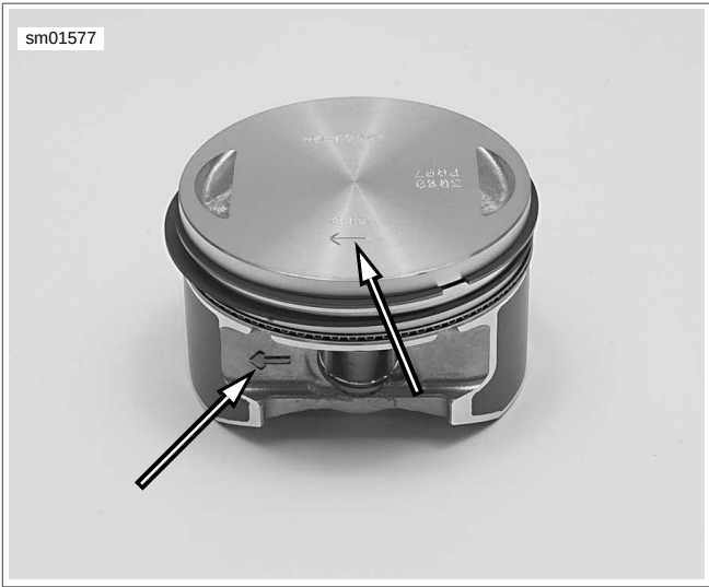
Figure 3-54. Arrows on Piston Must Point Toward Front of Engine (typical; XL shown)
