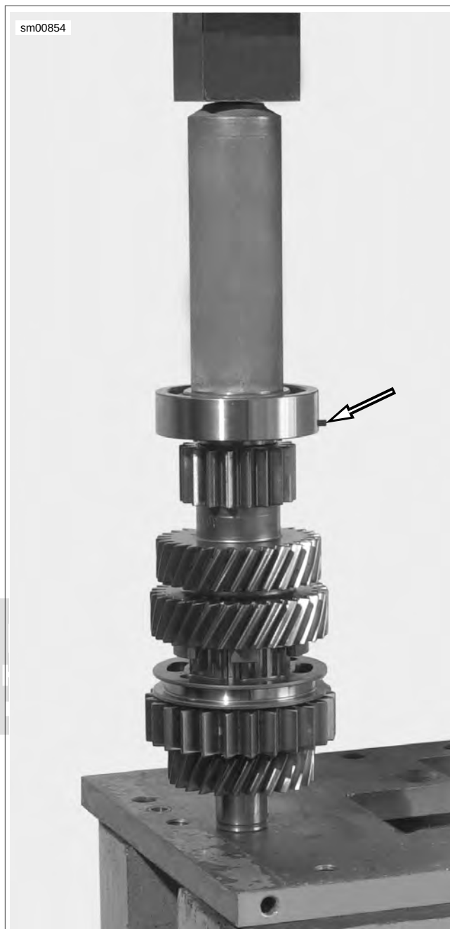
Figure 6-153. 1st Gear Bearing Replacement
