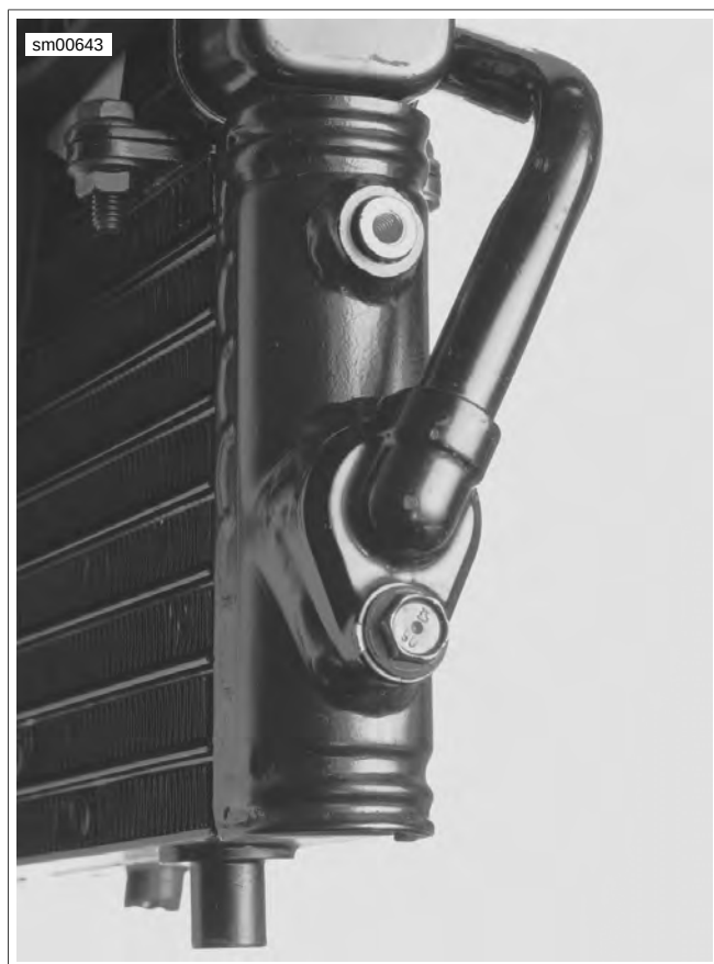
Figure 5-24. Oil Line Manifold
