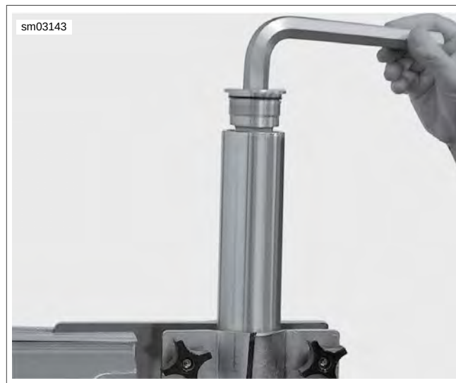
Figure 2-93. Clamp Fork and Loosen Fork Cap
