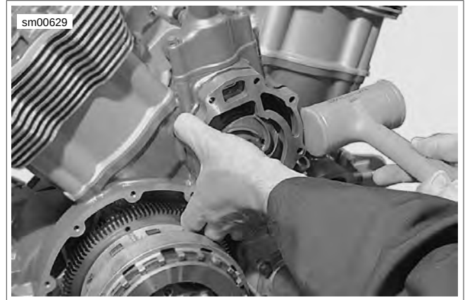
Figure 5-12. Removing Water Pump (clutch cover removed for clarity)
