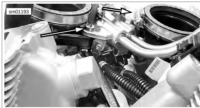
Figure 4-6. Fuel Rail/intake Seal Fasteners (typical)
