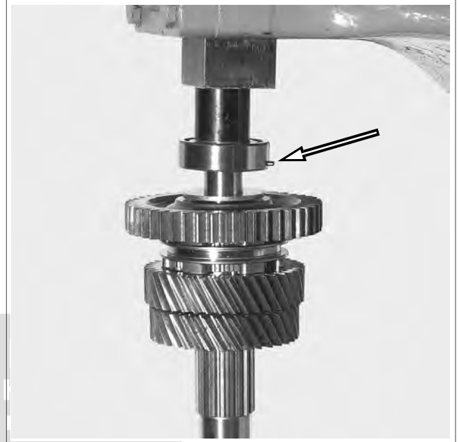
Figure 6-120. 1st Gear Bearing Installation
