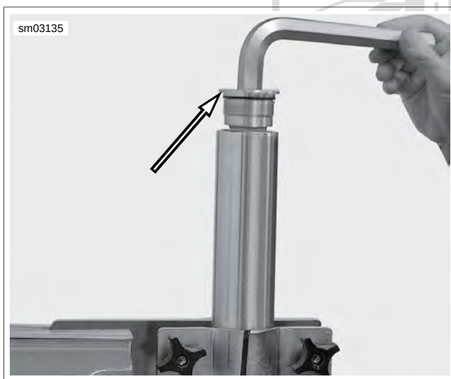
Figure 2-85. Clamp Fork and Remove Fork Cap
