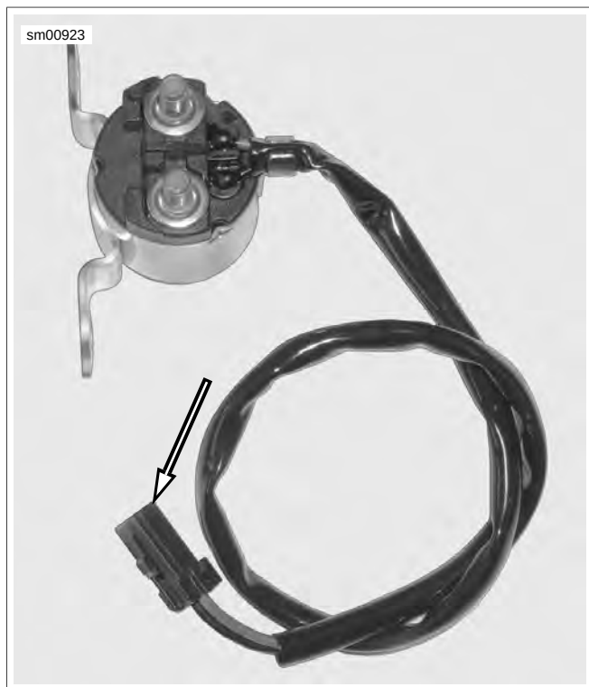
Figure 7-12. Solenoid Paired Black Wire and Green Wire Lead (typical)
