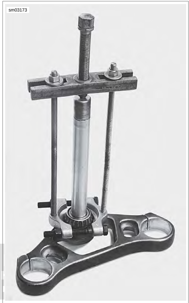
Figure 2-120. Bearing Puller Based on Universal Wedge Attachment (typical)
