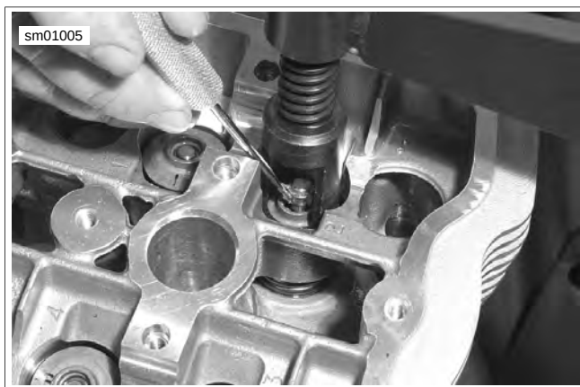
Figure 3-78. Install Valve Keepers
