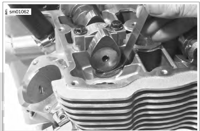
Figure 3-80. Check Valve Lash (typical)
