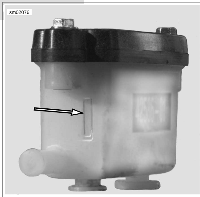
Figure 2-43. Rear Brake Reservoir Sight Glass (removed from motorcycle)
