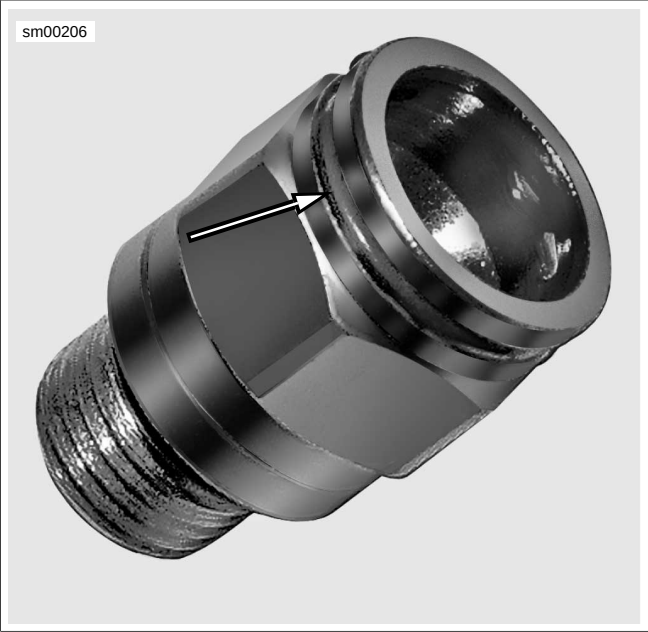
Figure 5-18. Oil Line Fitting with Spring Clip
