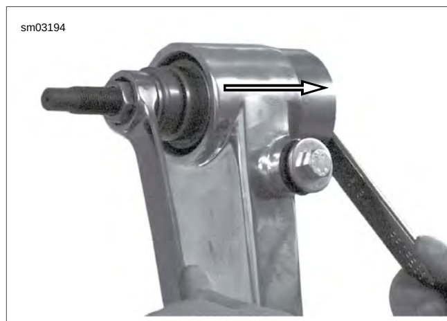
Figure 2-132. Install Left Side Swingarm Bearing (typical)
