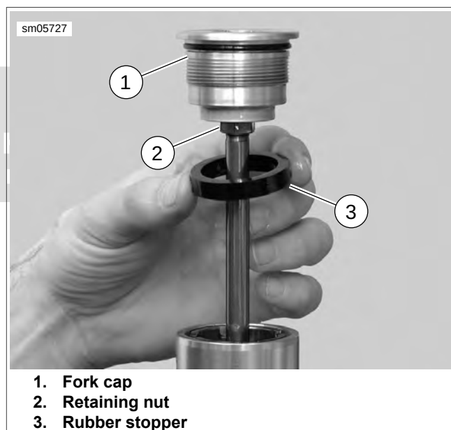
Figure 2-94. Remove Fork Cap, Retaining Nut and Rubber Stopper
