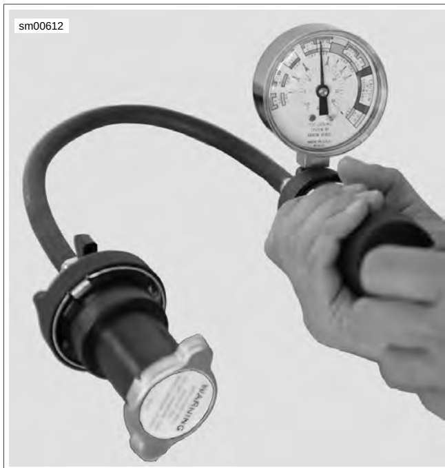
Figure 5-3. Pressure Cap Test
