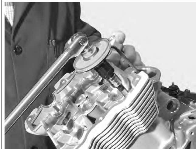
Figure 3-84. Tighten Head Bolts
