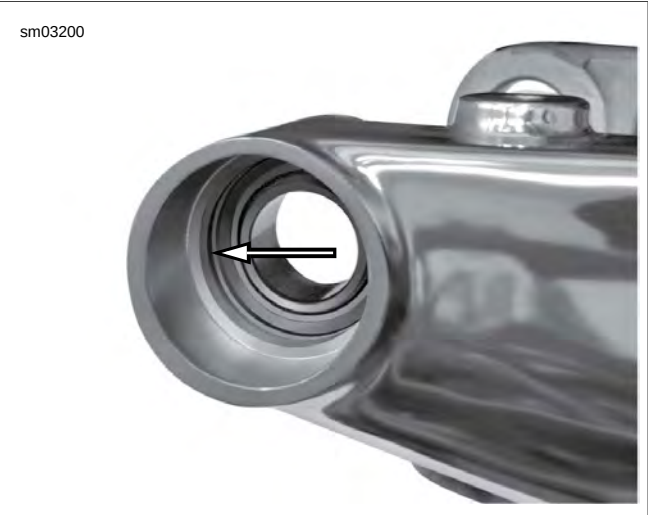
Figure 2-136. Lock Ring Fully Seated
