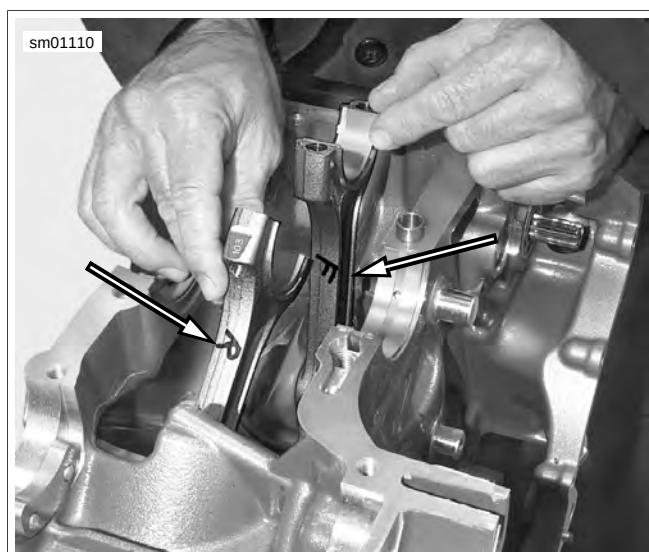
Figure 3-106. Mark Connecting Rods
