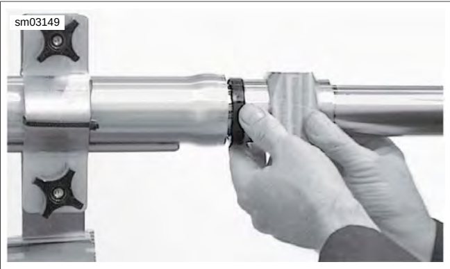
Figure 2-103. Install Bushing, Spacer, and Install Fork Seal in Place with Seal Driver
