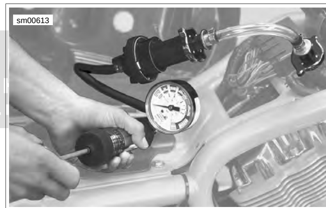
Figure 5-4. System Pressure Test (typical)
