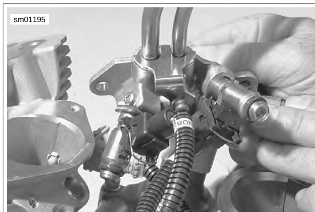
Figure 4-8. Fuel Rail with Injectors
