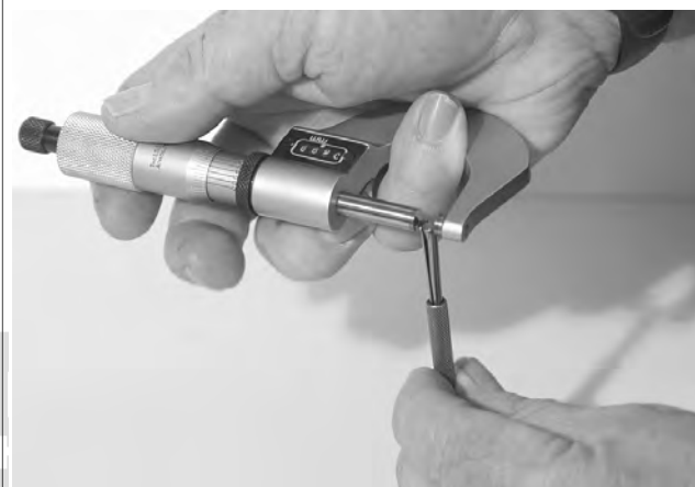
Figure 3-68. Measure Stem to Guide Clearance
