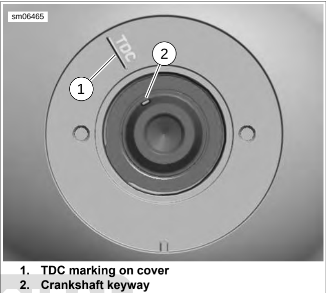
Figure 3-11. TDC Timing Alignment (alternator bolt removed)
