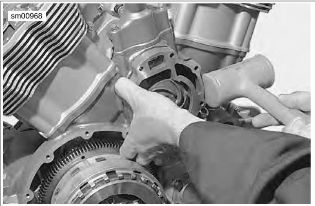
Figure 3-25. Removing Water Pump Housing
