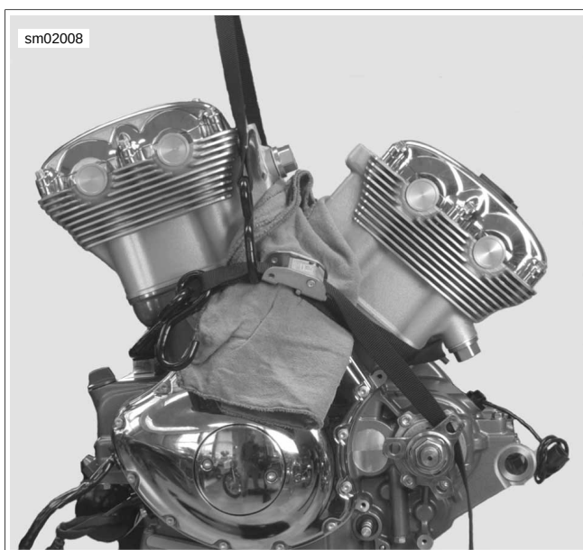
Figure 2-15. Engine Strapped for Hoisting
