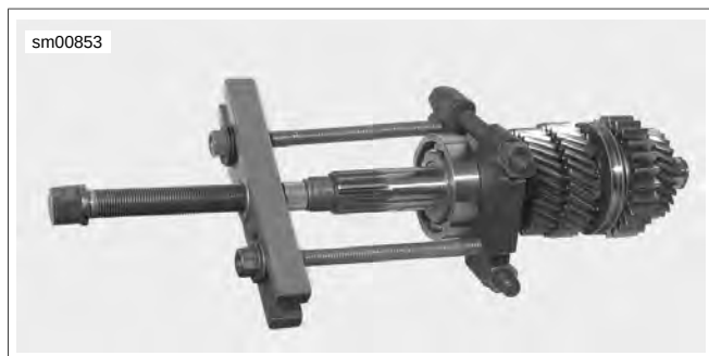
Figure 6-152. 1st Gear Bearing Removal
