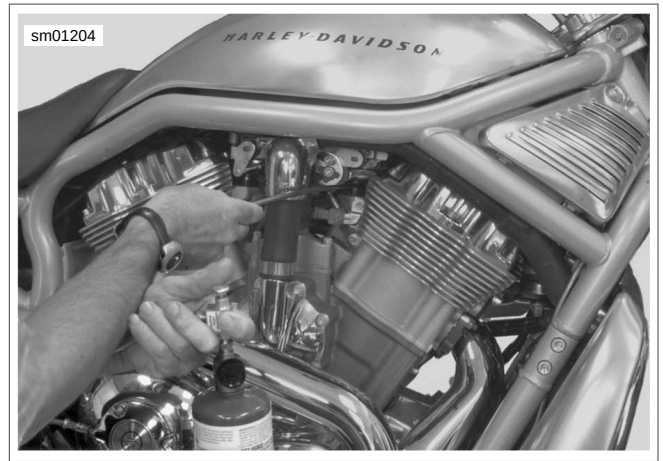
Figure 4-35. Checking for Leaks (typical)
