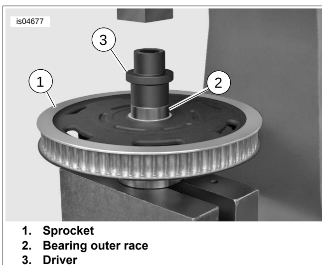
Figure 2-64. Install Compensator Sprocket Bearing
