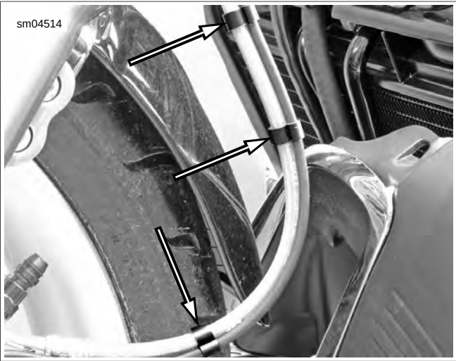
Figure 2-56. ABS Sensor Cable to Brake Hose Clips
