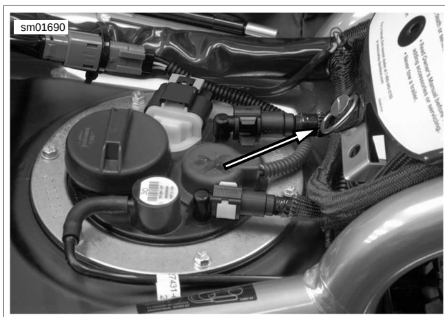
Figure 1-8. Air Box Cover Bailhead Fastener (typical)
