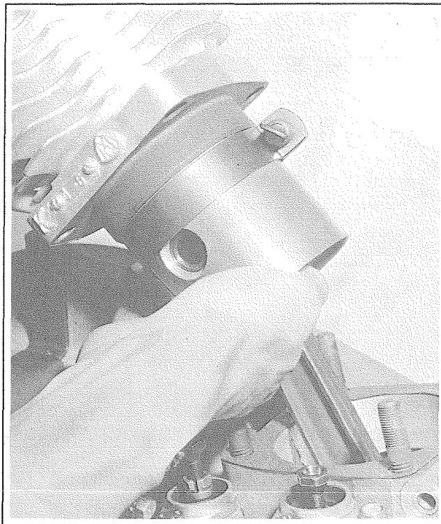
Figure 3C-29. Installing Cylinder on Piston
