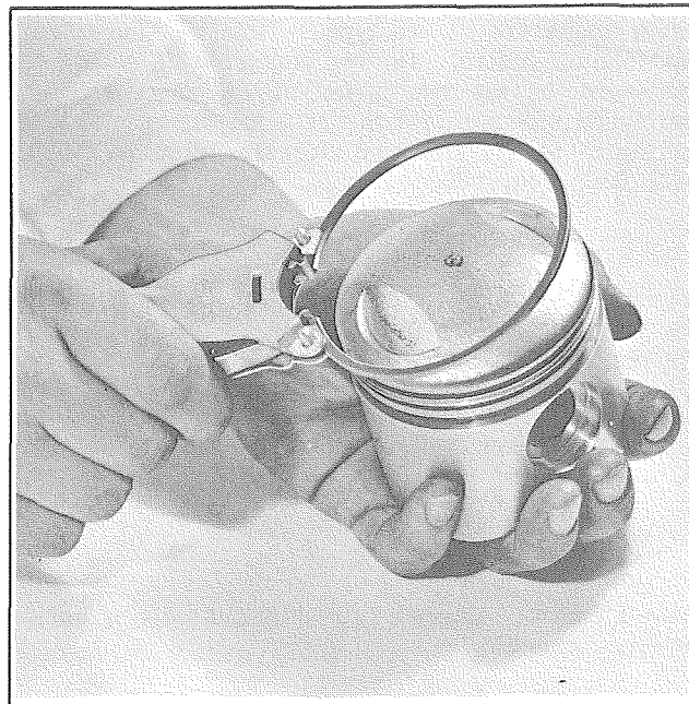
Figure 3C-23. Installing Piston Rings
