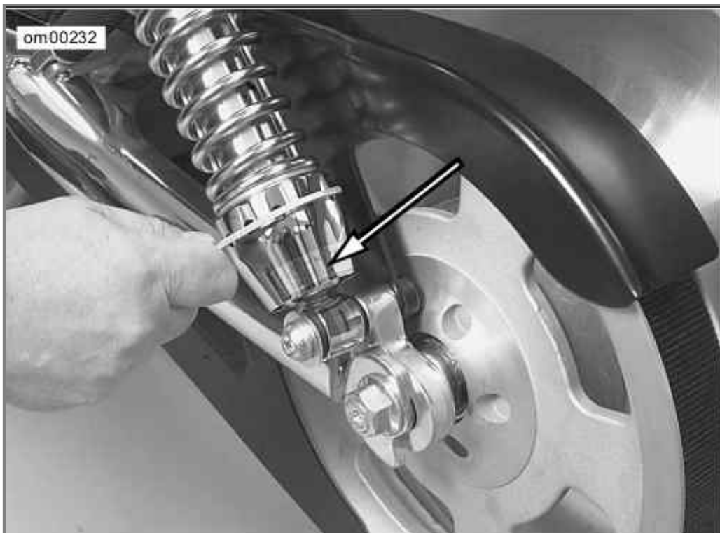
Rear Shock Absorber Adjustment: VRSCAW/VRSCDX Models
