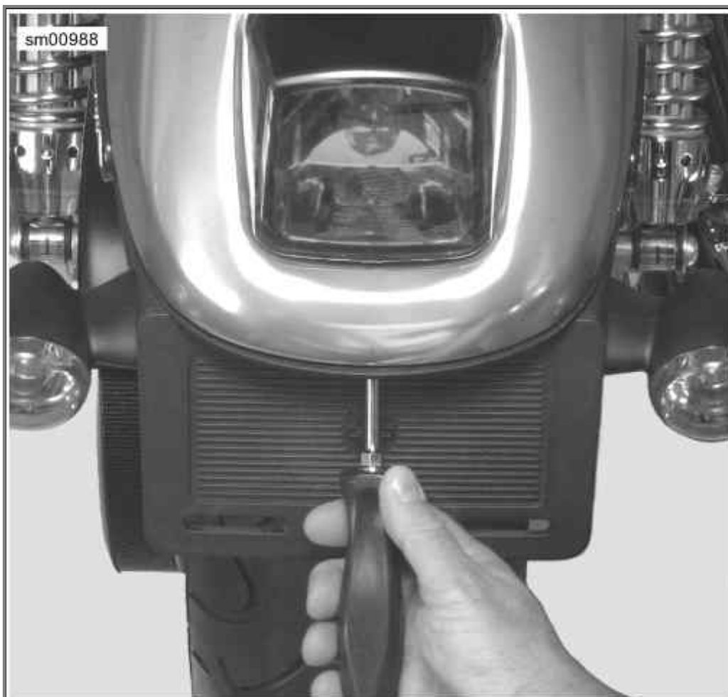
Releasing Tail Lamp Retaining Clip: VRSCAW/VRSCDX
