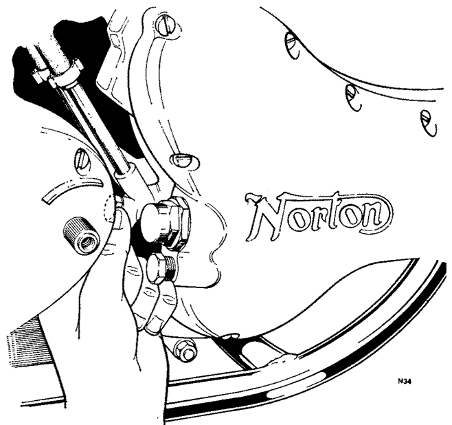
Fig. F1 Removing oil junction block securing bolt
