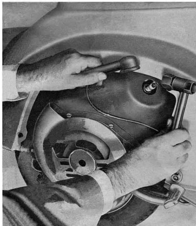
Fig. 10 - Dismantling spark - plug
