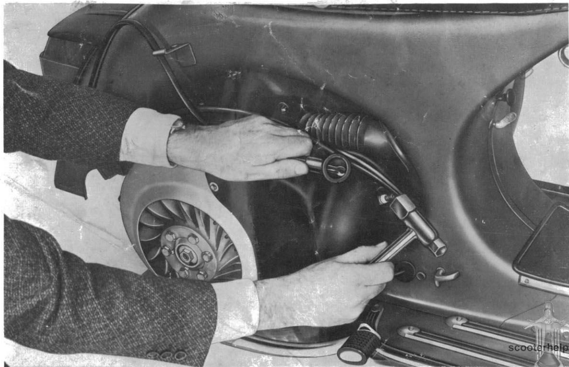
Fig. 15 - Dismantling spark plug
