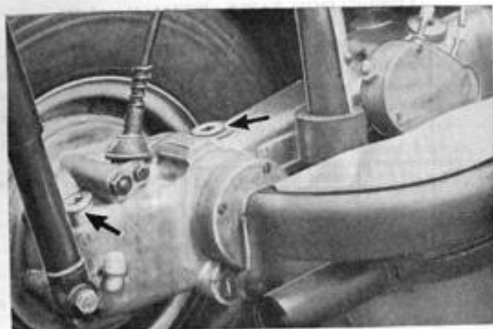
FIG. 21. FORWARD PLUG LUBRICATES REAR WHEEL SWINGING ARM. REAR PLUG REAR WHEEL TRANSMISSION
