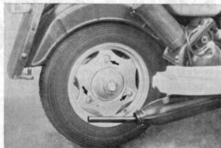
FIG. 27. REMOVAL OF PRIMA V REAR WHEEL REQUIRES THREE NUTS ONLY TO BE UNSCREWED
