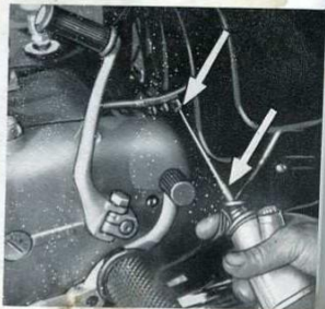
Greasing the rear chain
