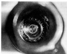
3.3 Remove damper rod retaining nut and withdraw stanchion from lower leg
