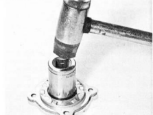
28.4 Oil seals can be drifted into position using a tubular drift
