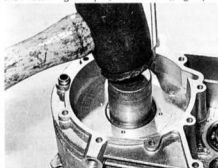
28.2 Tap bearings into place using a suitable tubular drift
