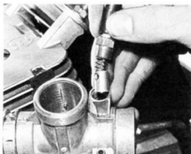
5.2 Unscrew throttle valve and choke plunger and remove carburettor
