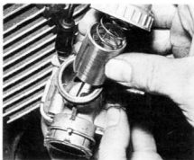
5.4 On refitting ensure slot in throttle valve aligns with pin in carburettor body
