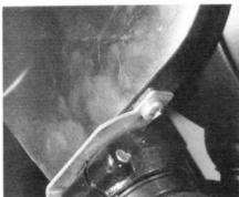
11.1a On basic models, fairing is retained by a single screw on each lower edge ...
