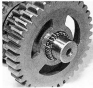
26.13g Insert all the needle rollers into the centre of the pinion ...
