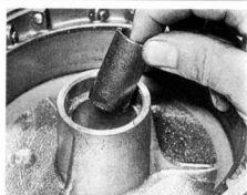
6.6c ... then invert wheel, insert spacer and fit second bearing in a similar manner
