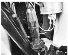
On 251 models rear stoplamp switch is adjusted using plastic sleeve not ...
