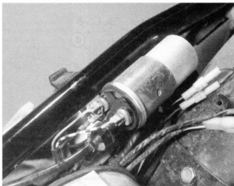
8.9 Ignition HT coil is located under the seat
