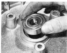
6.6a Wheel bearings should be fitted with their sealed surface facing outwards
