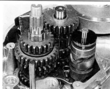
29.6c Install the selector drum and fit selector fork guide pin to its respective groove
