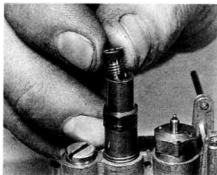
6.4a Main jet is a screw fit into base of needle jet ...
