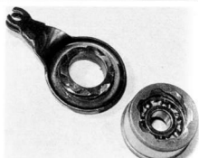
22.7 Examine clutch lifting mechanism worm gear for wear – 251 shown
