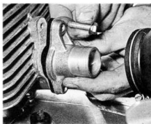
5.6 Inlet stub can be removed if necessary - check gasket
