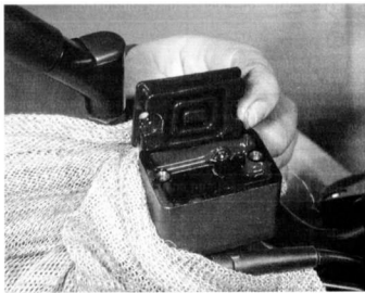
2.2b Remove reservoir cap, plate and diaphragm to add fluid
