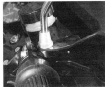
11.10a Hand guards are retained by the mirror mounting ...
