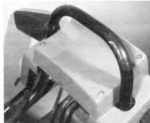
11.7 Tail fairing bridging panel is retained by four screws
