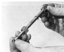
31.1a On 125 and 150 models, fit the circlips and thrust washers to each end of the tachometer driven gear ...
