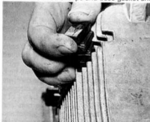
6.2 Do not forget to remove noise dampers before removing cylinder head
