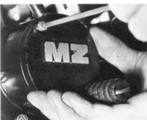
12.1 Oil pump is located behind small circular cover on left-hand crankcase cover - 125 shown
