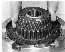
33.8c Fit the primary drive gear to align all friction plate slots ...
