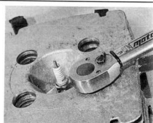
36.5b ... then refit cylinder head and tighten nuts to specified torque setting
