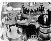
29.6f Refit the gearchange shaft ensuring its return spring and claw are correctly engaged
