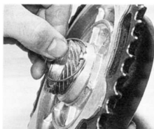
7.7a Ensure speedometer drive gear circlip fits into hole in sprocket
