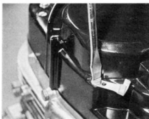
34.3a On 125 and 150 models do not omit oil pipe guide (where fitted)
