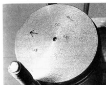
36.3b ... ensuring arrow on piston crown faces forward ...
