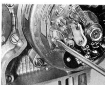
Slacken retaining screws and move contact breaker baseplate to adjust ignition timing
