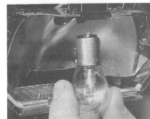
13.6a 251 models employ a combined stop/tail lamp bulb. Note offset pins on bulb...
