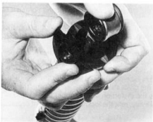
13.2a Compress spring, remove split collets from top of suspension unit ...
