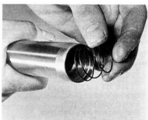
3.8d Refit the spring ensuring its large end is uppermost ...
