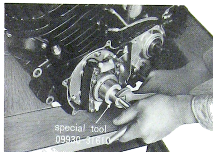
Fig. 5-1-2 Removing magneto rotor
