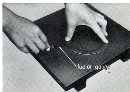
Fig. 5-2-23 Checking clutch driven plate warpage
