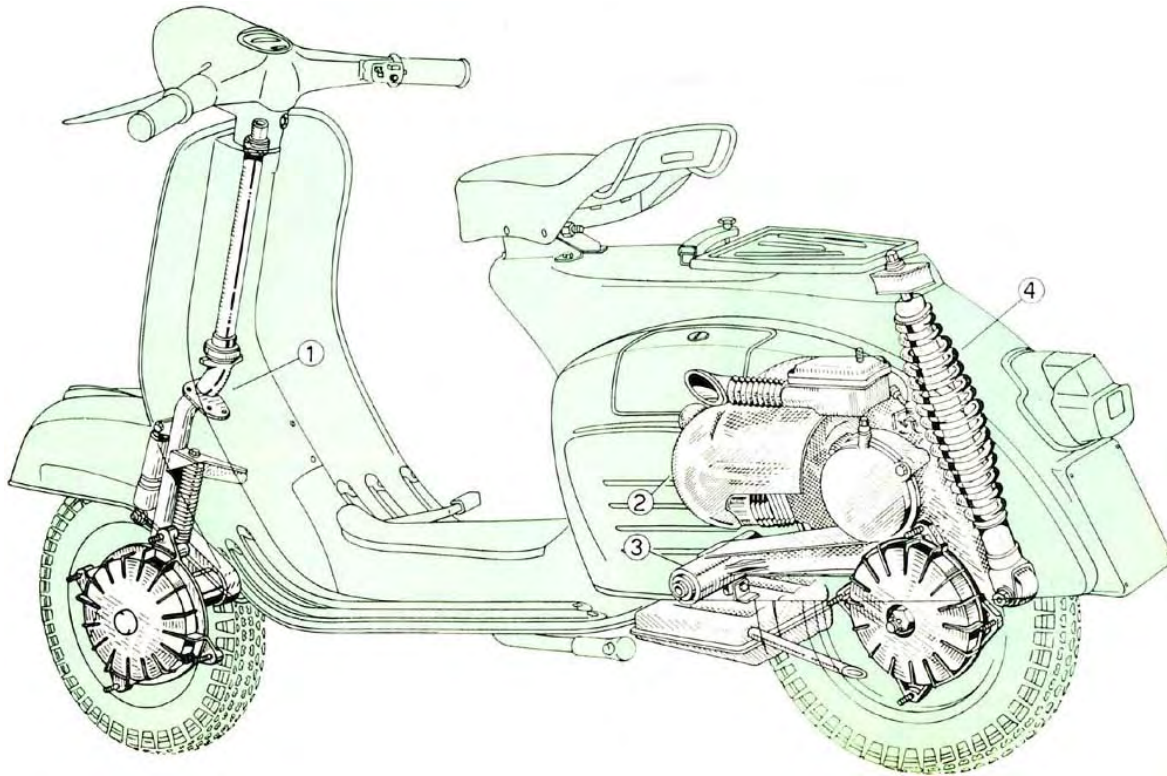
Fig. 20 - Installation of engine and suspension
