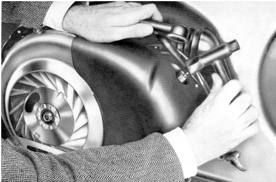
Fig. 10. Dismantling spark plug
