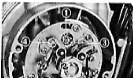
(1) Index mark (2) "F" mark (3) Cylinder number (4) 1.4 cylinder breaker points (5) Contact breaker base plate
