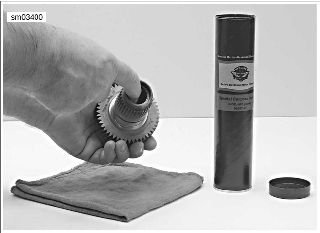
Figure 5-77. Lubricating Main Drive Gear Needle Bearing
