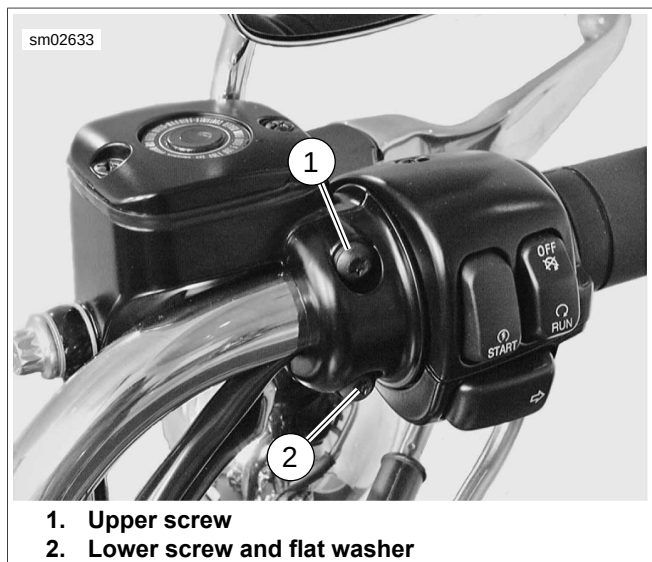
Figure 6-147. Handlebar Switch Clamp Screws
