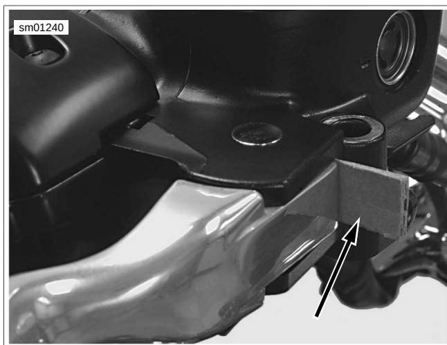
Figure 2-52. Install Cardboard Insert Before Removing Master Cylinder Assembly
