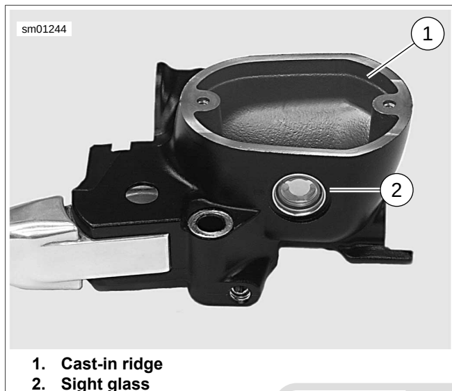
Figure 2-60. Filling Front Master Cylinder Reservoir
