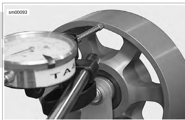
Figure 1-29. Measuring Lateral Side Play on Idler Pulley
