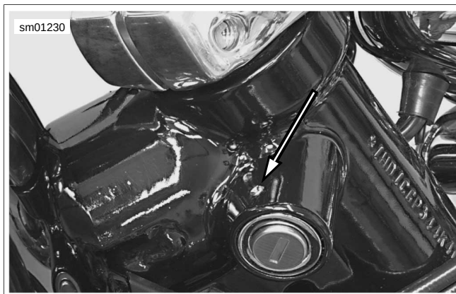
Figure 2-240. Fork Lock Pin
