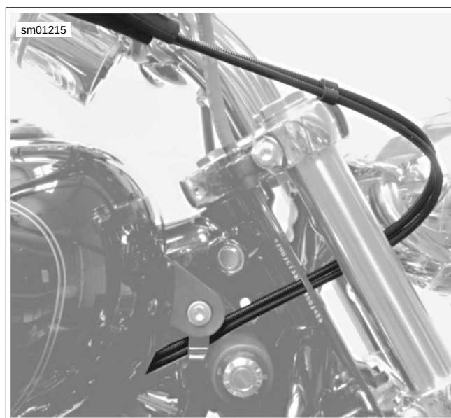
Figure 2-177. Throttle Control Cable Routing: XL Models
