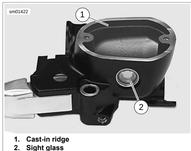
Figure 1-58. Filling Front Master Cylinder Reservoir (typical)
