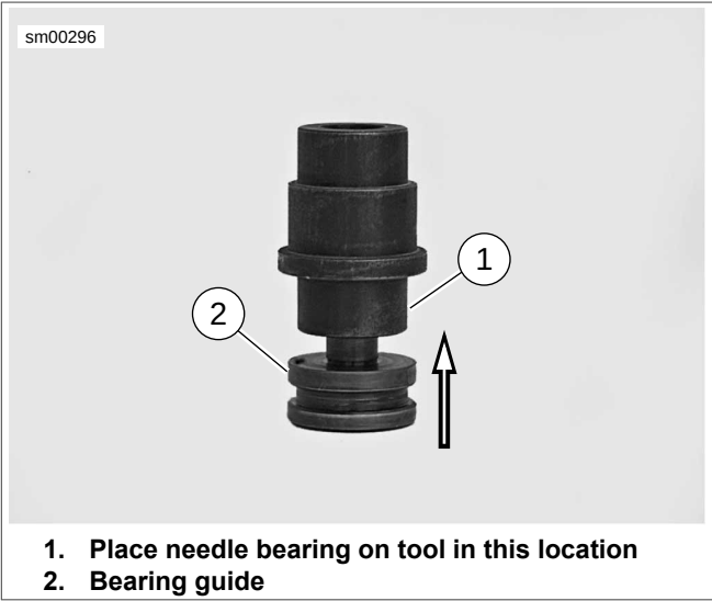
Figure 5-28. Bearing Installer
