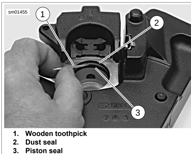
Figure 2-105. Caliper Seals
