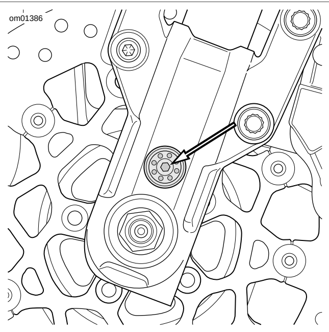
Figure 1-79. Spring Preload Adjuster: XR 1200X
