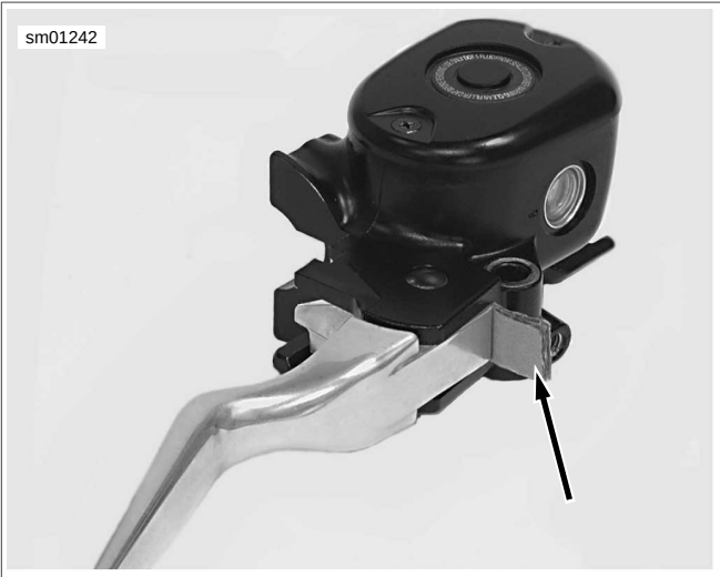
Figure 2-56. Install 5/32 in (4 mm) Cardboard Insert Before Installing Master Cylinder Assembly
