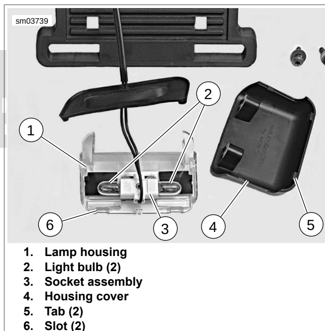
Figure 6-62. Replacing License Plate Light Bulbs: XL 883N, XL 1200X (HDI)
