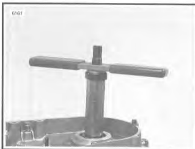
Figure 3-99. Installing Flywheel Spacer and Outer Bearing
