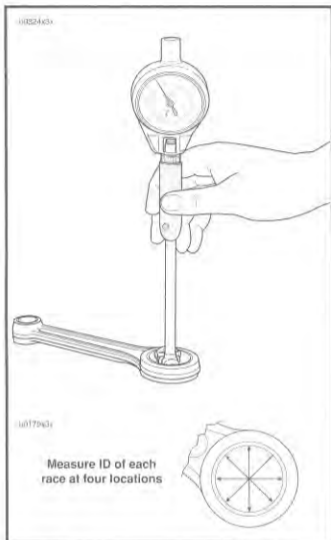
Figure 3-82. Measuring Connecting Rod Race Inside Diameter
