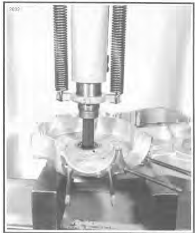
Figure 3-77. Sprocket Shaft Outer Race Removal
