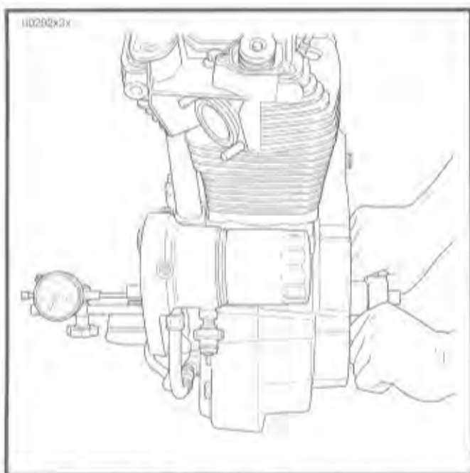
Figure 3-73. Checking Flywheel End Play
