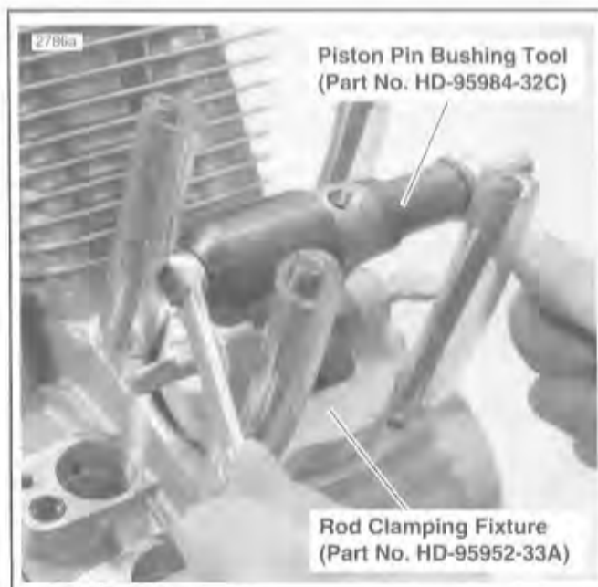
Figure 3-36. Installing New Piston Pin Bushing
