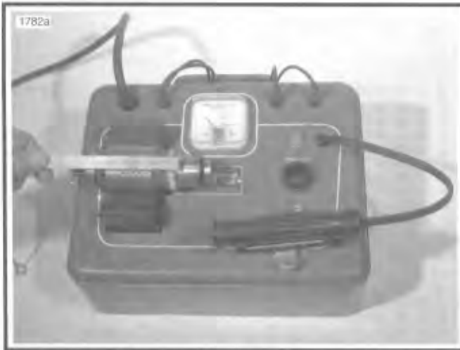
Figure 5-14. Shorted Armature Test Using Growler
