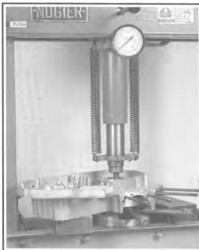
Figure 3-75. Pressing Flywheel from Crankcase
