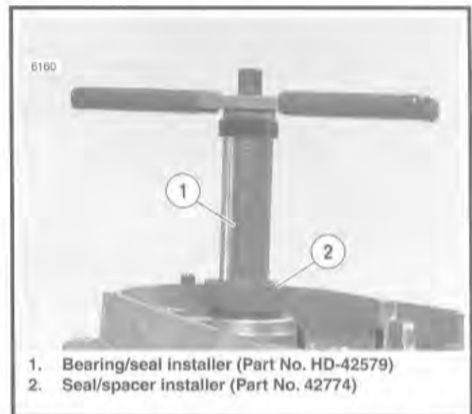
Figure 3-101. Install Bearing Seal/Spacer
