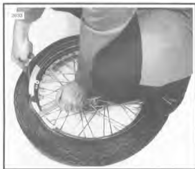
Figure 2-33. Starting Tire Off Rim
