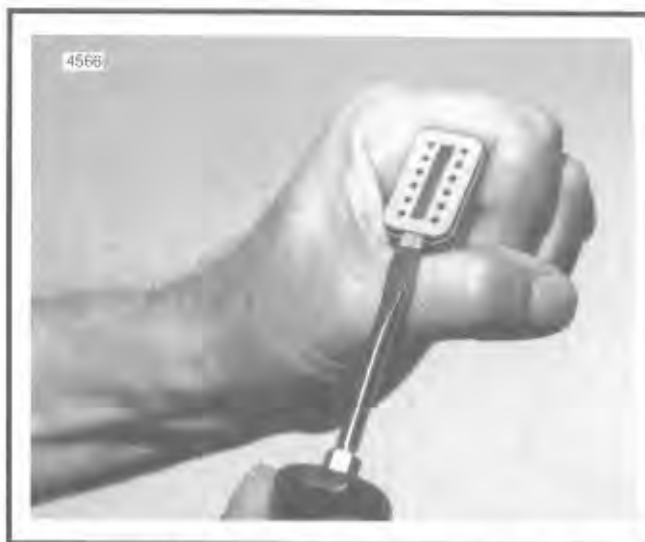
Figure 7-98. Remove Secondary Locking Wedge
