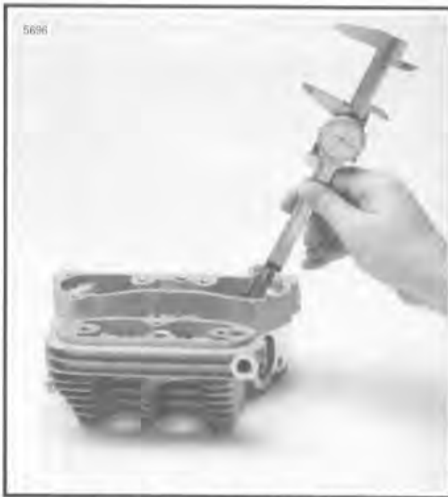
Figure 3-21. Measuring Valve Stem Protrusion
