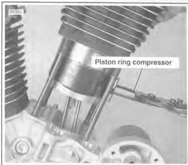
Figure 3-38. Installing Cylinder Over Piston
