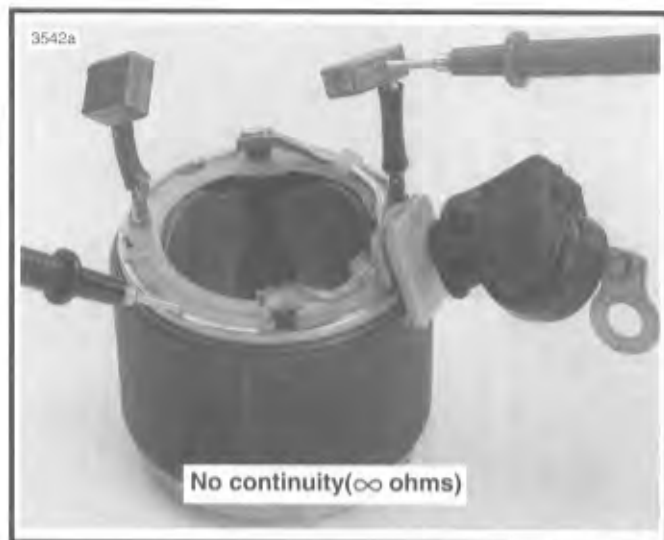
Figure 5-17. Grounded Field Test
