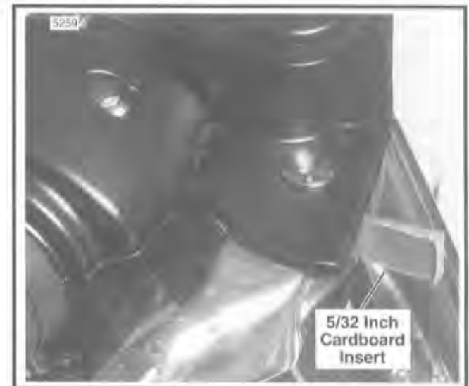
Figure 2-43. Install Cardboard Insert Before Removing Master Cylinder Assembly
