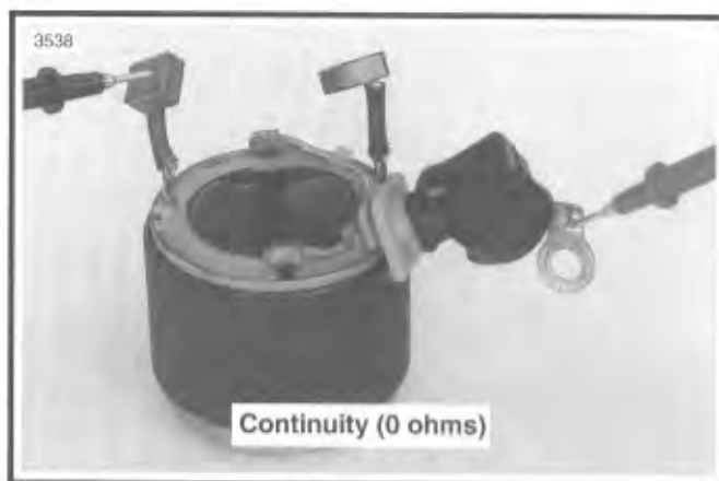
Figure 5-18. Open Field Test
