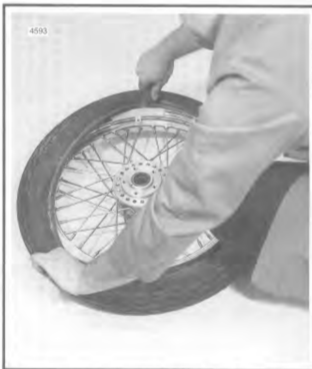
Figure 2-36. Starting Second Bead on Rim
