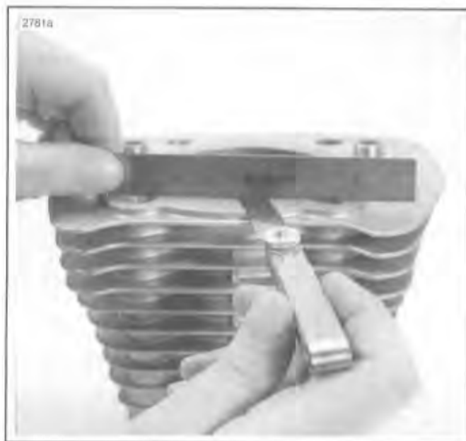
Figure 3-28. Checking Gasket Surfaces
