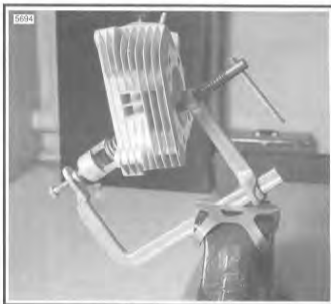
Figure 3-10. Compressing Valve Springs
