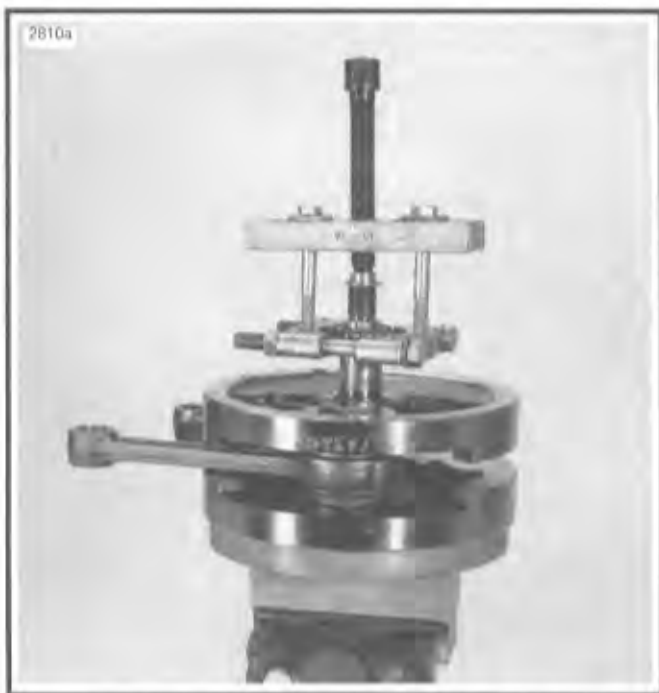
Figure 3-78. Removing Sprocket Shaft Roller Bearing
