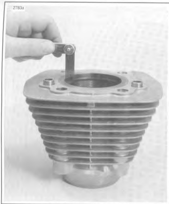
Figure 3-31. Measuring Ring End Gap
