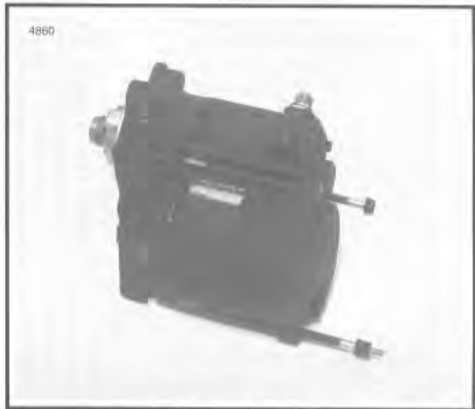
Figure 5-9. Removing the Thru-Bolts
