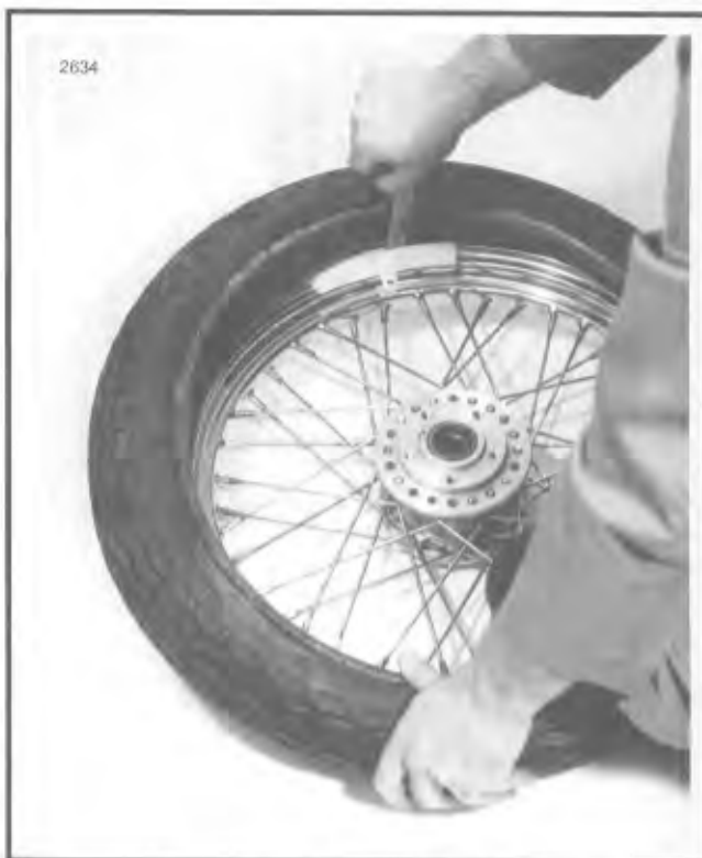
Figure 2-35. Starting Bead on Rim
