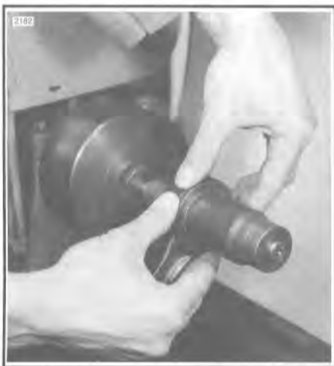
Figure 3-80. Lapping Connecting Rod Races
