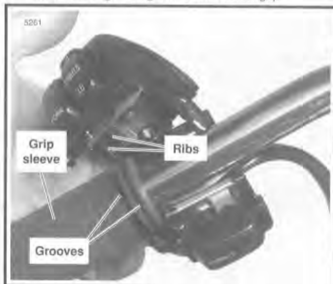
Figure 7-75. Install Left Handlebar Switch Housings
