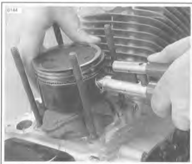
Figure 3-37. Installing Piston Retaining Rings
