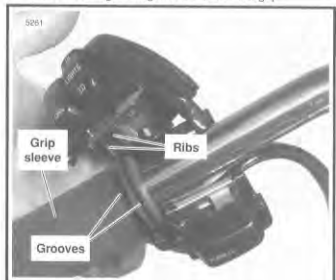
Figure 7-75. Install Left Handlebar Switch Housings
