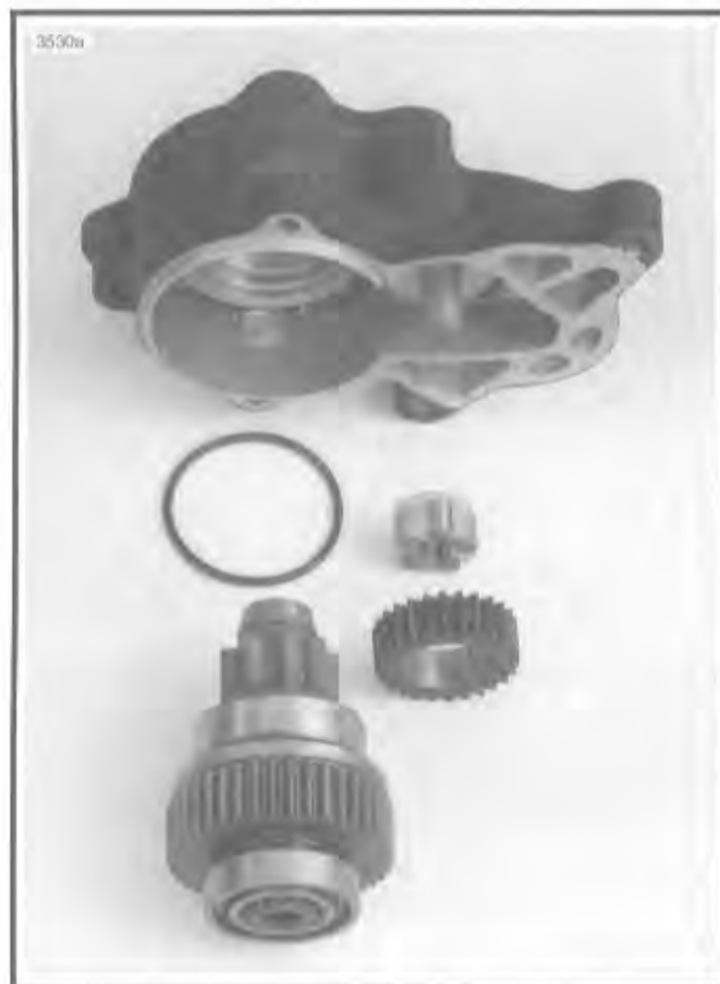
Figure 5-21. Starter Drive Assembly
