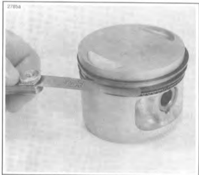
Figure 3-34. Measuring Ring Clearance in Groove
