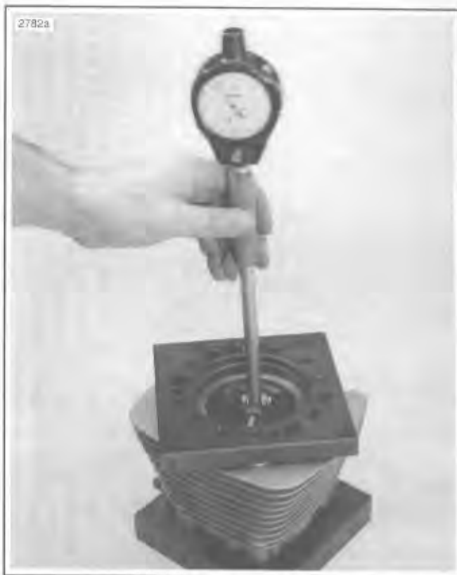
Figure 3-29. Measuring Cylinder Bore
