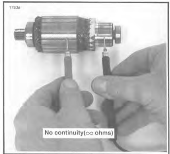
Figure 5-15. Grounded Armature Test
