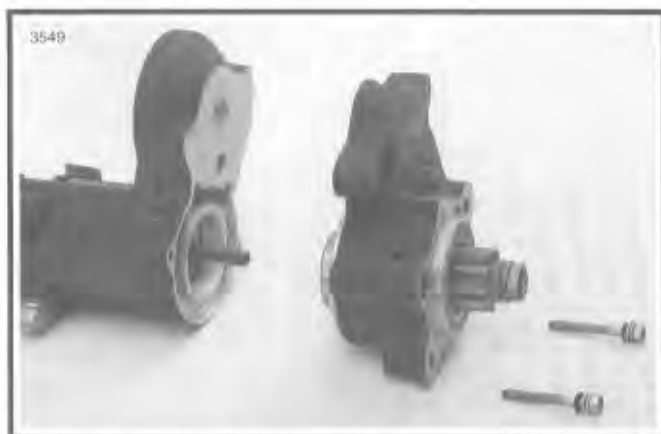
Figure 5-20. Removing Starter Drive Housing
