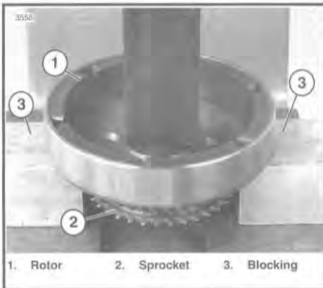
Figure 7-47. Removing Rotor From Sprocket
