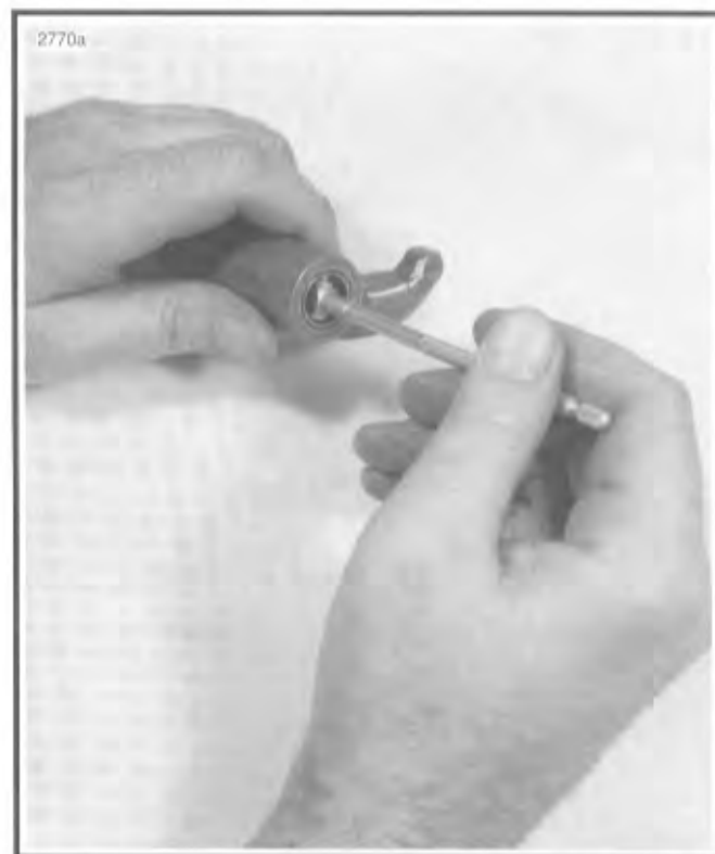
Figure 3-14. Measuring Rocker Arm Bushing Inner Diameter
