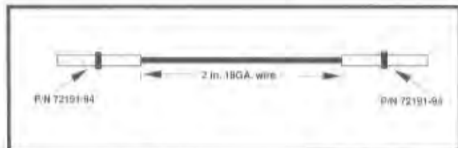
Figure 7-13. Diagnostic Test Wire
