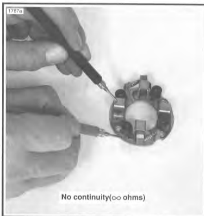
Figure 5-19. Brush Holder Insulation Test
