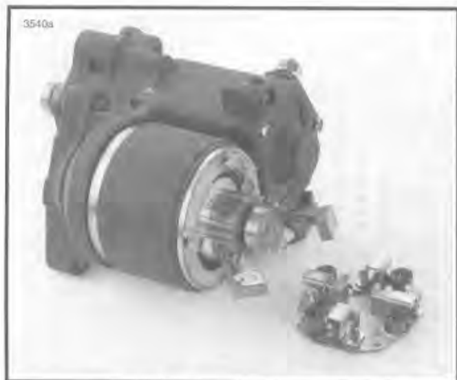
Figure 5-12. Removing Brush Holder
