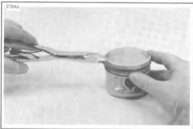
Figure 3-32. Installing Piston Rings
