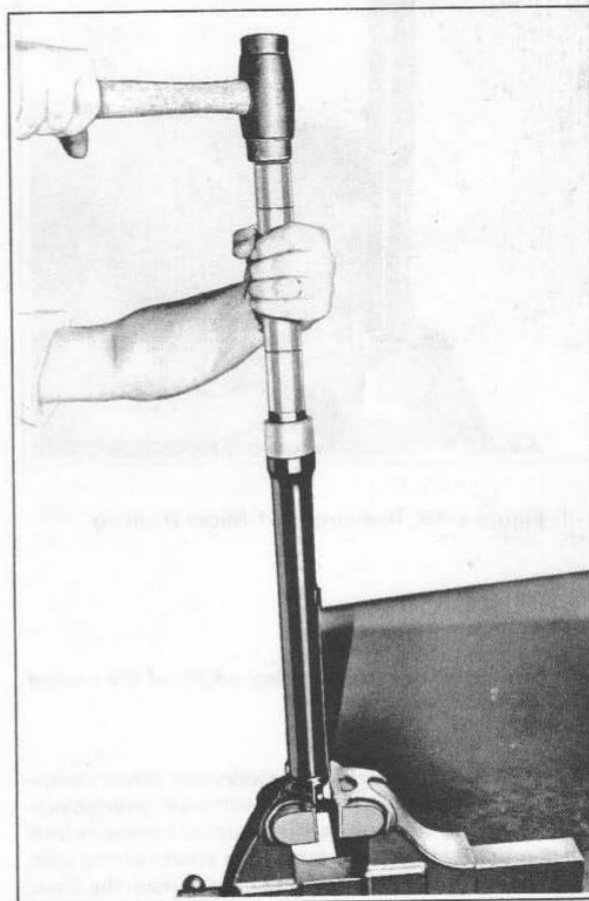
Figure 2-47. Installing Fork Slider Bushing
