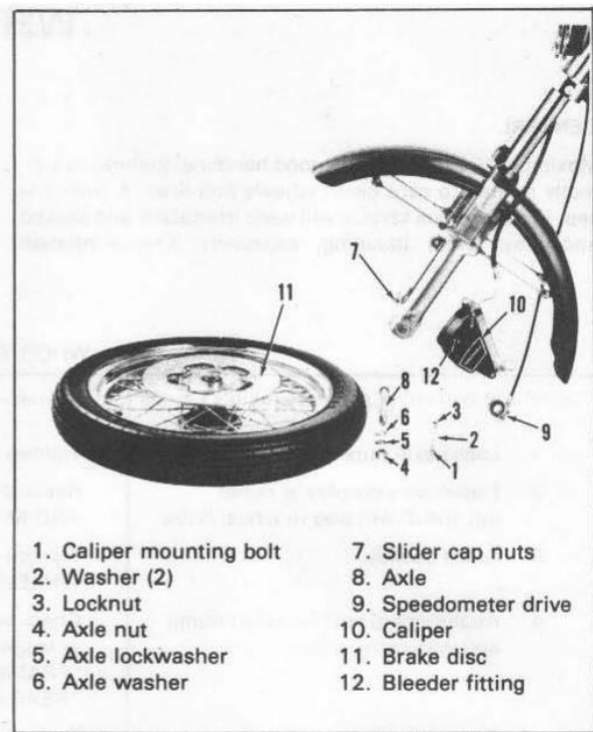
Figure 2-7. Front Wheel Removal (1974 to 1977)
