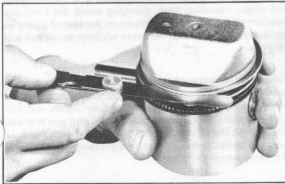
Figure 3-16. Measuring Ring Clearance in Grooves
