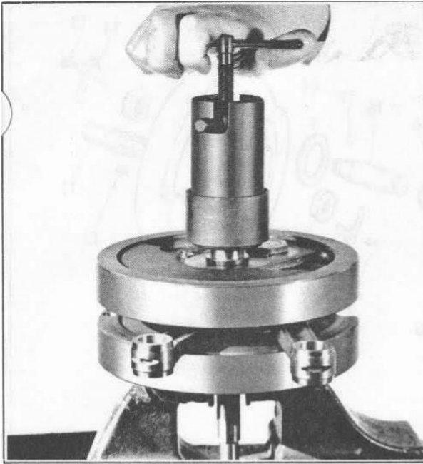
Figure 3-43. Removing Bearing from Sprocket Shaft
