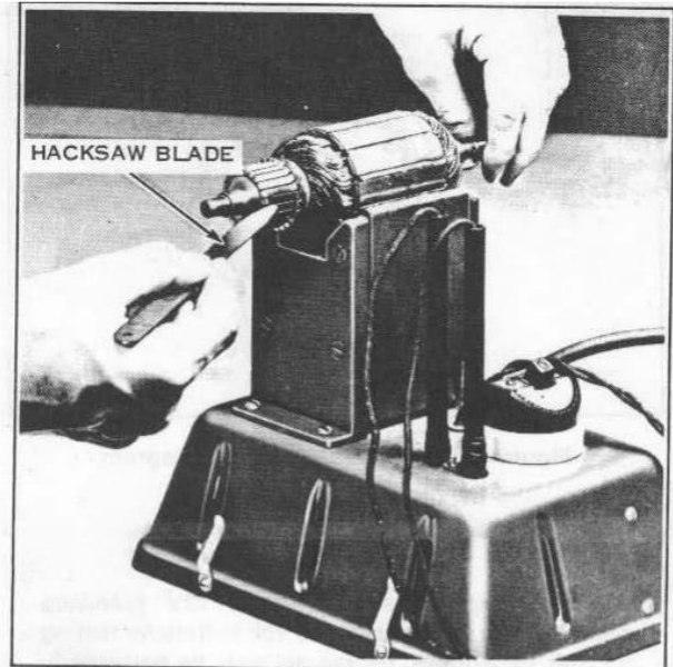
Figure 5-16. Testing Armature for Open Circuit
