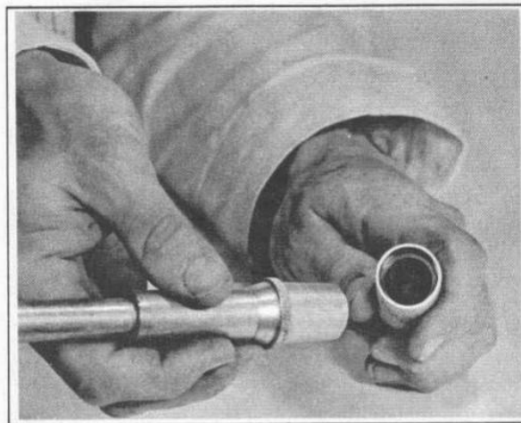
Figure 3-22. Inserting Piston Pin Lock Ring in Tool (1976 and Earlier)
