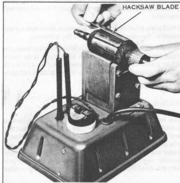
Figure 5-15. Testing Armature for Short
