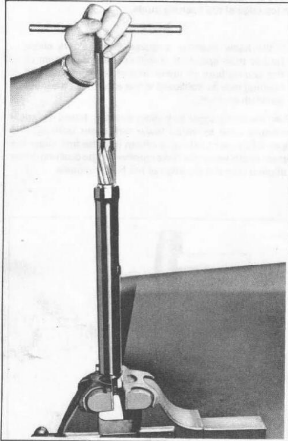
Figure 2-48. Reaming Fork Slider Bushing
