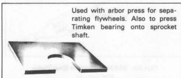
Part No. 96137-52A Flywheel Support Plate
