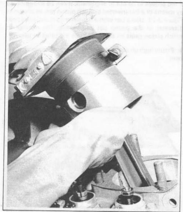
Figure 3-24. Installing Cylinder on Piston
