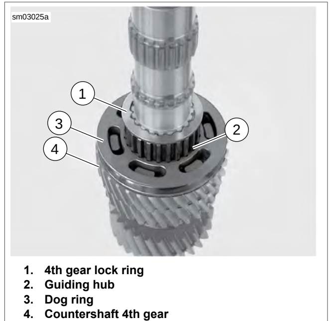
Figure 6-23. Countershaft Assembly
