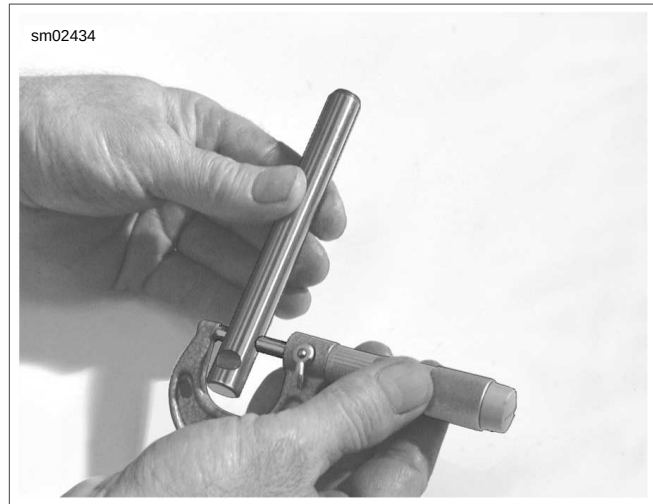
Figure 3-35. Checking Shaft to Bushing Fit
