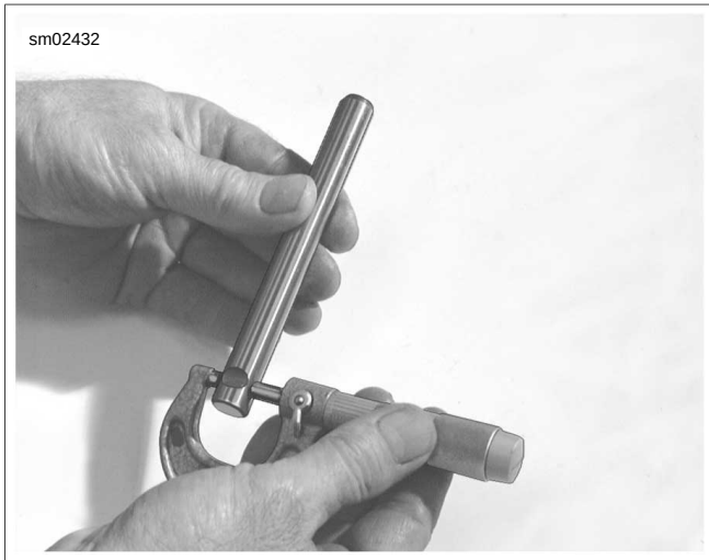
Figure 3-33. Checking Shaft to Support Plate Fit
