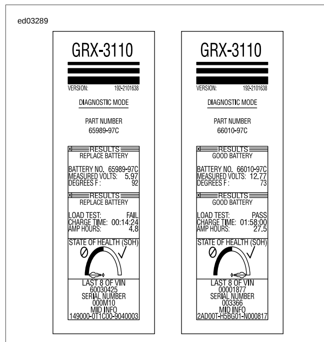
Figure 3-1. Battery Test Results Printout (Typical)
