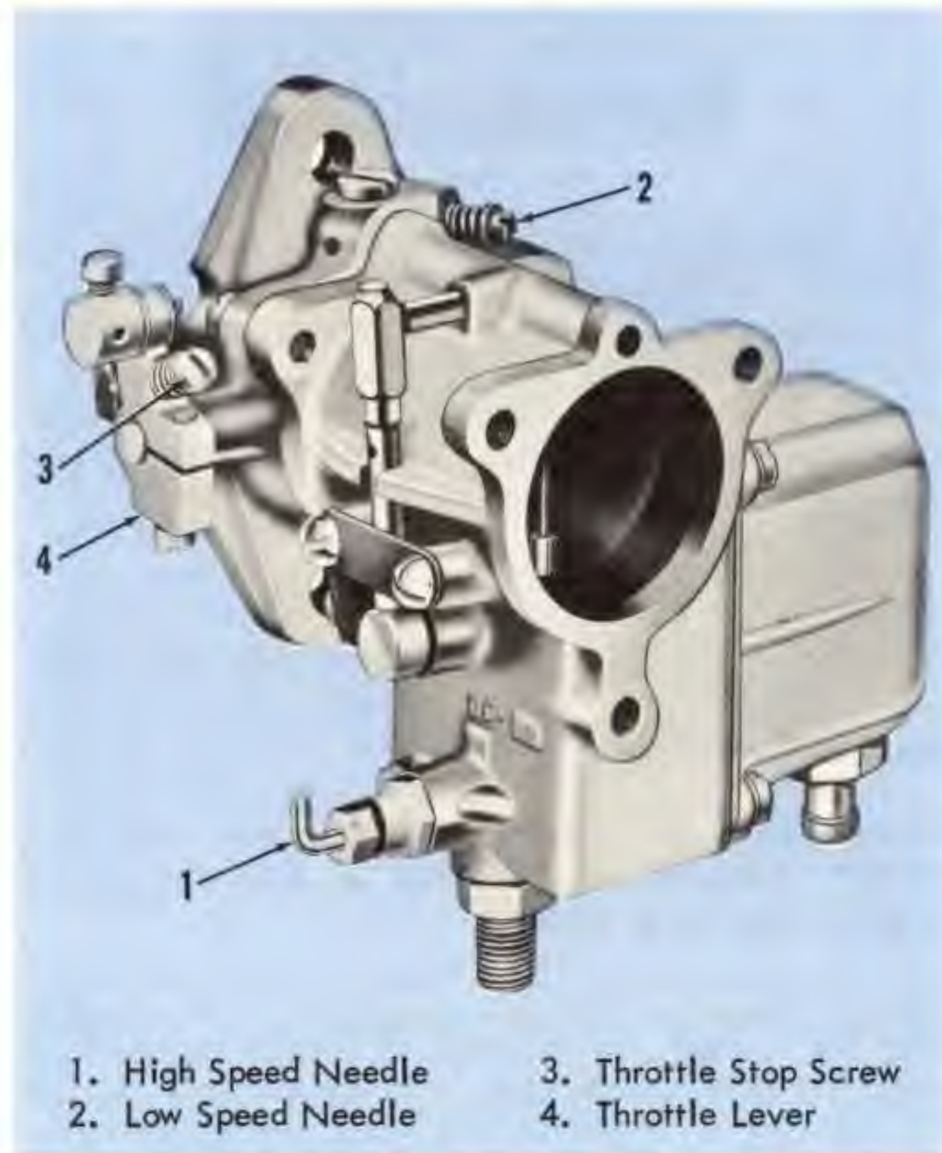
FIGURE 9. CARBURETOR
